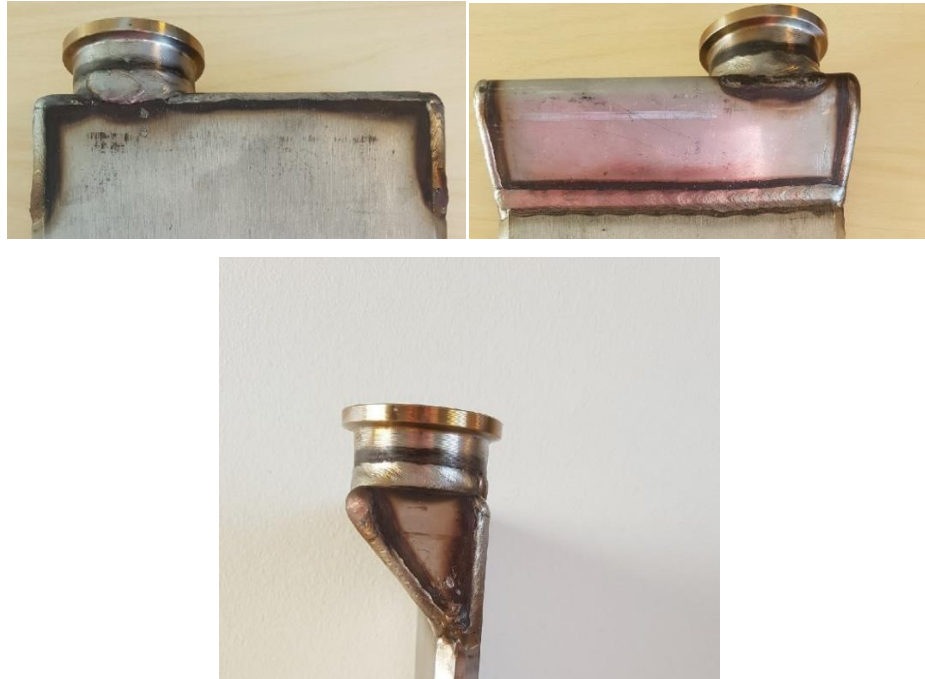
Figure 34. Welding sections in the pressing air nozzle.
