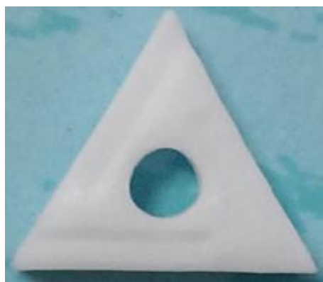
Figure 12. 3D printed alumina cutting tool cutting item without major defects (Mod. Zhou et al. 2016, p. 11602).
