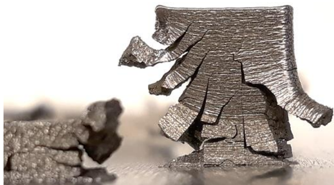
Figure 38. T15 test prints with brittle fractures and lack of fusion
