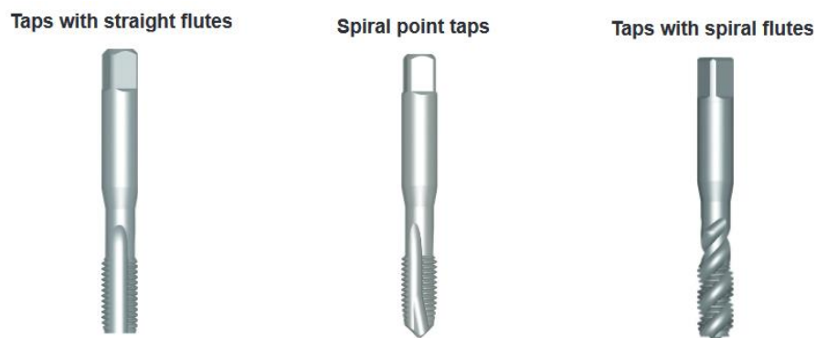
Figure 10. Different types of taps (Mod. DORMER 2013, p. 66-67).
