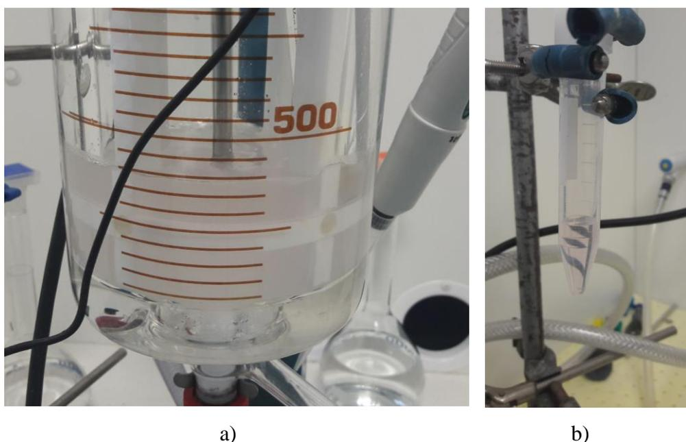
Figure 62. Stripping procedure: a) stripping process (mixing), b) pregnant aqueous phase
