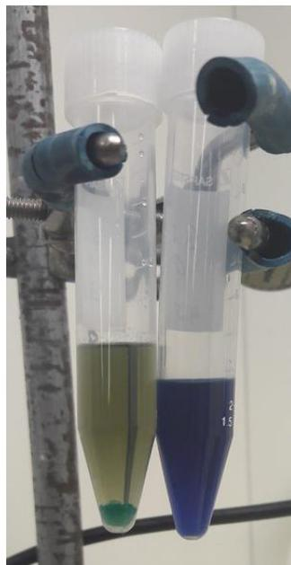
Figure 51. Samples of aqueous (left) and organic (right) phases after the extraction procedure
