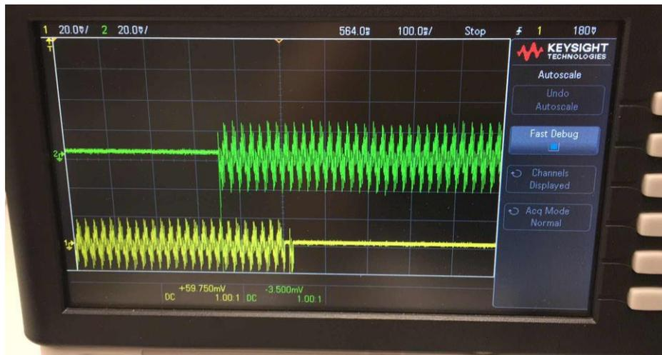
**Figure 36.** Hall signals detection without pull-up resistor
