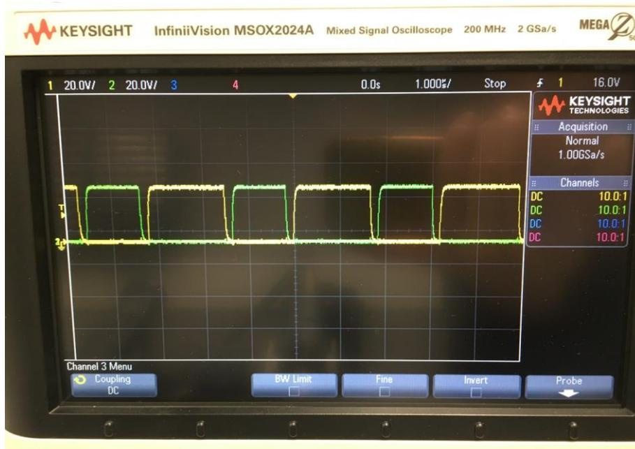
**Figure 40.** The PWM\_A and PWM\_B signals with a 200ns DTI.
