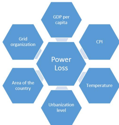
237 238 Fig. 11. Parameters which affect T&D grid power loss level.
