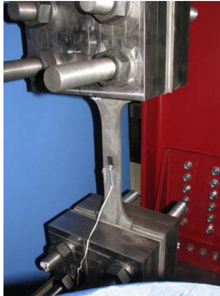
Figure 44. Test setup in 1200 kN test rig.
