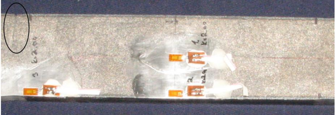
Figure 46. LC5-4 specimen with three strain gauges attached and crack on ground edge.
