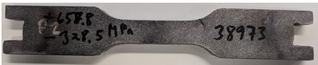
Figure 28. The specimen and crack nucleation point on curved section.
