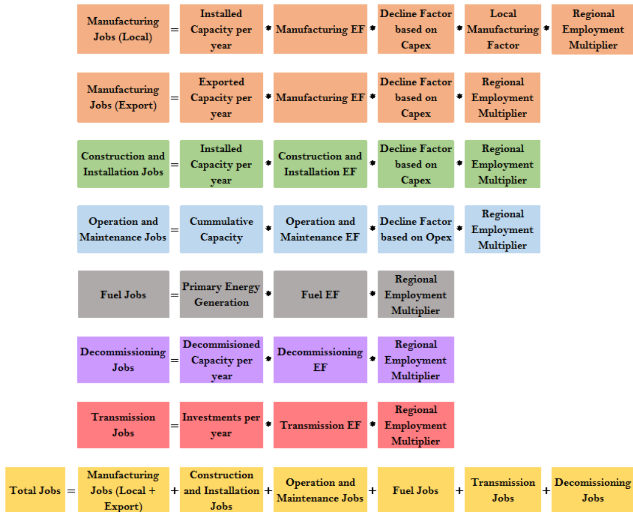
Figure 1: Method for estimation of job creation during the energy transition. Abbreviations: Employment Factor (EF), Capital Expenditure (CAPEX) and Operational Expenditure (OPEX).
