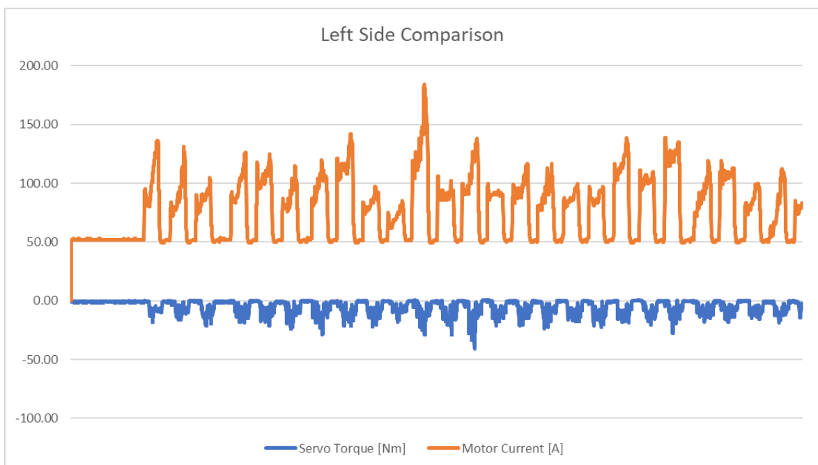
Figure 22. Comparison of the left side servo torque and motor current.
