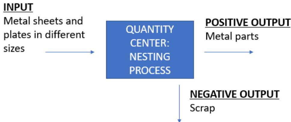
Figure 12. Material flow model of the nesting process.
