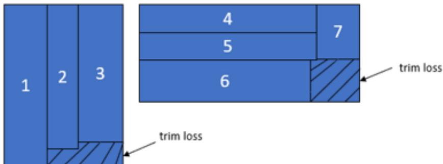
Figure 7. Illustration of the structure of cutting problems (Adapted from Dyckhoff 1990, 145)
