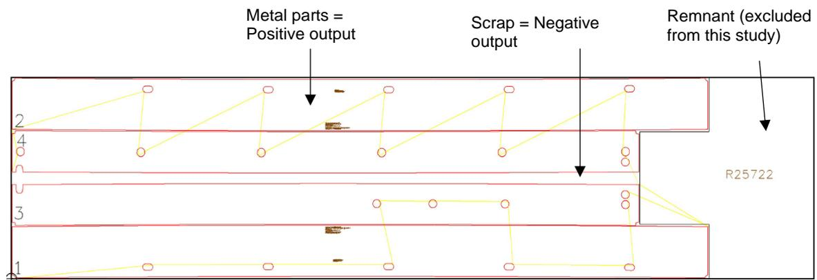
Figure 13. An example of the case company's nesting process (Source: case company's nesting report)
