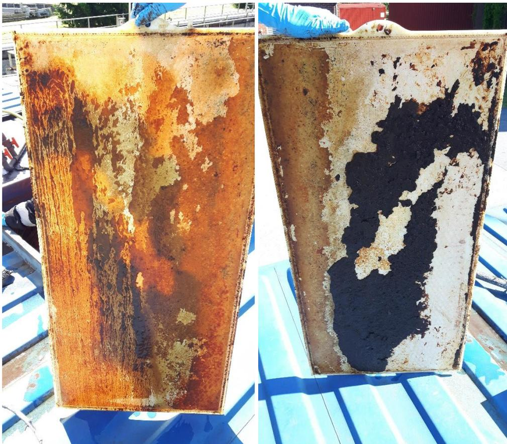
**Figure 49.** Gel layer and cake formation on the membrane surface.
