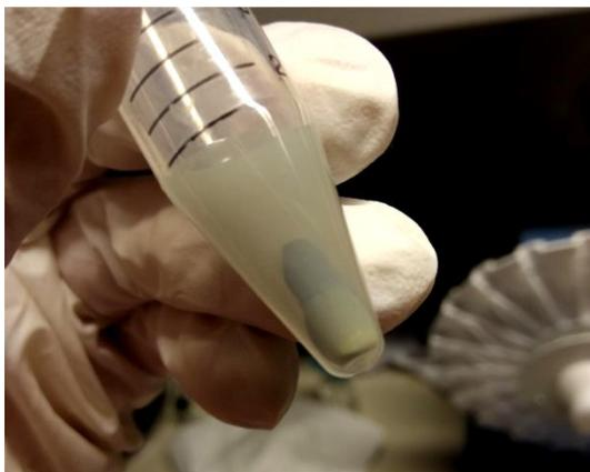
Figure 3.21. Centrifuged photocatalyst powder, nanoparticles and liquid phase after Au photoreduction
