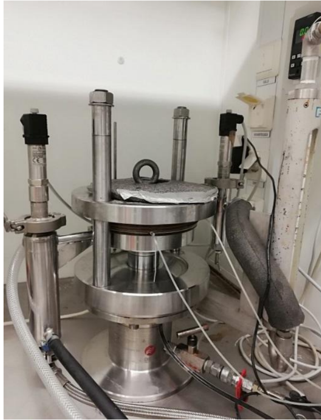
Figure 3.1. DSS Labstack M20 filter used in the nanofiltration and reverse osmosis filtration experiments.
