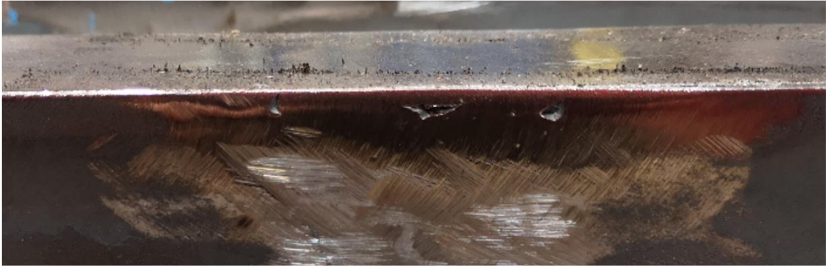
Figure 11 Rail after grinding
