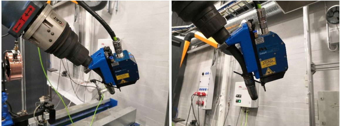
Figure 6. Laser sensor and bracket attachment connected to the welding torch.
