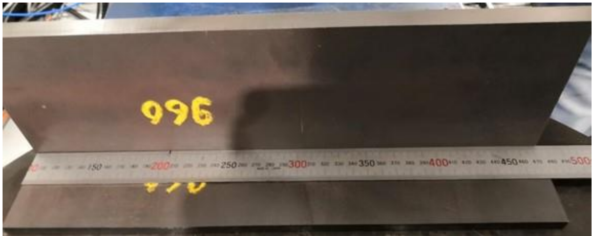
Figure 7. Measurement of the seam. Note that the ruler starts at 100\text{ mm} .
