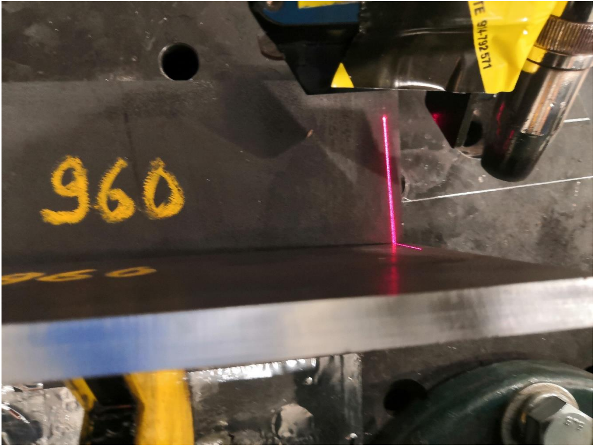
Figure 10. Laser sensor position relative to the workpiece.
