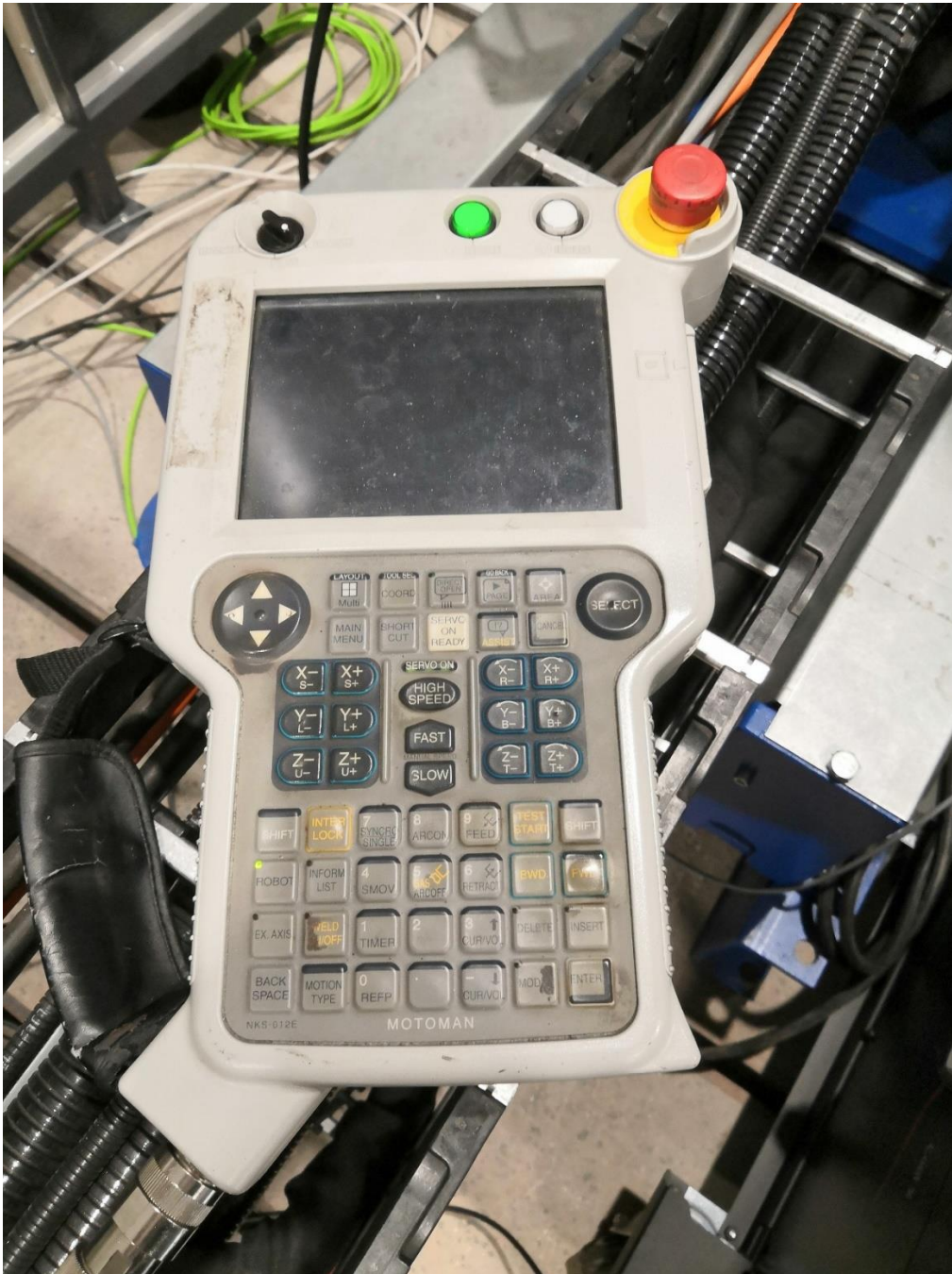
Figure 8. Robot controller used to set the starting position of the scan.
