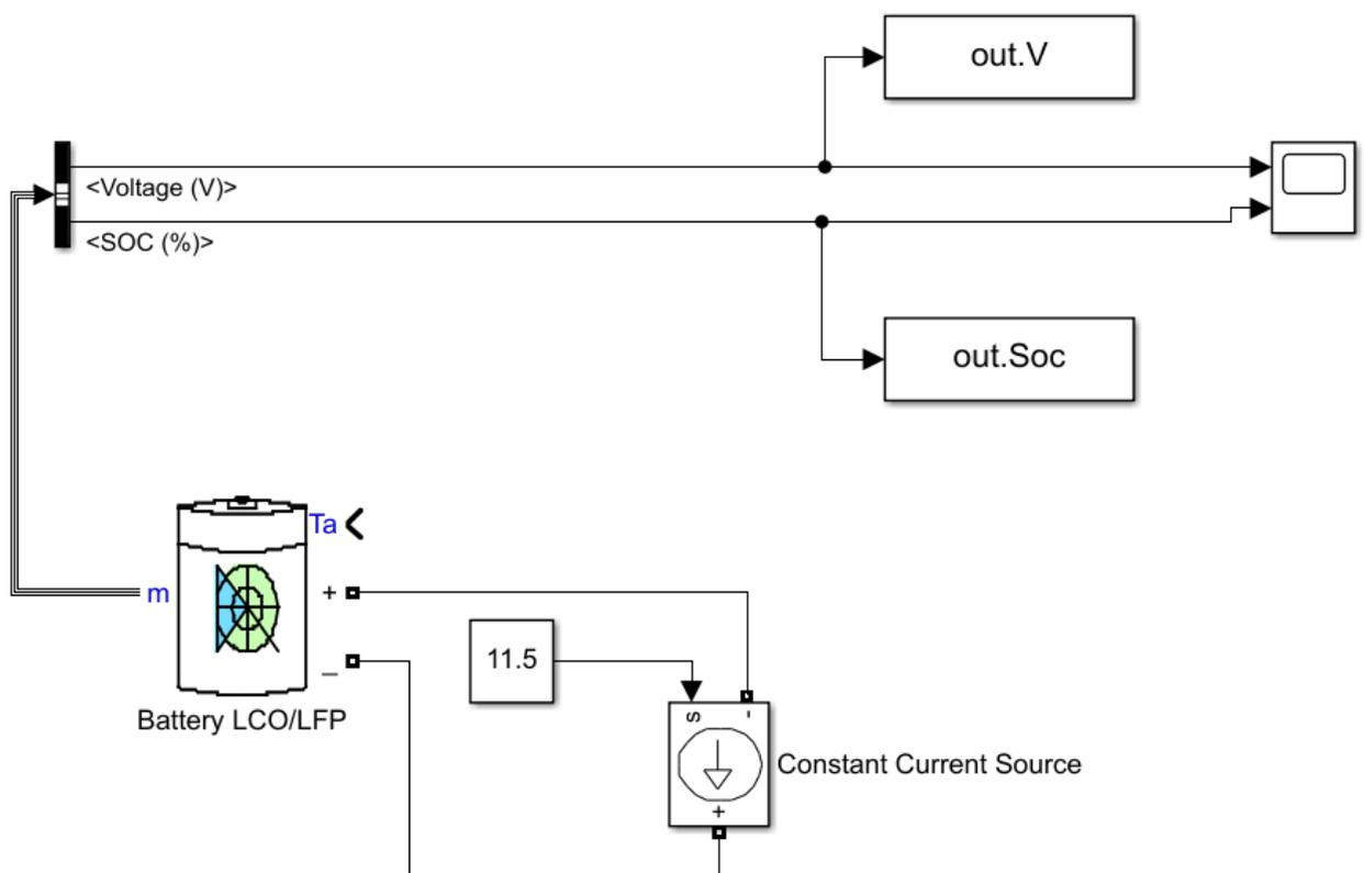
Fig. 3. Simulation of battery cell under constant discharge current.
