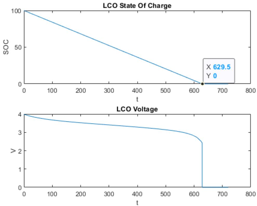
Fig. 4. LCO State of charge and voltage over time. The LCO cell is being discharged at 5C rating (10.25 A).
