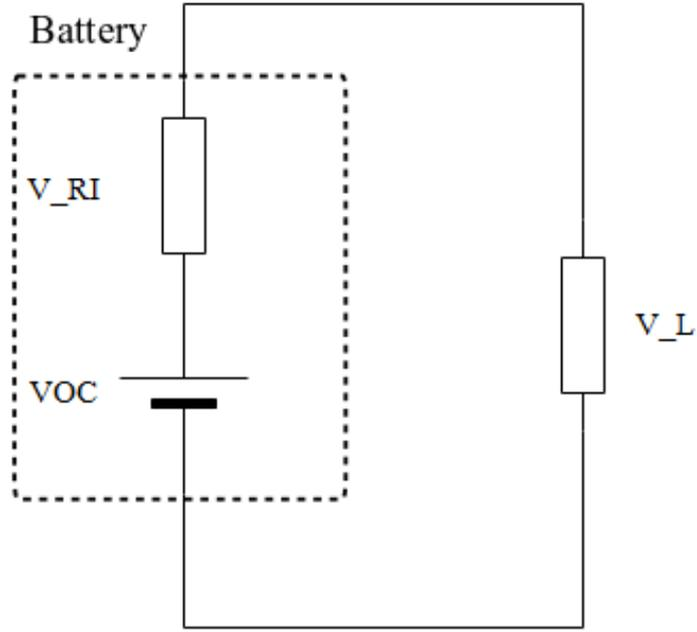
Fig. 1. Equivalent electric circuit of the battery with external load. Ideal voltage source VOC is complemented with resistance  $R_1$  to take into account the voltage drop inside the battery.
