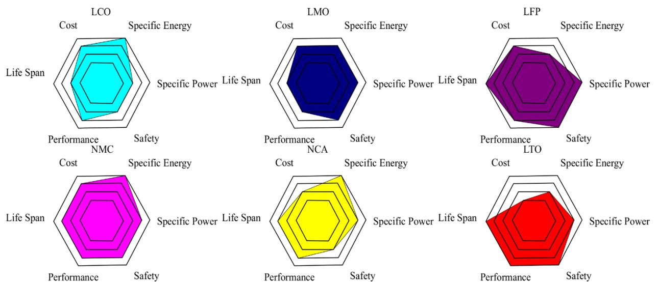
Fig. 2. Hexagons for each battery type showing characteristics under discussion [7].
