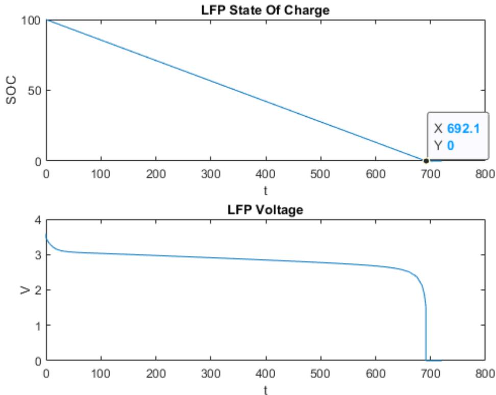
Fig. 5. LFP State of charge and voltage over time. The LCO cell is being discharged at 5C rating (11.5 A).
