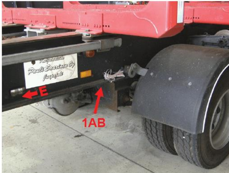
Figure 9. Strain gauges 1A and 1B.
