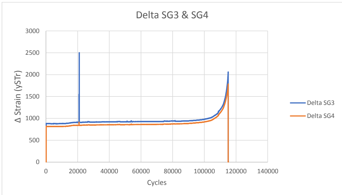
Figure 36. Delta strain values SG3 and SG4.
