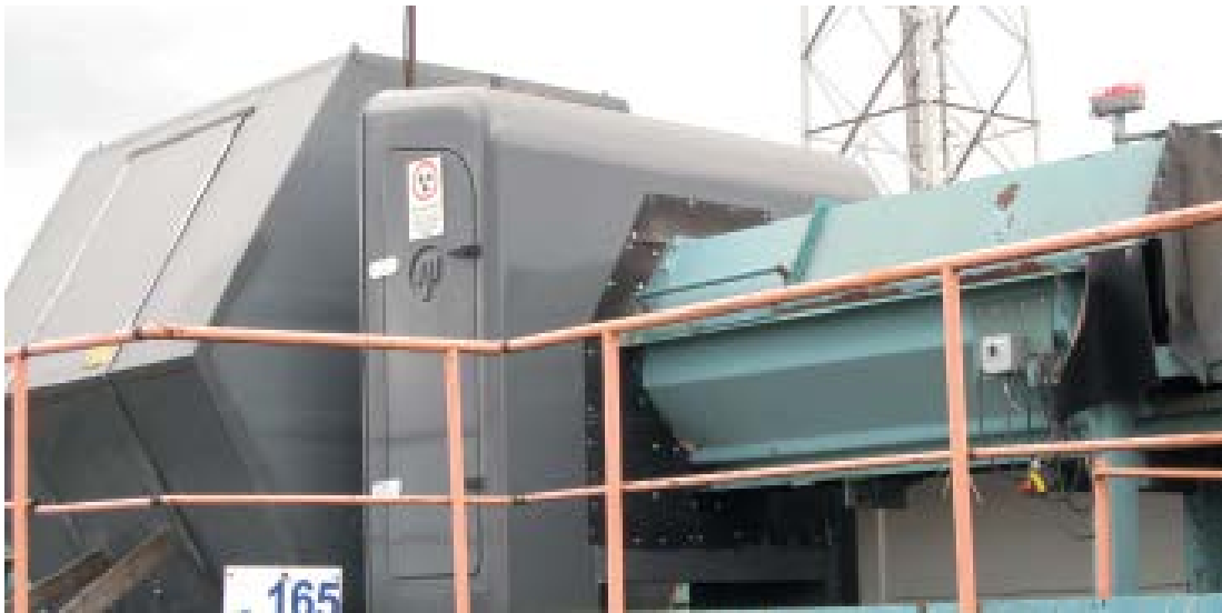
Figure 6. X-ray log scanner. (Inray.fi, 2019)
