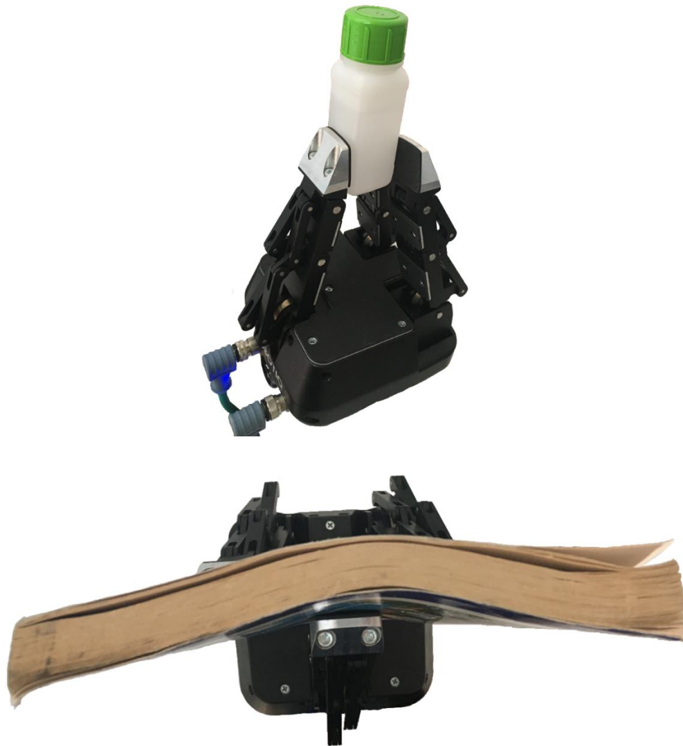
Figure 43. The gripper holding different objects.
