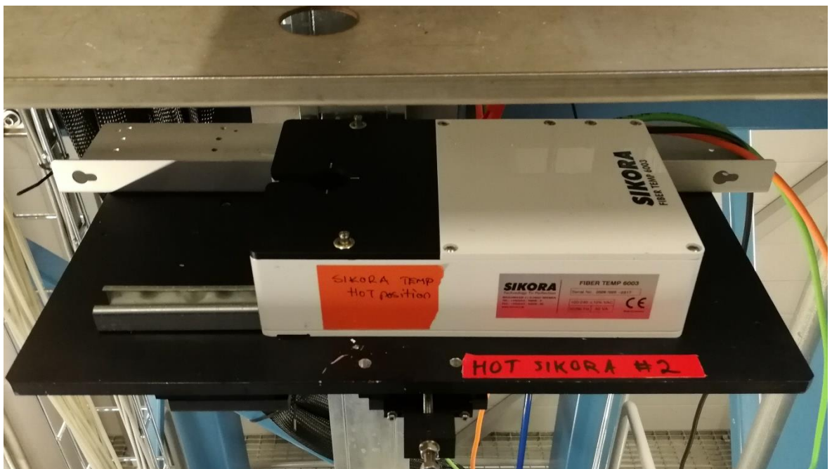
Figure 8. Hot fiber temperature measurement gauge: SIKORA FIBER TEMP 6003
