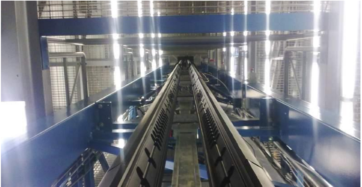
Figure 6. View upwards along the cooling tube of Nextrom Fiber Cooling System (FCS).
