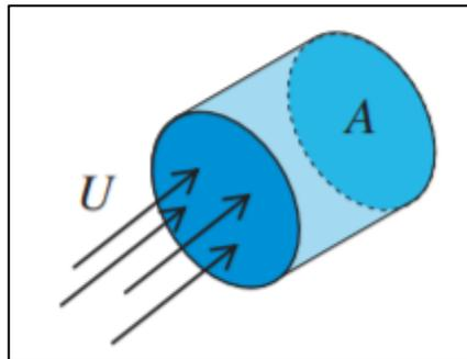
Figure 2. Air flow at velocity  $U$  through area  $A$ . (Letcher, 2017)
