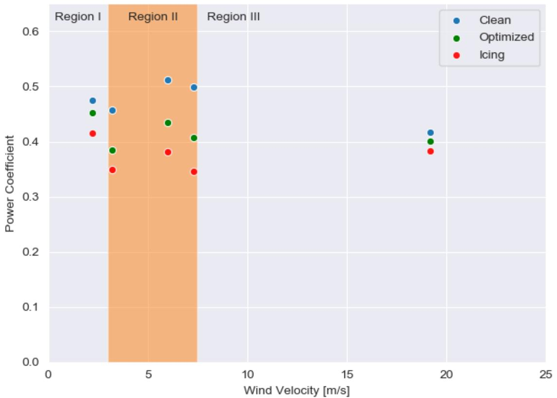
Figure 26. Combined results of the power coefficients with respect to wind velocity for the five references. Aerodynamic loss is a relation between the analysed power coefficient (optimized or non-optimized) with the power coefficient of the clean case and it is defined according to the following equation:
