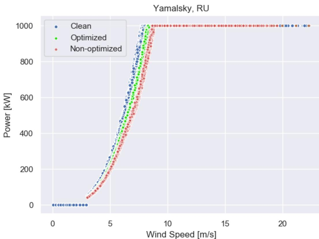
Figure 46. Superposition of the power curves in Yamalsky, RU.
