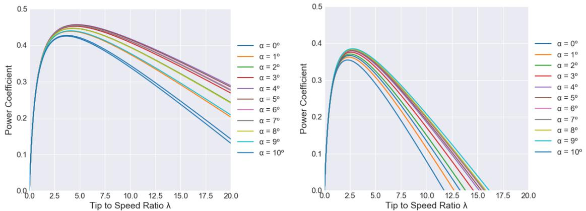
Figure 22. Curves of power coefficient for clean (left) and icing (right) cases for Hudecz (2014).
