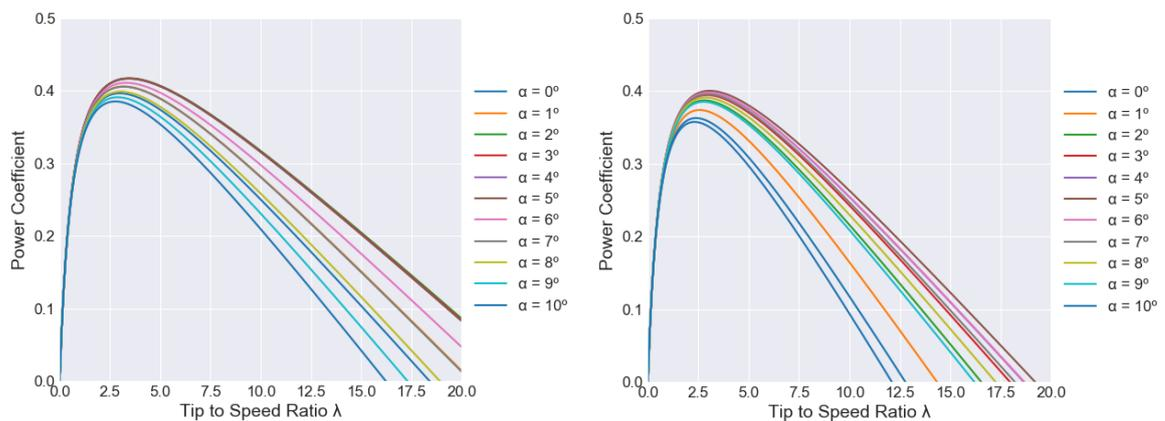
Figure 16. Curves of power coefficient for clean (left) and icing (right) cases for Homola et al. (2010).
