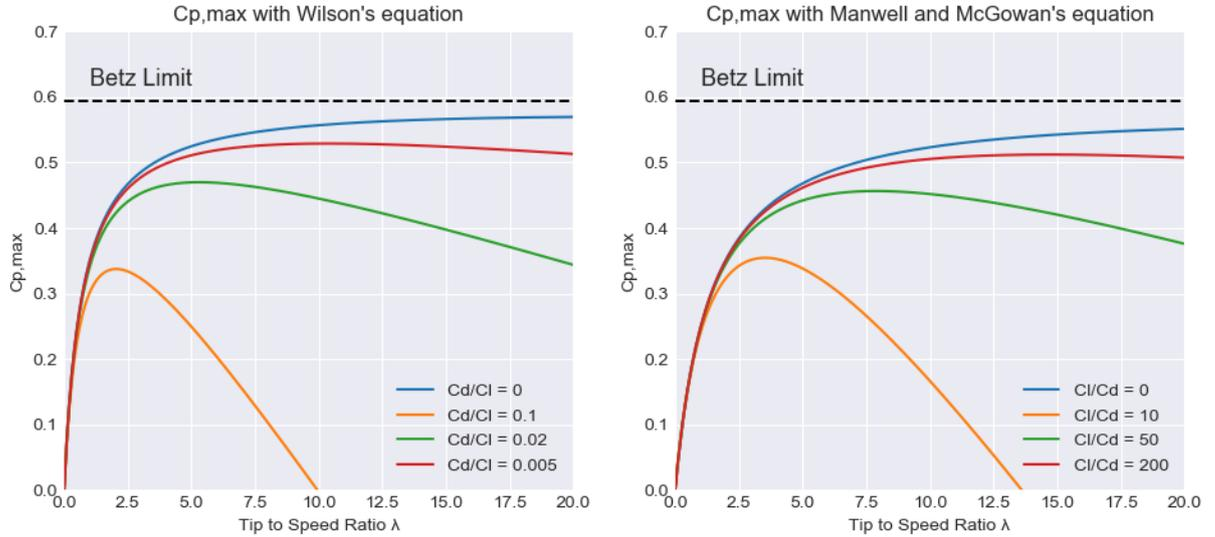
Figure 7. Comparison of the curves for maximum  $C_p$  according to different authors.
