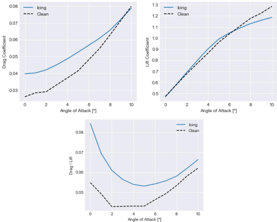
Figure 11. Drag coefficient (top left), lift coefficient (top right) and ratio drag/lift (bottom) for icing and clean airfoil by Homola et al. (2010).
