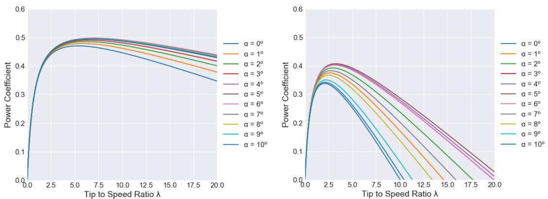
Figure 20. Curves of power coefficient for clean (left) and icing (right) cases for Turkia et al. (2013).
