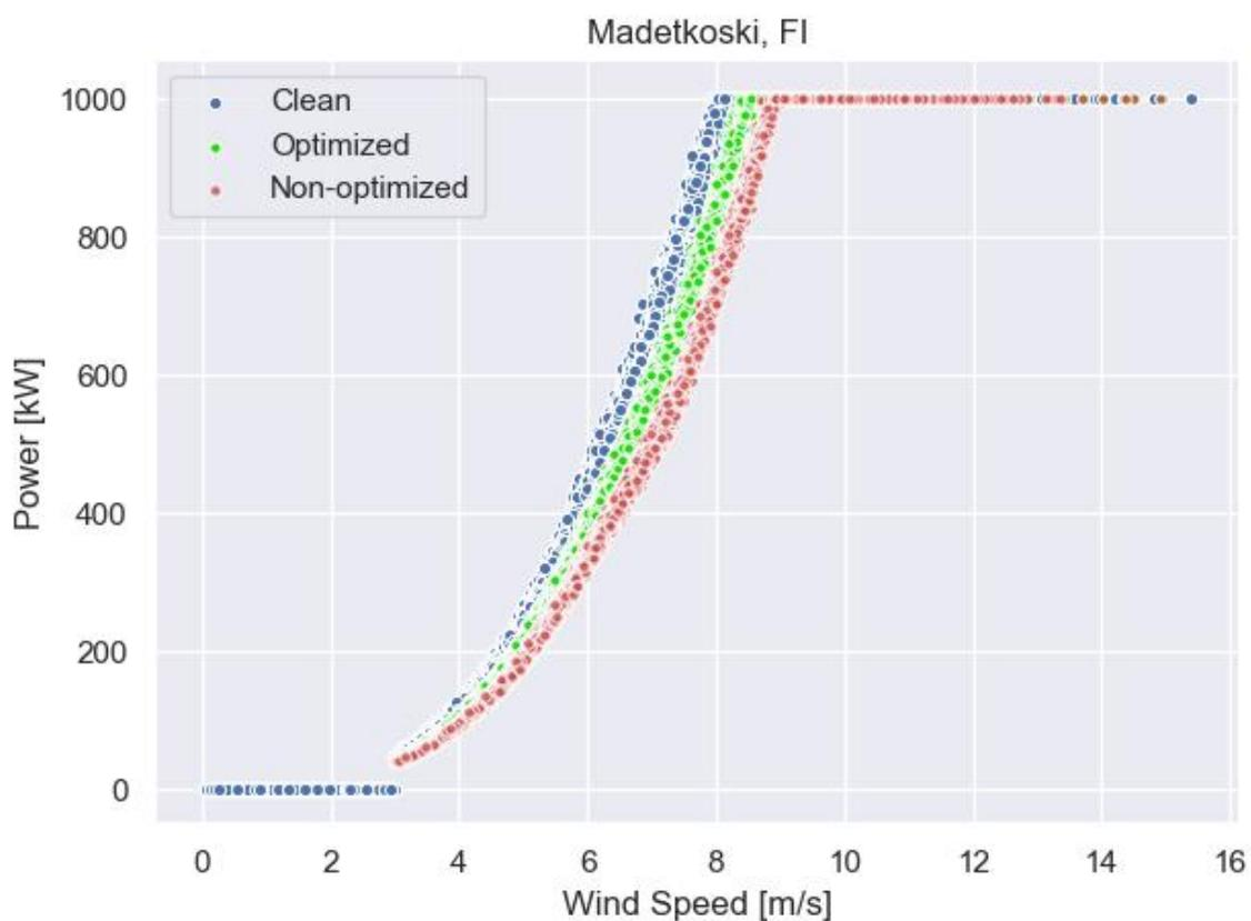
Figure 37. Superposition of the power curves in Madetkoski, FI.
