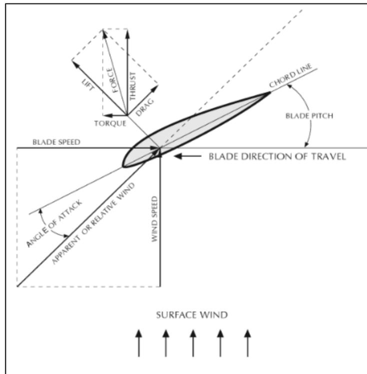
Figure 6. Pitch of the blade, angle of attack dependent of the wind direction and chord line, lift and drag forces depends on the angle of attack. (Gipe, 2004)
