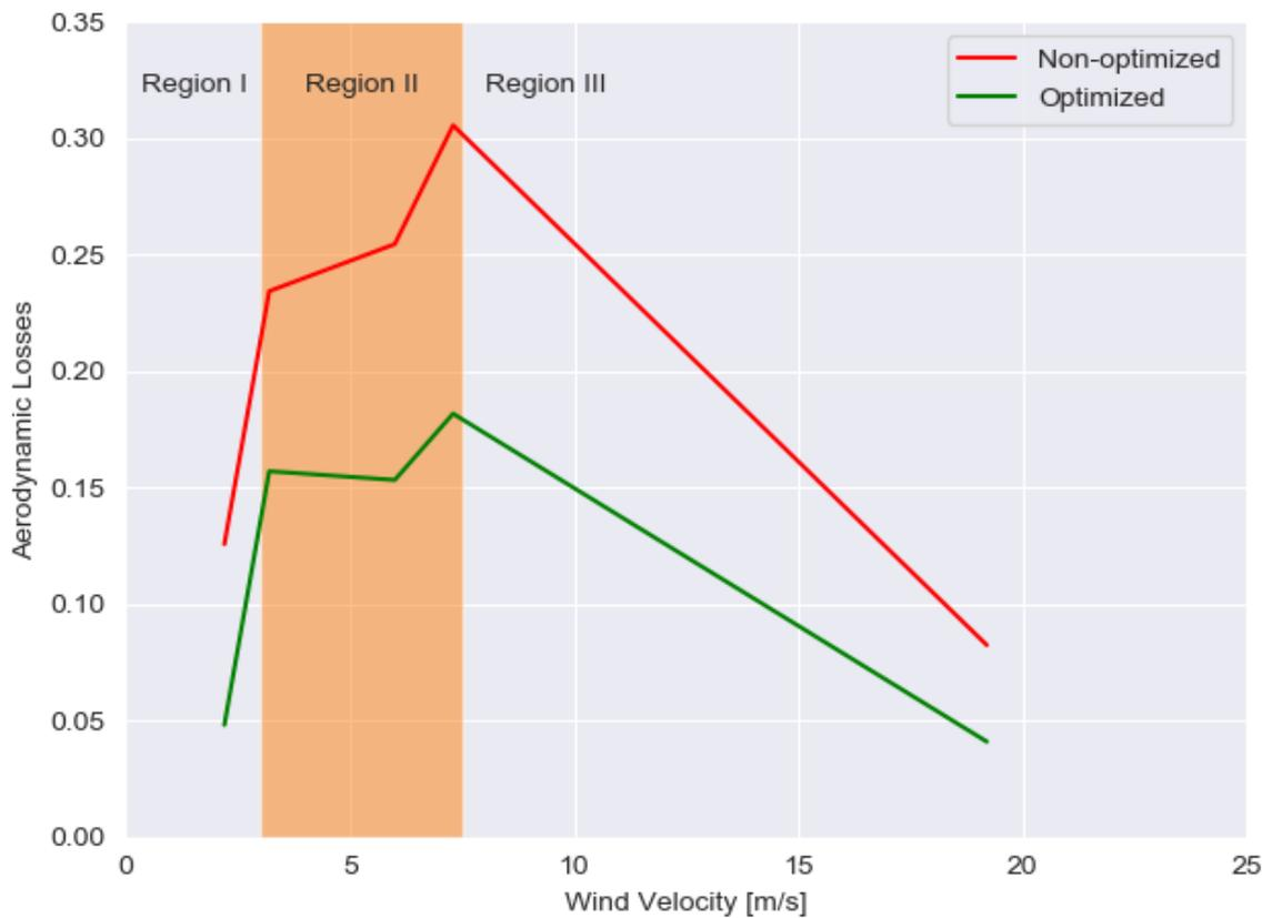
Figure 27. Combined aerodynamic losses of the icing and optimized cases with respect to the wind velocity for all five references.
