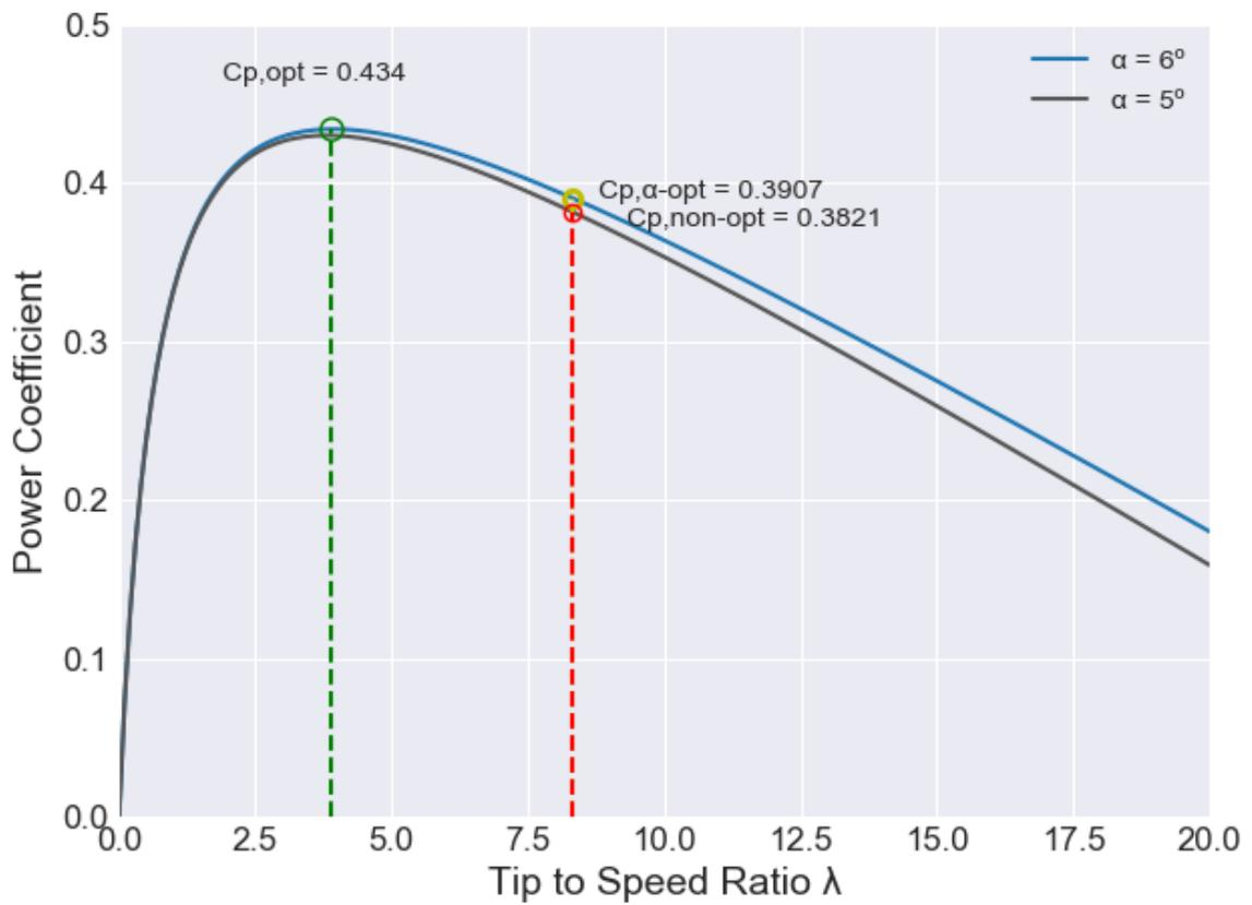
Figure 19. Analysis of the optimization method for Etemaddar et al. (2012).
