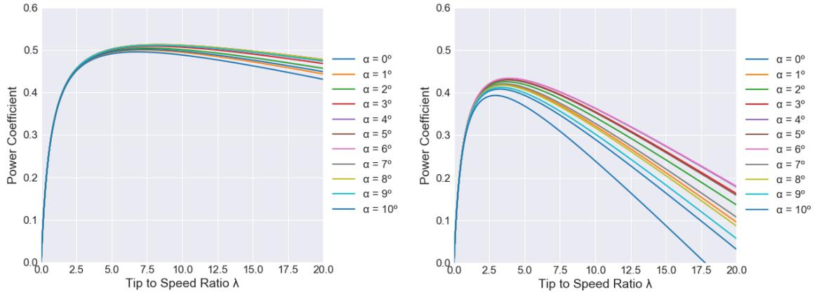
Figure 18. Curves of power coefficient for clean (left) and icing (right) cases for Etemaddar et al. (2012).
