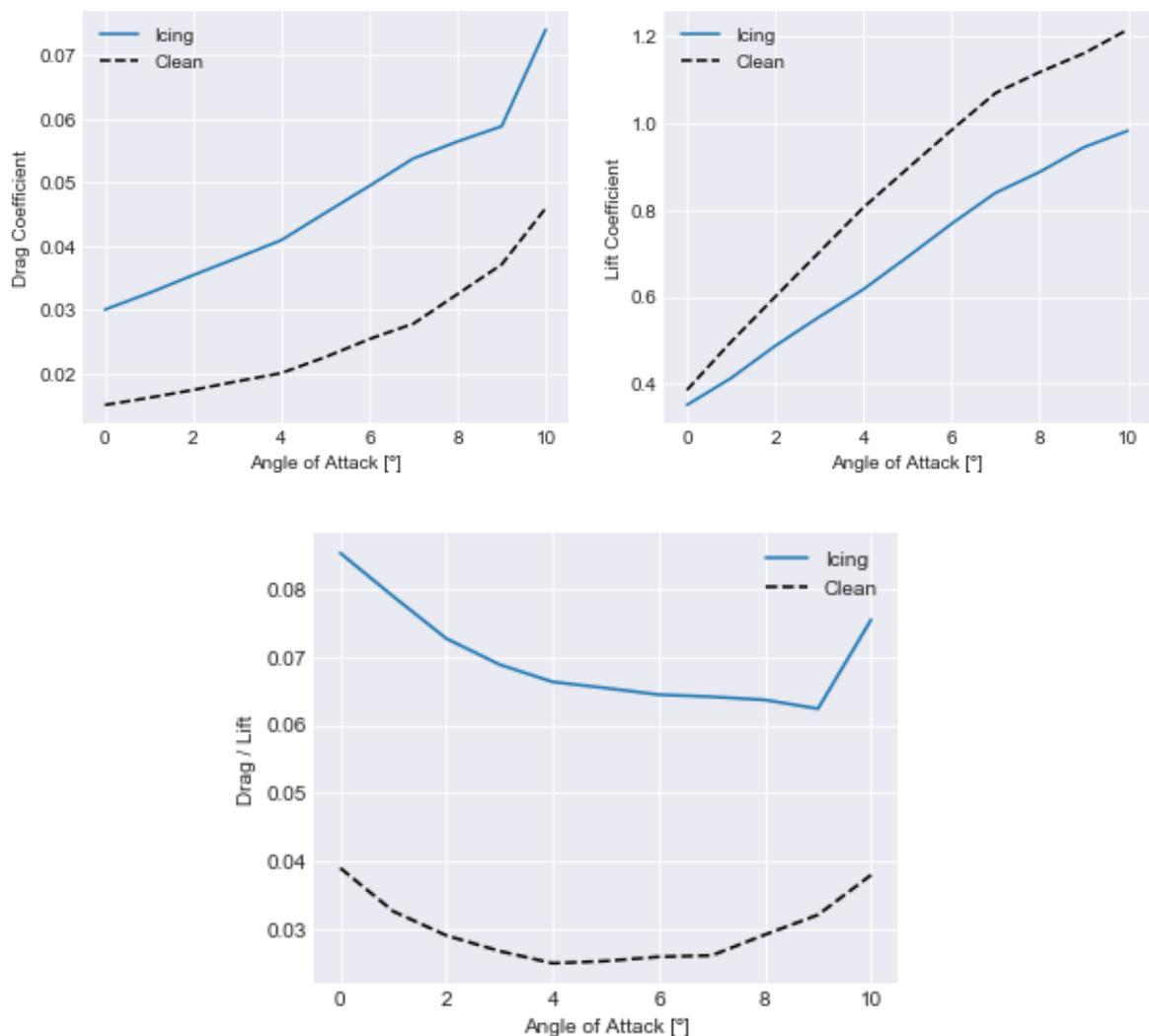
Figure 14. Drag coefficient (top left), lift coefficient (top right) and ratio drag/lift (bottom) for icing and clean airfoil by Hudecz (2014).
