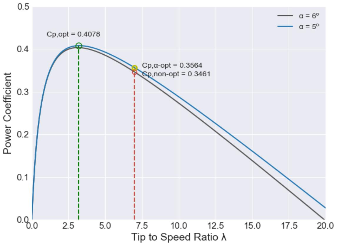
Figure 21. Analysis of the optimization method for Turkia et al. (2013).
