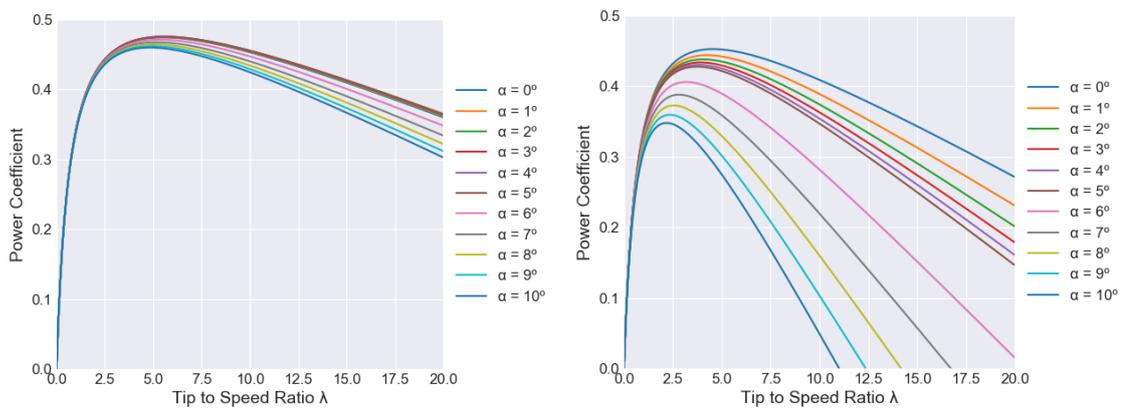
Figure 24. Curves of power coefficient for clean (left) and icing (right) cases for Gantasala et al. (2019)
