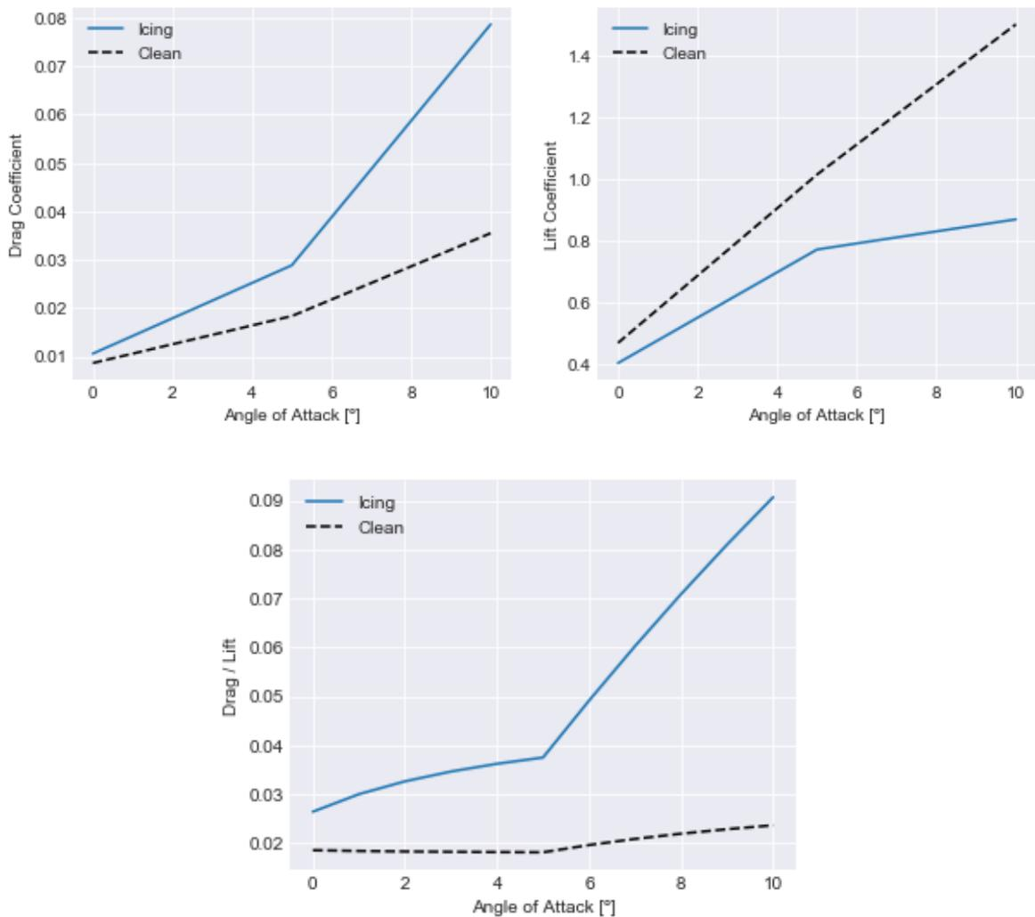
Figure 15. Drag coefficient (top left), lift coefficient (top right) and ratio drag/lift (bottom) for icing and clean airfoil by Gantasala et al. (2019).
