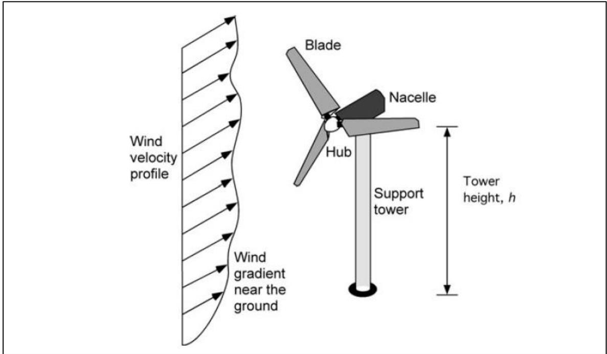
Figure 4. Wind turbine general structure. (Letcher, 2017)
