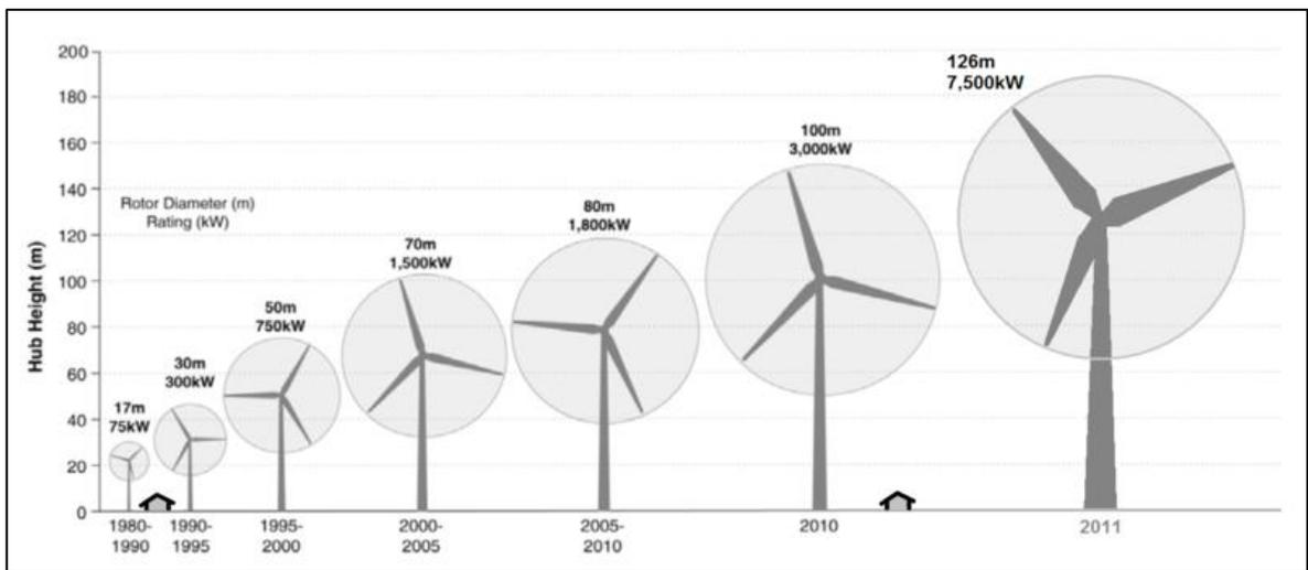
Figure 3. Size evolution of wind turbines over time. (Lantz, Hand, & Wiser, 2012)
