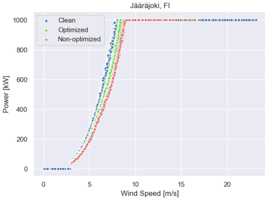
Figure 31. Superposition of the power curves for Jääräjoki, FI.
