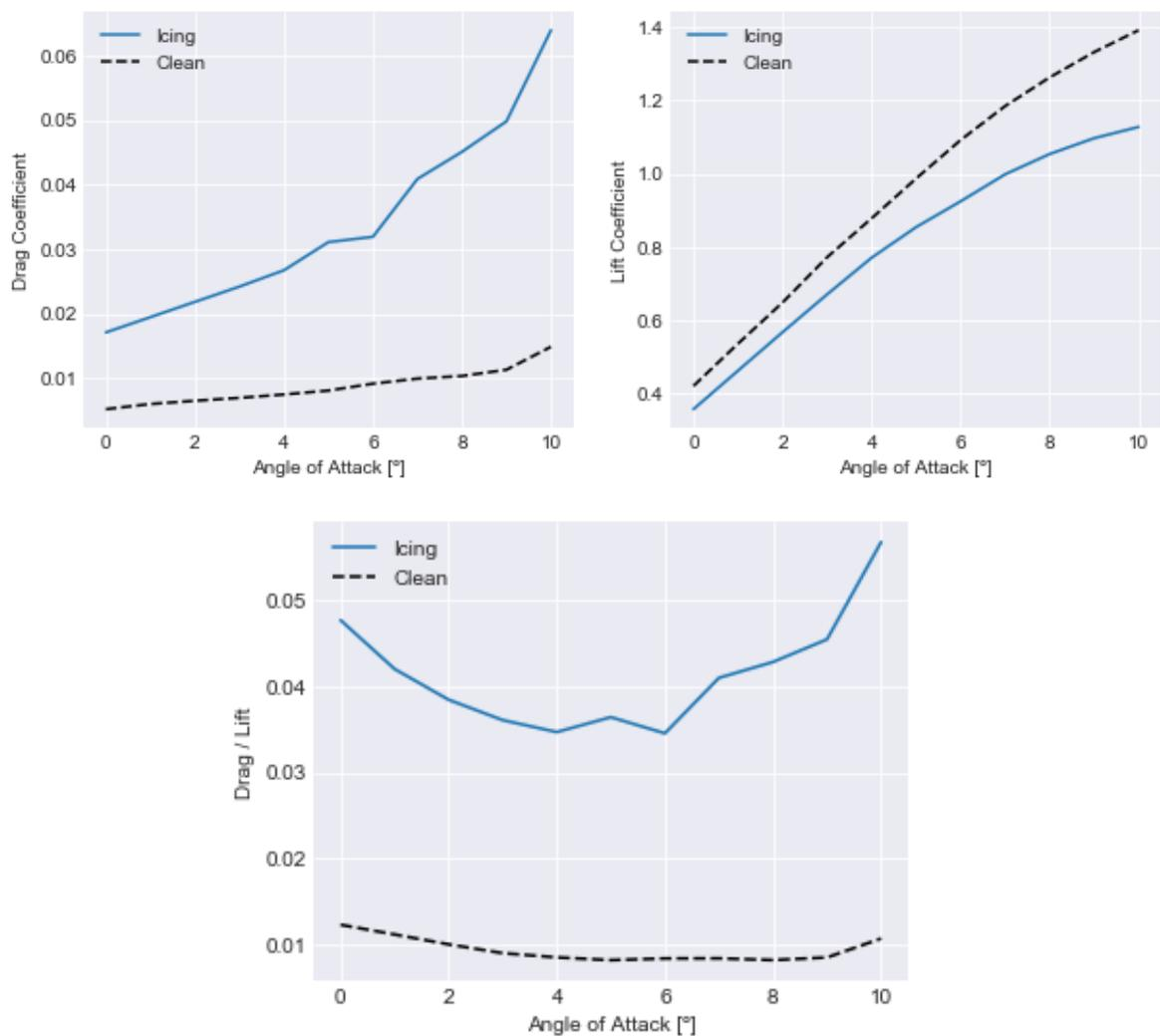
Figure 12. Drag coefficient (top left), lift coefficient (top right) and ratio drag/lift (bottom) for icing and clean airfoil by Etemaddar et al. (2012).
