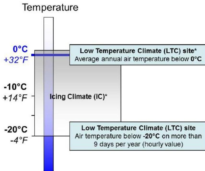
Figure 10. Low temperature and icing climate. (IEA Wind Task 19, 2017)
