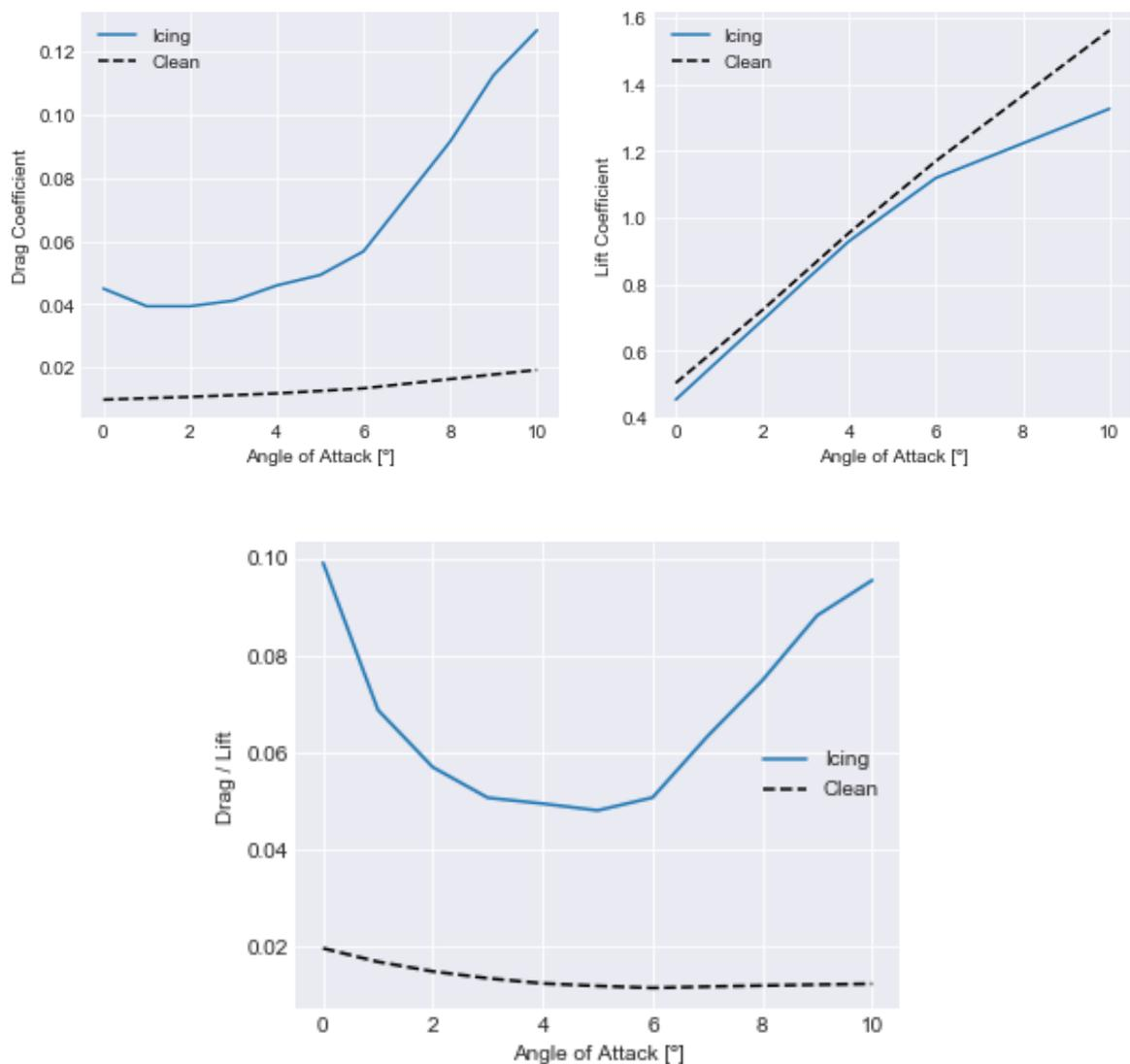
Figure 13. Drag coefficient (top left), lift coefficient (top right) and ratio drag/lift (bottom) for icing and clean airfoil by Turkia et al. (2013).
