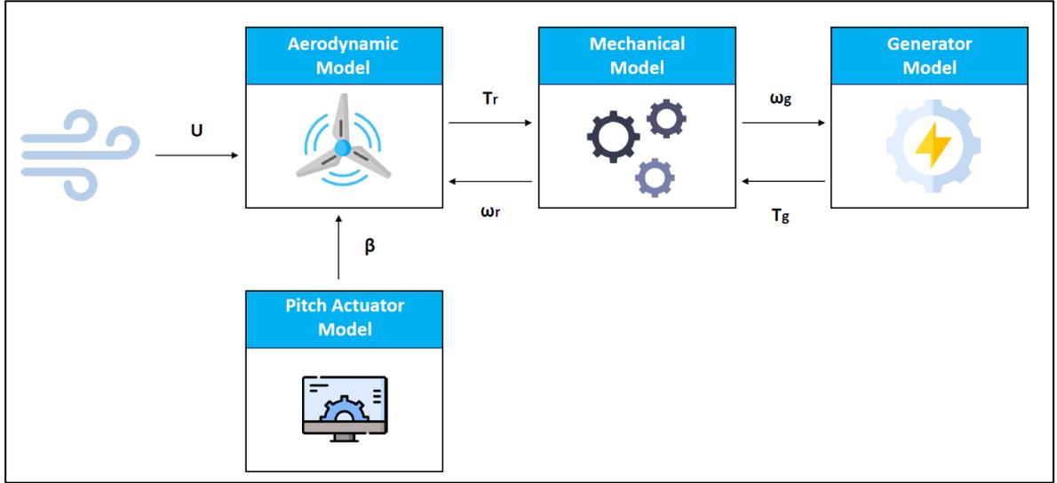
Figure 5. Interconnection of sub-models describing the characteristics of the wind turbine. (Thomsen, 2006)
