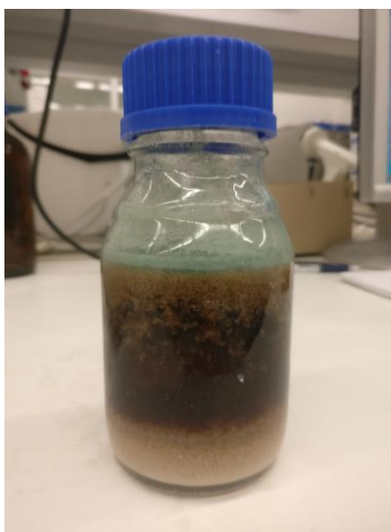
Figure 26 Cotton/polyester degradation product solution.
