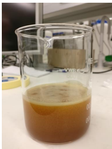
Figure 24 Acrylic fibers resulted in a thick liquid with no visible textile pieces.
