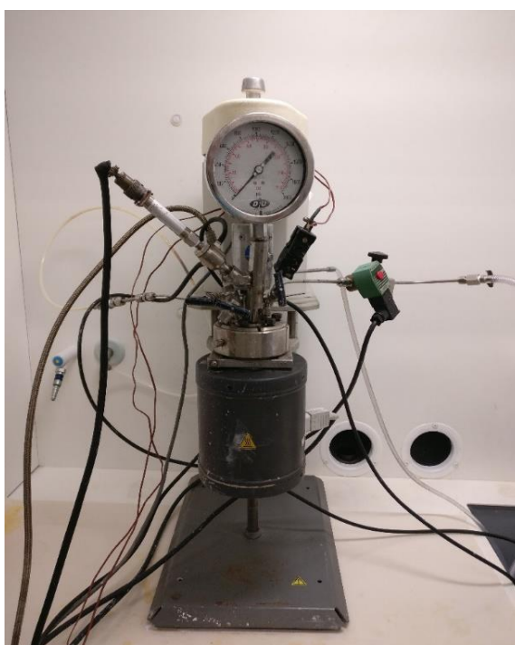
Figure 16 Autoclave used for the experiments.
