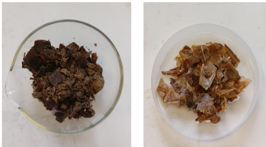
Figure 23 Leftover mass of polyester (left) and polyamide (right)
