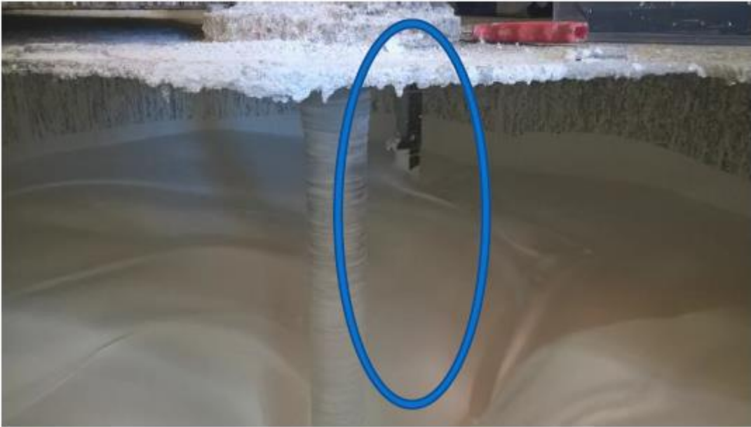
Figure 31. Collo sensor submerged in paint mixing vessel (Collo-technology 2018)
