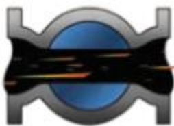
Figure 27. When the plug valve is open, the seats are well protected (Flowserve2017)
