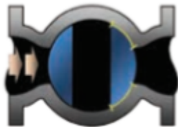
Figure 26. Plug valve is valve in-line maintainable
