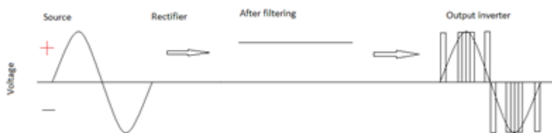
Figure 9. Principle waveforms of a voltage-source frequency converter: DC bus filtering creates almost smooth DC voltage. Output pulses of the inverter are formed with many pulses per half period.
