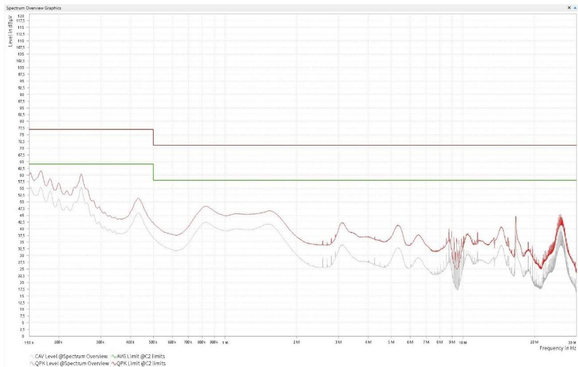
Figure 9. The conducted emissions with bypass circuit, added CM inductors and 33 nF Y-capacitors in the DC link. The emissions are under the required level (green line).
