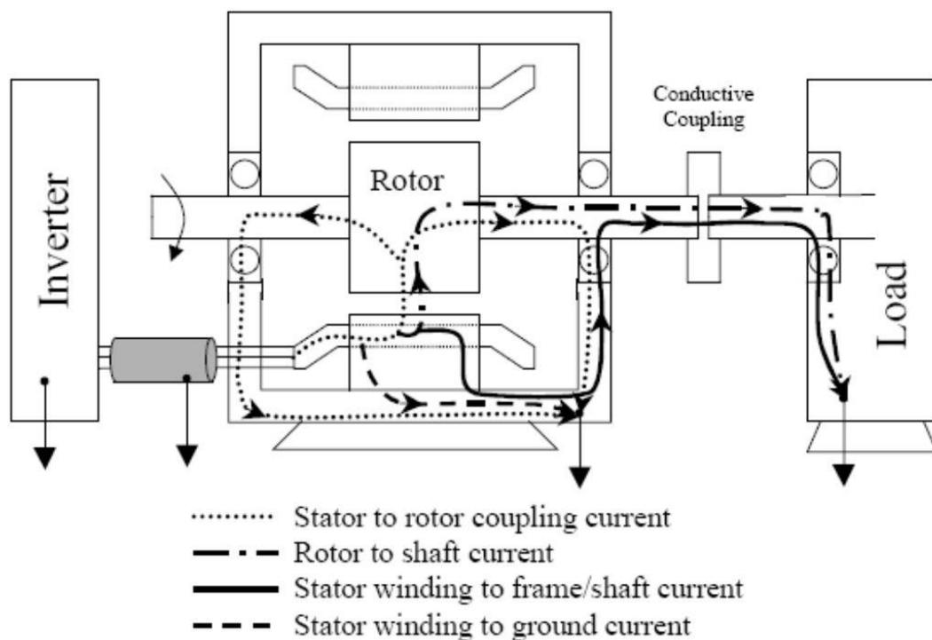
Figure 5. Leakage currents couple from the windings to the frame and rotor and can flow through bearings which causes wear to the bearings (Thakar et. al. 2015).
