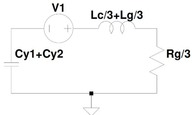
Figure 4. A common mode equivalent circuit. Capacitors  $C1 \dots C3$  do not appear in the equivalent circuit.
