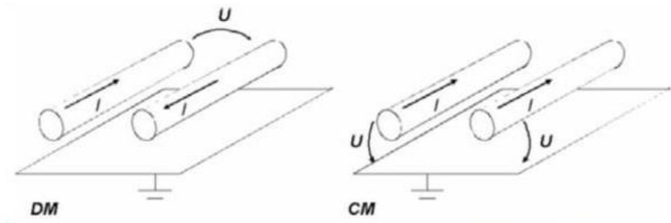
Figure 1. Differential mode voltage is the voltage between the main wires carrying signal or power. The common mode voltage is the voltage sum between the signal or power wires and the ground potential.
