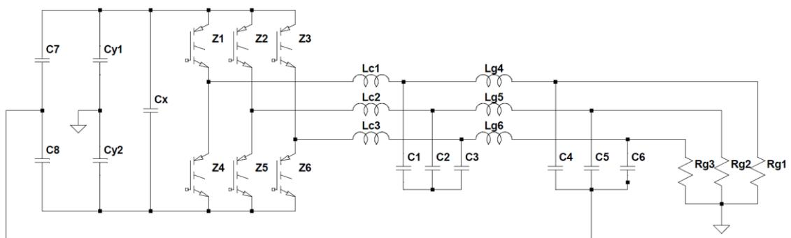
Figure 7. Bypass capacitors C4...C8 connected from the AC phases to the DC-link.
