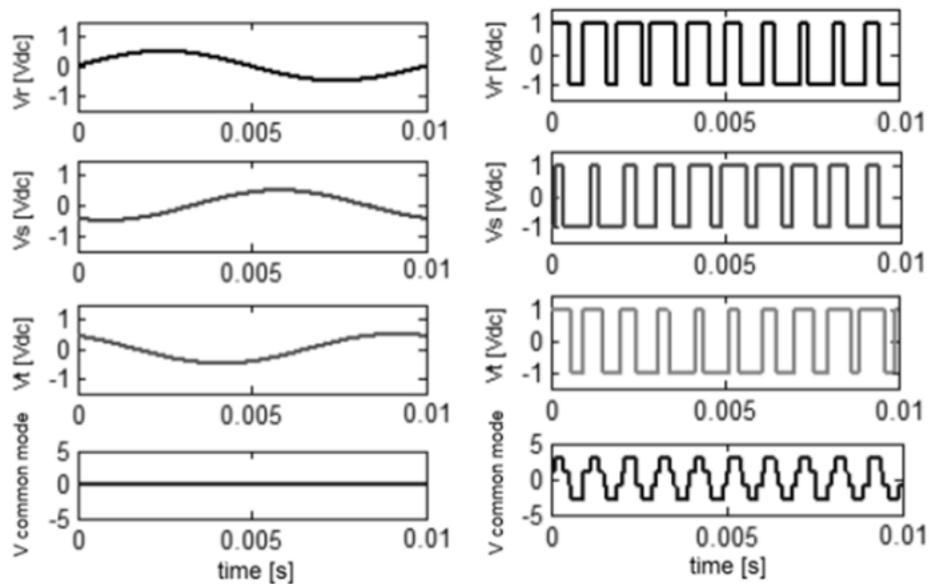
Figure 2. The common mode voltage is a sum of three phase voltages,  $V_r$ ,  $V_s$  and  $V_t$  (Prieto et. al., 2011).
