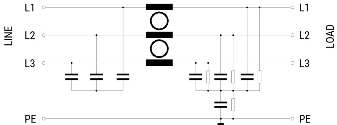
Figure 6. A typical commercially available AC filter circuit. Between the line input and the CM inductor, there are X-capacitors connected between the phases in Y-configuration. Between the CM inductor and the load output there are X-capacitors with a Y-capacitor connected from Y-point to the protective earth (PE). Resistors are connected in parallel to the load side capacitors to adjust the damping ratio. (KEMET, 2017)
