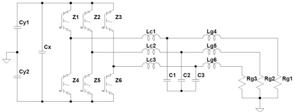
Figure 3. Three-phase inverter connected to a sinusoidal filter and a grid. DC-link Y-capacitance is drawn as two capacitors,  $C_{y1}$  and  $C_{y2}$
