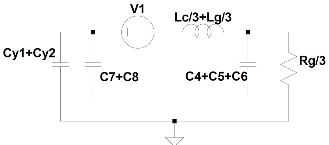
Figure 8. Equivalent circuit with the bypass capacitors.
