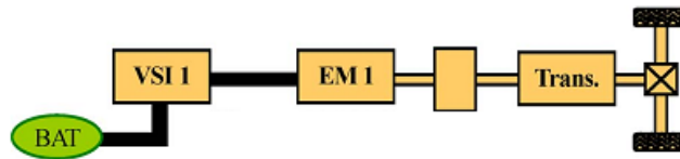
Figure 4. Architecture of a battery-powered electric vehicle (adopted from Chan et al., 2010).
