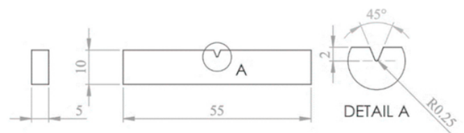
Fig. 3. Schematic of the Charpy impact specimen and the notch detail. (Unit in mm, not to scale).
