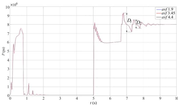
Fig. 6. Pressure response of the lift cylinder versus time excited by a step input
