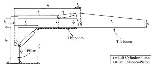
Fig. 2. A schematic of the jib crane model
