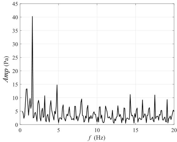
Fig. 5. Frequency versus the pressure amplitude at air volume fraction 1.9 and frequency 5 Hz
