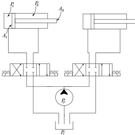
Fig. 3. The schematic of the hydraulic circuit for the case study
