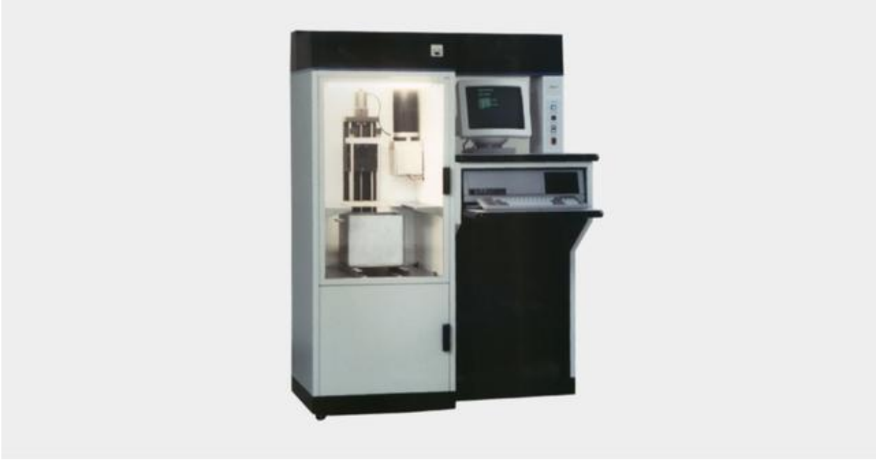
Figure 1.12. The first 3D printer (3D Systems, 2020)
