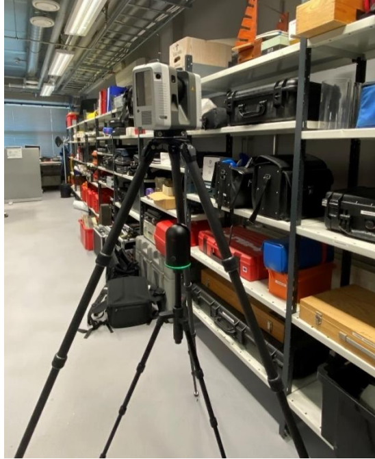
Figure 2.1. Leica RTC360 (the big one) and Leica BLK360 (the small one)
