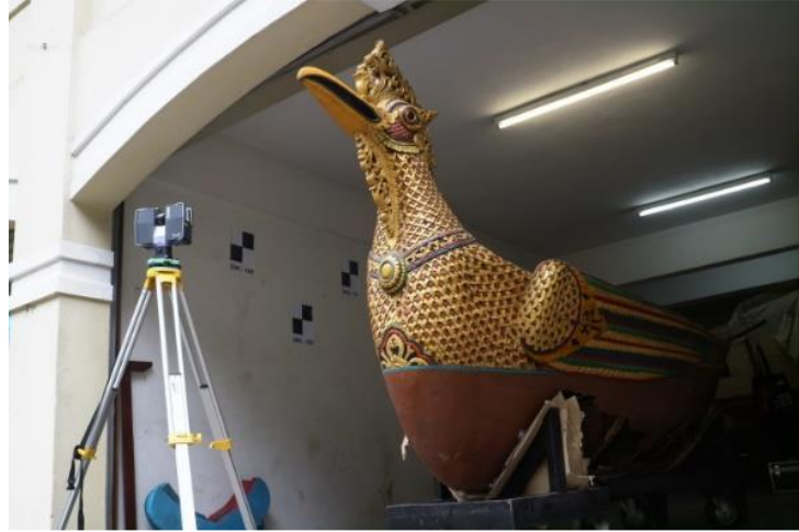
Figure 1.8. Scanning process of a boat (Sharif, et al., 2018, p. 3).
