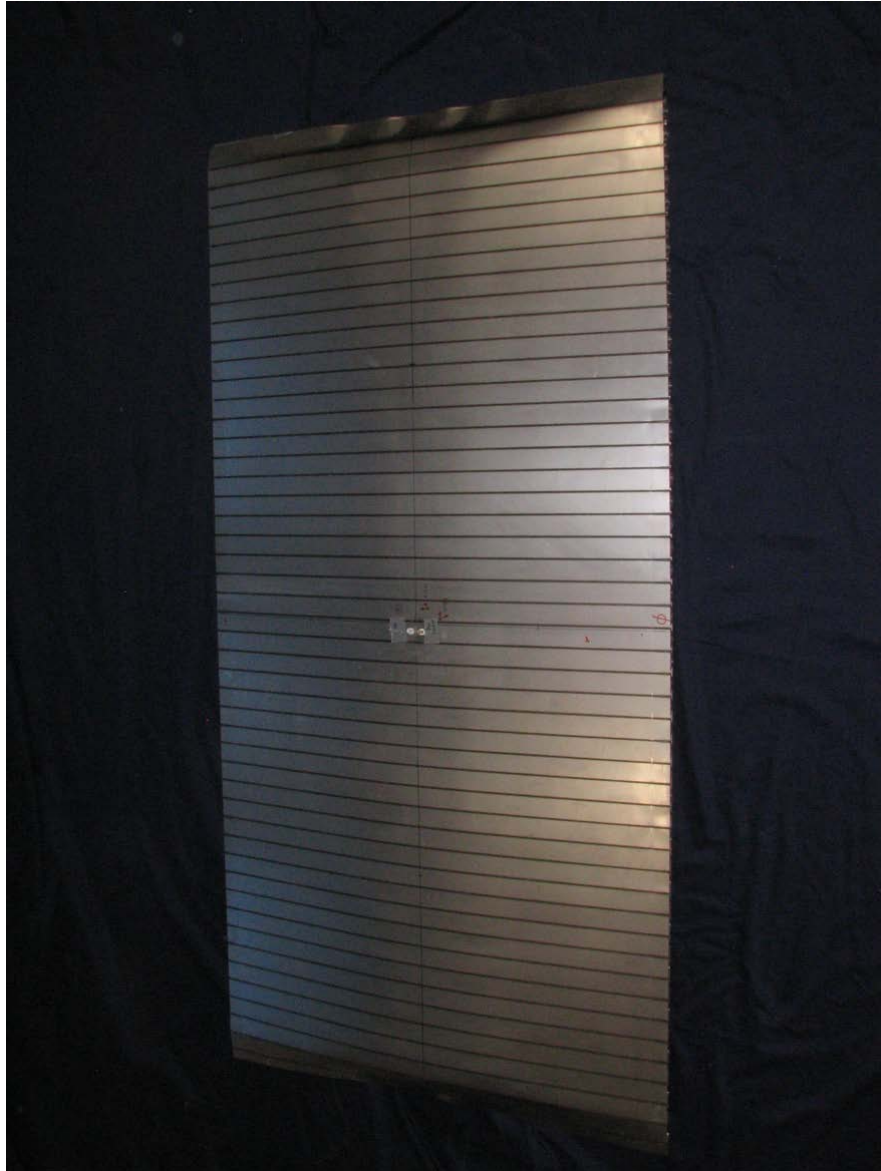
Figure E.10. The lower side of the KV-2 shows little plastic deformation except the edges.
