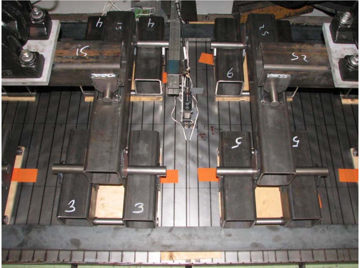
Figure E.3. The upper plate of KV-2 has buckled, as happened with KV-1.
