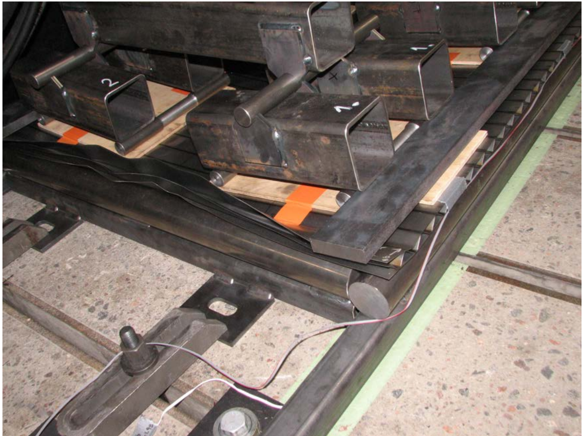
Figure E.7. Due to very pronounced plastic hinge, the left edge has lost its loading capacity, and the right edge carries more loading.
