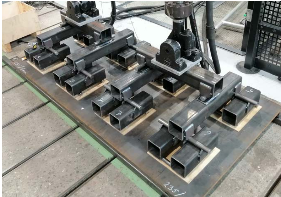
Figure 15. Proofing the test device with 8 mm steel plate of S235. Cylinder support is missing.
