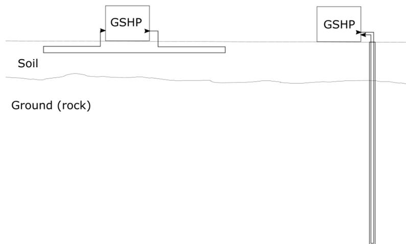
**Figure 6.** Horizontal and vertical GHE's.
