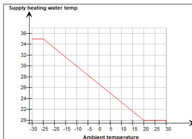
**Figure 2.** Space heating temperature control (screenshot from IDA-ICE).
