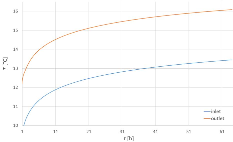
**Figure 19.** Inlet and outlet temperature evolution from  $t = 1$  to  $t = 64$  h, linear scale.
