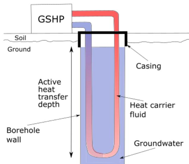
**Figure 7.** Side view of a borehole heat exchanger, not in scale.
