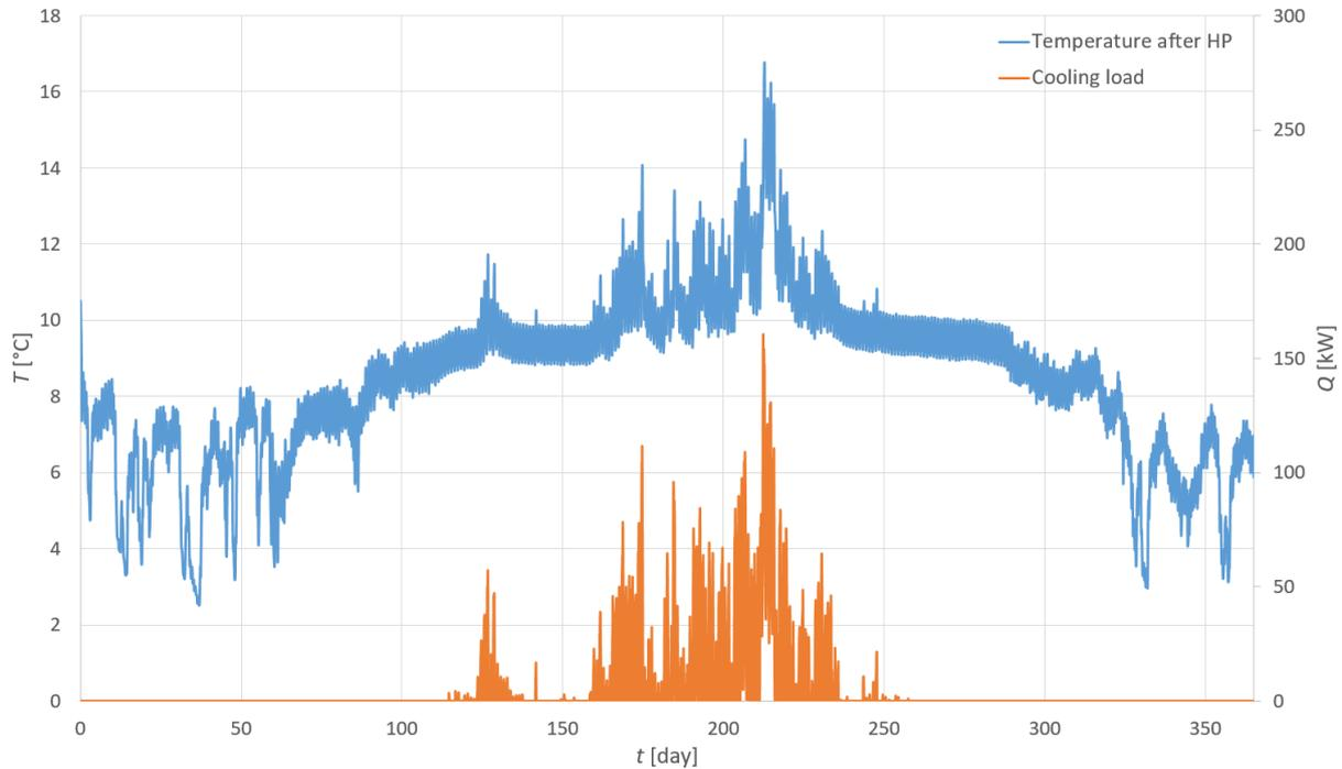
**Figure 34.** 1<sup>st</sup> year heat carrier temperature after HP displayed along the annual cooling load profile.
