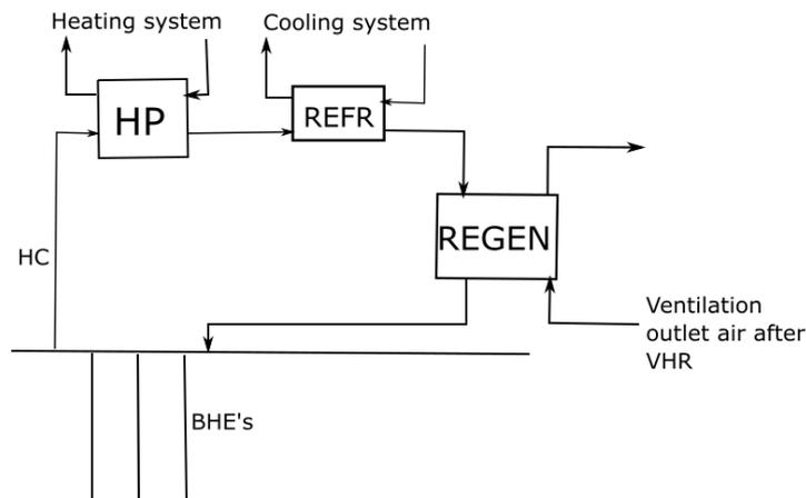
**Figure 25.** Illustration of the regeneration heat exchanger's position in the system.
