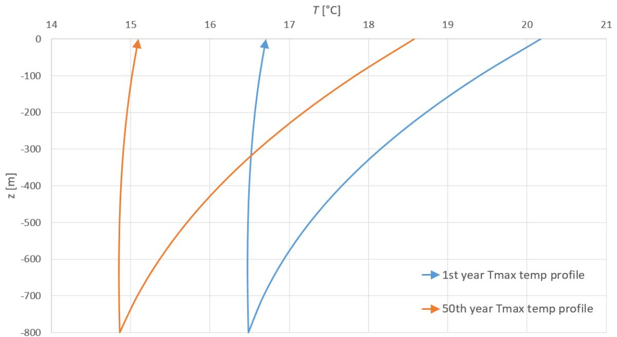
**Figure 31.** 1st year and 50th year vertical temperature profile during peak maximum temperature.
