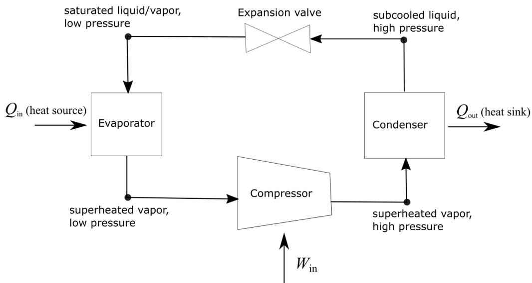
**Figure 4.** Vapor compression cycle working principle.
