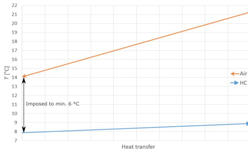
**Figure 26.** Regeneration heat transfer diagram, at an arbitrary time.
