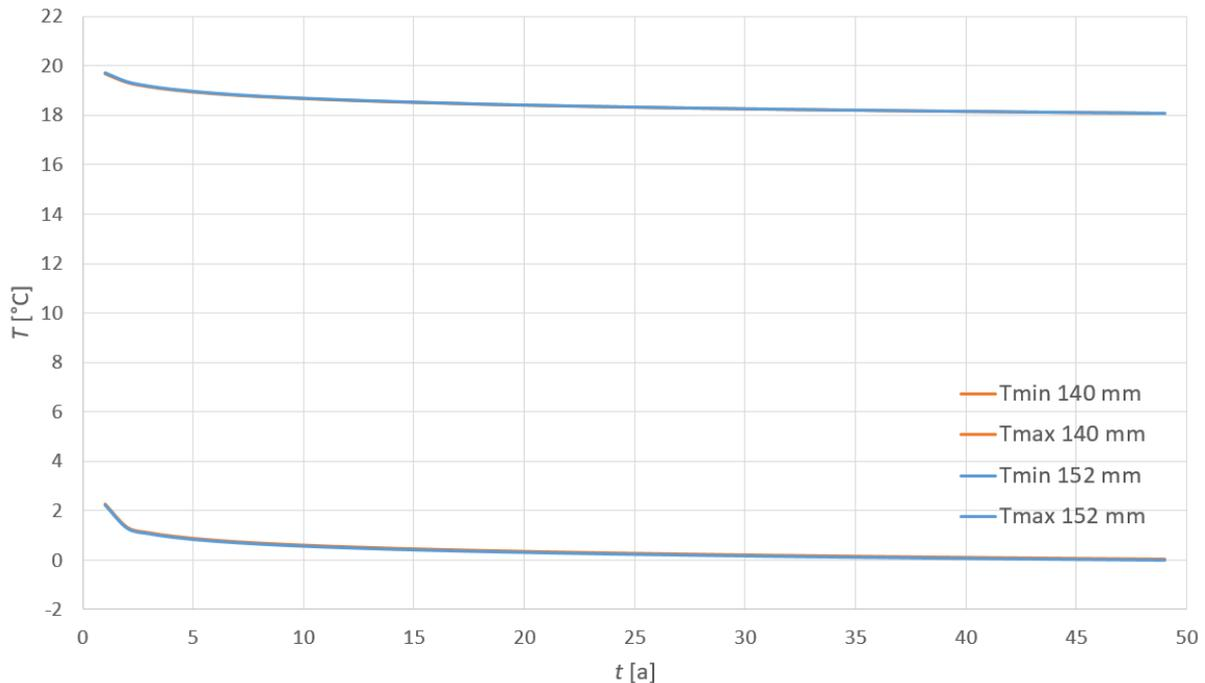
**Figure 33.** The effect of borehole diameter on the min/max mean fluid temperatures with improved grout  $k$ .
