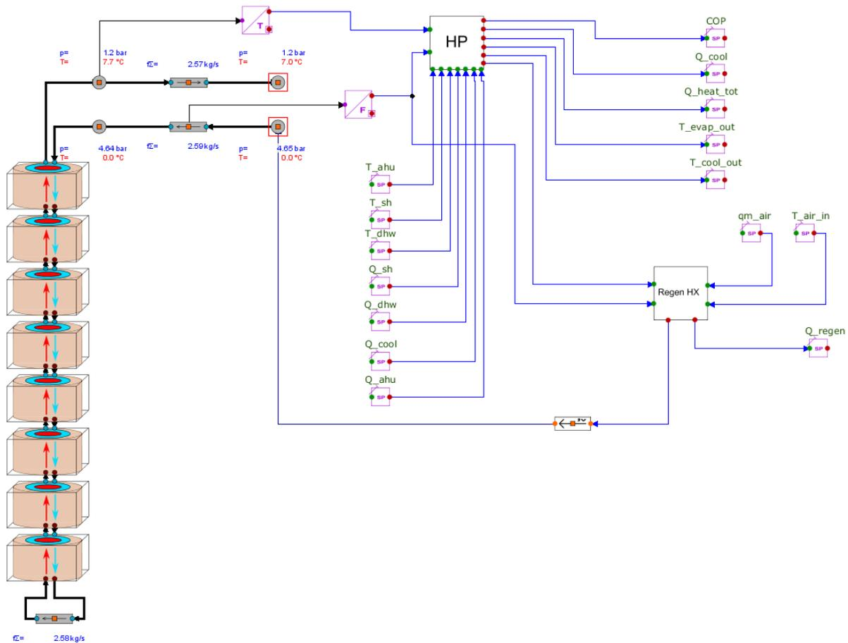
**Figure 18.** Screenshot of the Apros configuration window, with the HP module connected to the BHE model.
