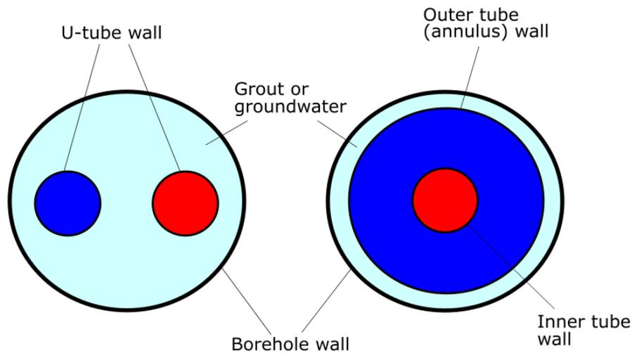
**Figure 9.** Cross-sections of a u-tube BHE and CBHE.
