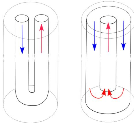
**Figure 8.** Side views of u-tube BHE and CBHE.
