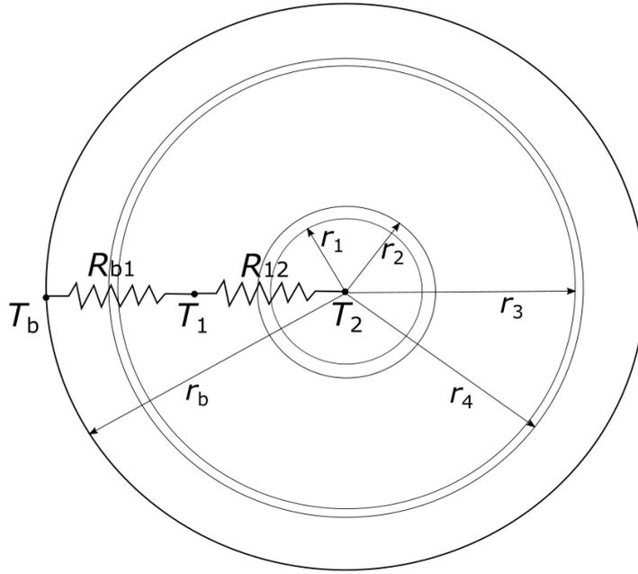
**Figure 10.** Heat transfer resistance network of a CBHE.
