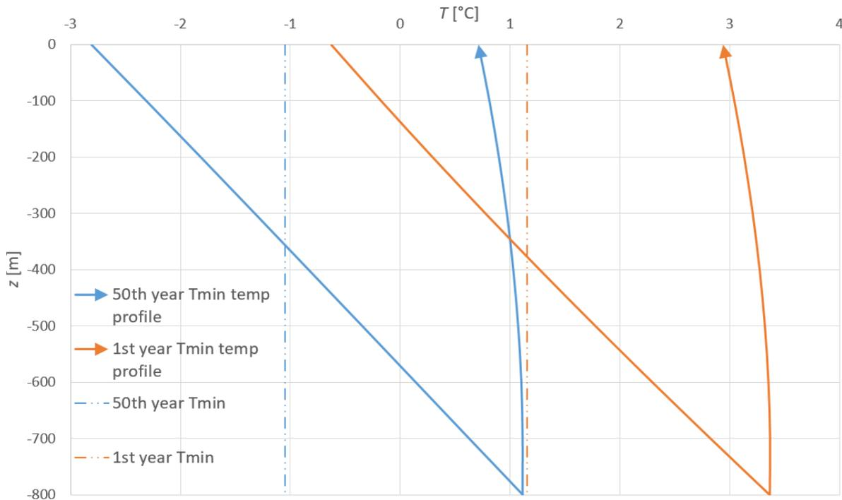
**Figure 30.** 1st year and 50th year vertical temperature profile during peak minimum temperature.
