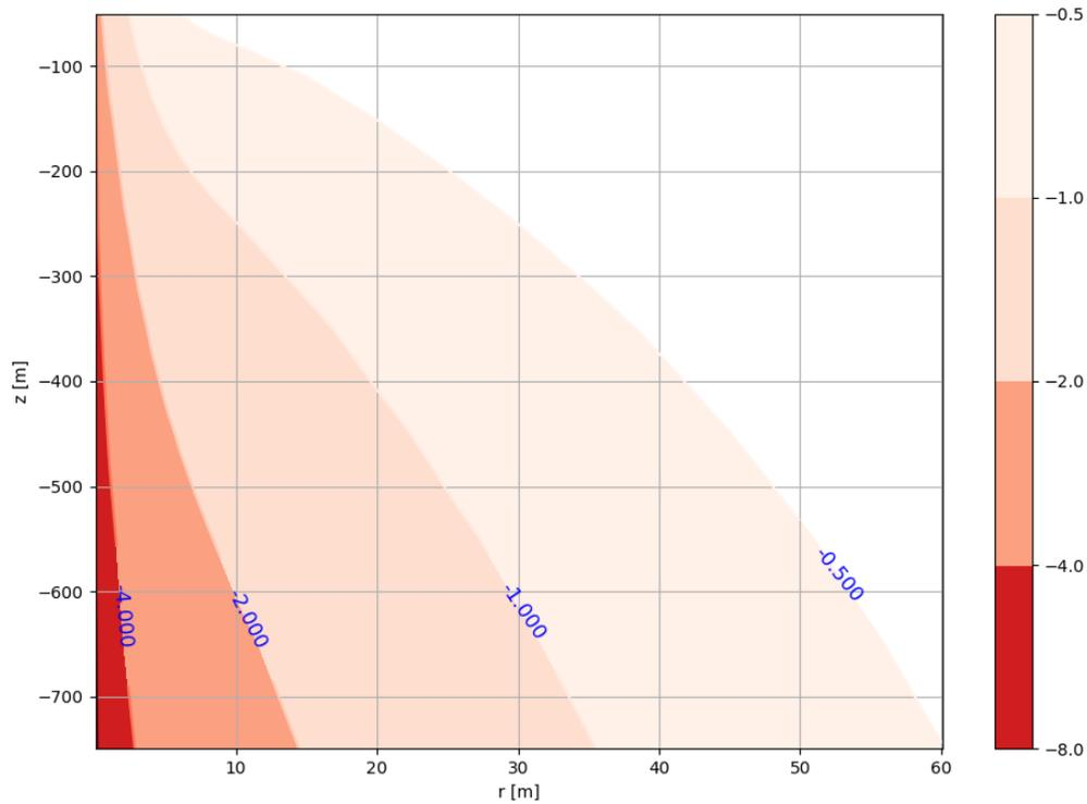
**Figure 37.** Ground temperature change contour after 50 years of operation, without regen.
