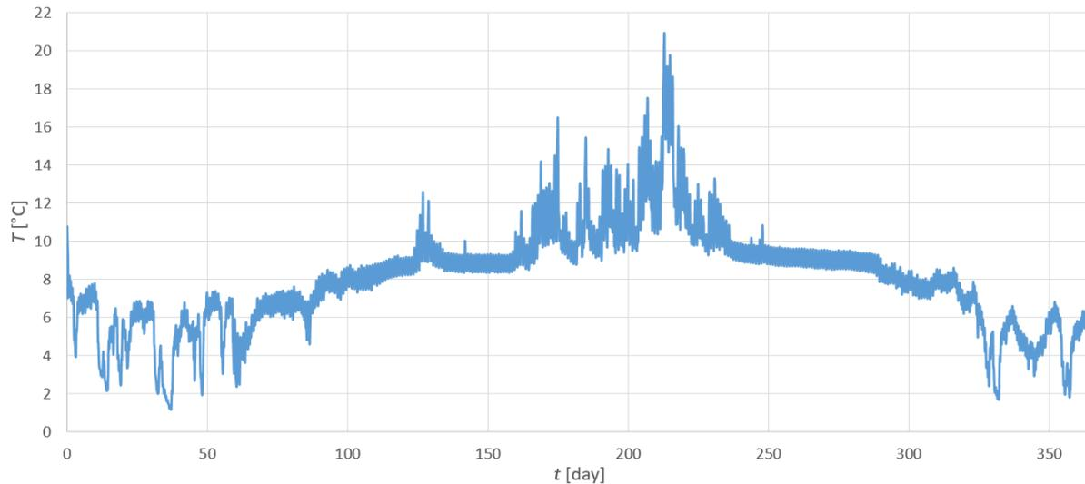
**Figure 28.** First year MFT profile (3 BHE's), 1 hour log interval.
