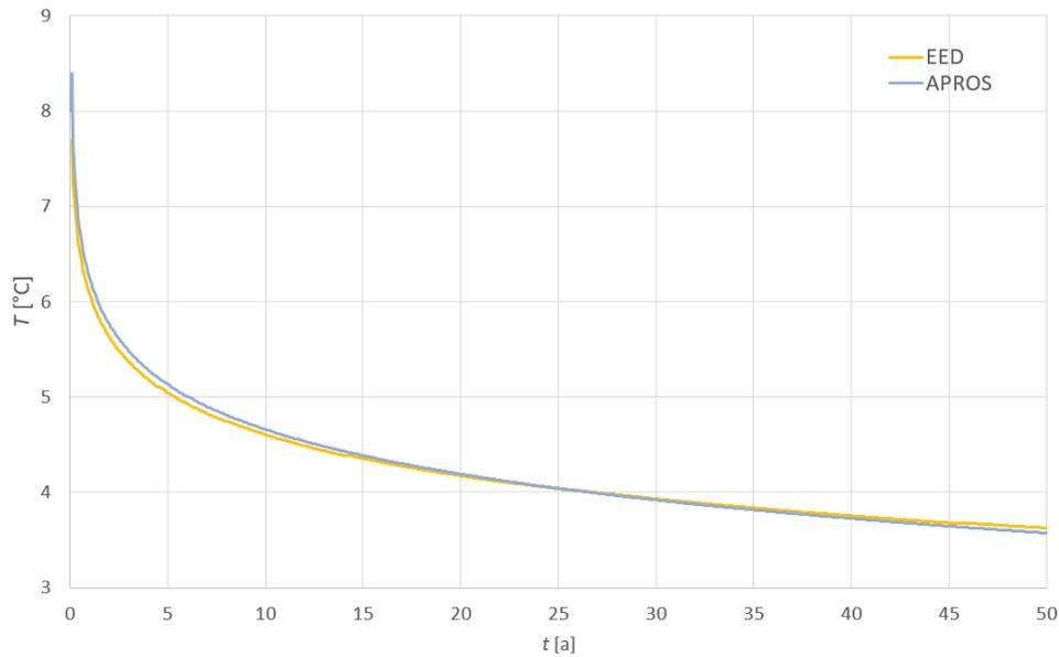
**Figure 22.** Mean fluid temperature (MFT) for 50 years, calculated with the Apros model and EED.
