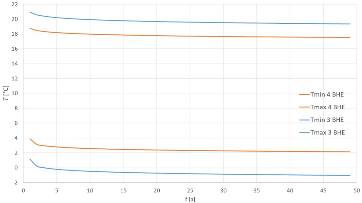
**Figure 29.** 50 year annual minimum and maximum of mean fluid temperatures, 3 BHE's vs. 4 BHE's.
