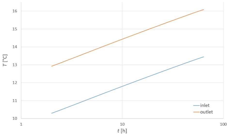
**Figure 20.** Inlet and outlet temperature evolution from  $t = 1$  to  $t = 64$  h, logarithmic scale.
