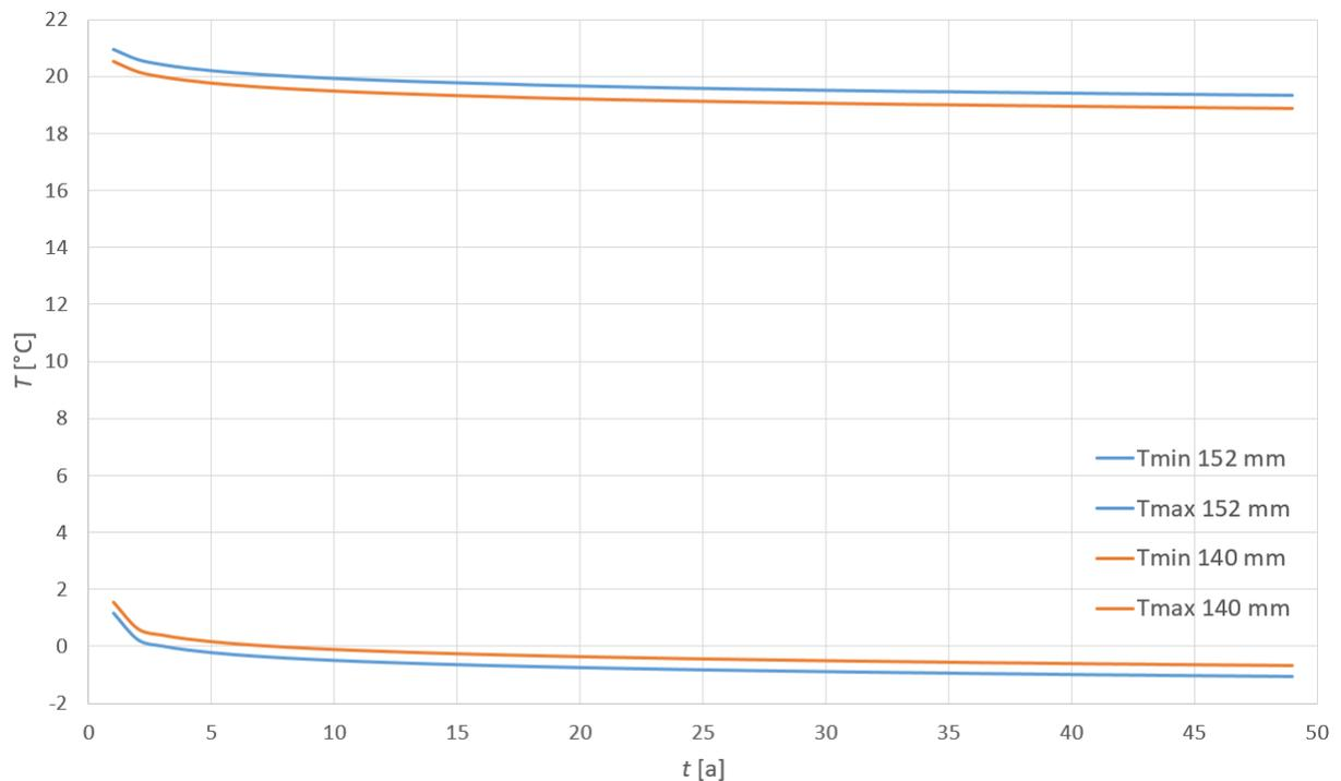
**Figure 32.** The effect of borehole diameter on the min/max mean fluid temperatures, 3 BHE's.
