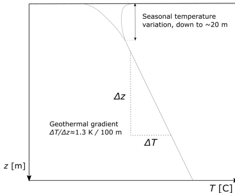
**Figure 5.** Visualization of ground heat fluxes and geothermal gradient.
