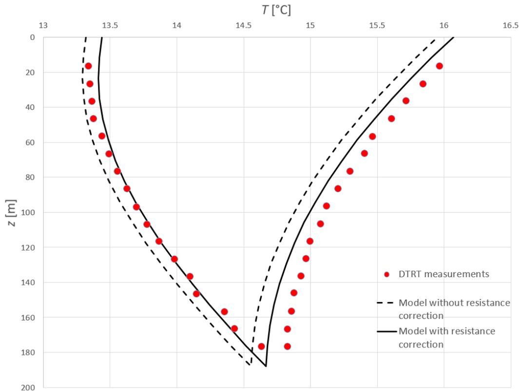
**Figure 21.** Heat carrier temperature profile at  $t = 63$  h, measurements and model output.
