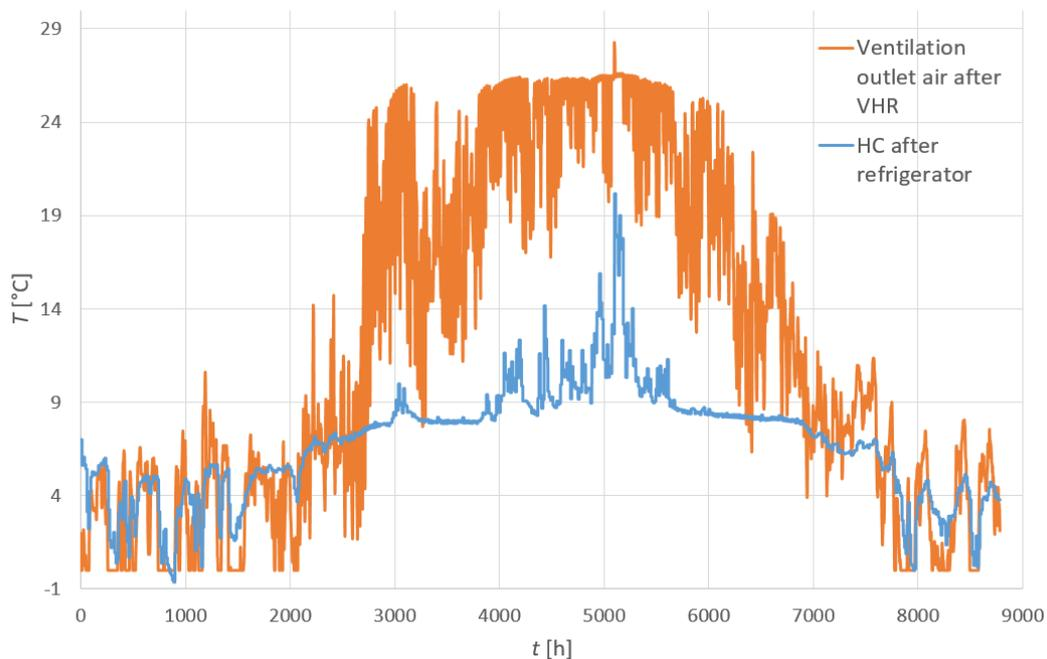
**Figure 24.** First year heat carrier temperature after refrigerator and VHR outlet temperature.
