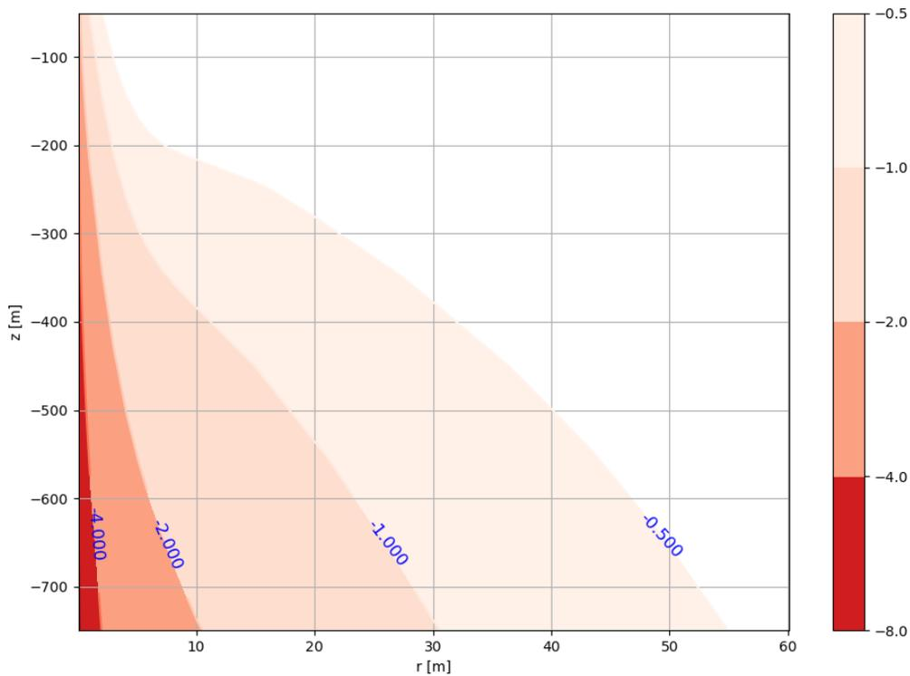
**Figure 38.** Ground temperature change contour after 50 years of operation, with regen.
