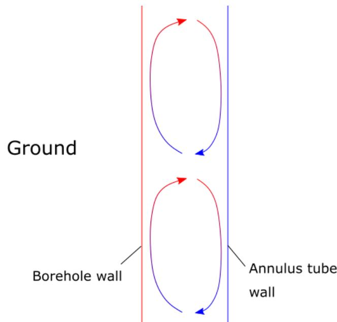
**Figure 11.** Groundwater movement by natural convection.
