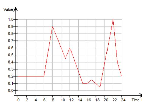
Figure 3. Example of the daily DHW consumption profile, scaled (screenshot from IDA-ICE).
