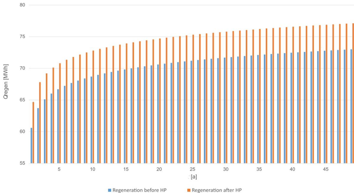
**Figure 35.** Annual available regenerative heat, heat exchanger before HP vs. after HP.
