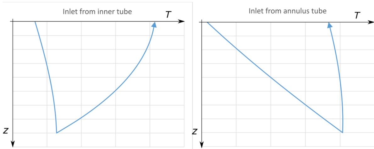
**Figure 12.** Heat carrier temperature profile shapes with inlet from inner tube and annulus.
