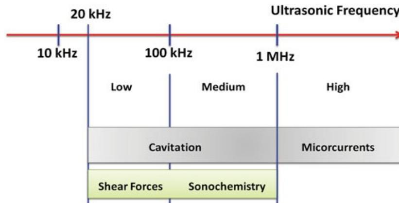
**Figure 6.** Ultrasonic frequencies and cavitation area (Kumar Tyagi 2014, p. 1223)
