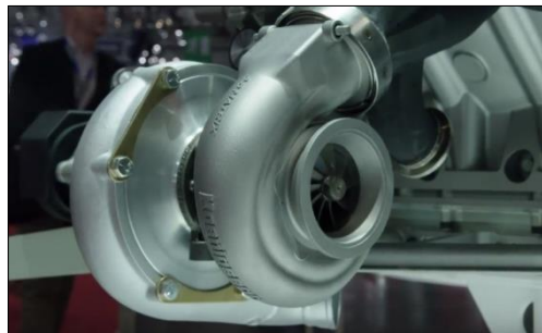
Fig. 9. World's first AM printed automobile turbocharger used in Koenigsegg One [26].
