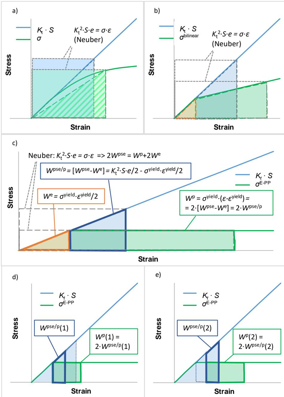
Figure 4.9: Applying Neuber’s rule to different material models: a) continuous nonlinear; b) bilinear; c) elastic-perfectly plastic (E-PP); followed by incremental application of Neuber’s rule to the E-PP material model (Figures d and e for increments 1 and 2, respectively). In the figure,  $W^{\text{e}}$  is elastic SED,  $W^{\text{p}}$  is plastic SED,  $W^{\text{pse}/\text{p}}$  is the incremental plastic portion of the pseudoelastic SED.
