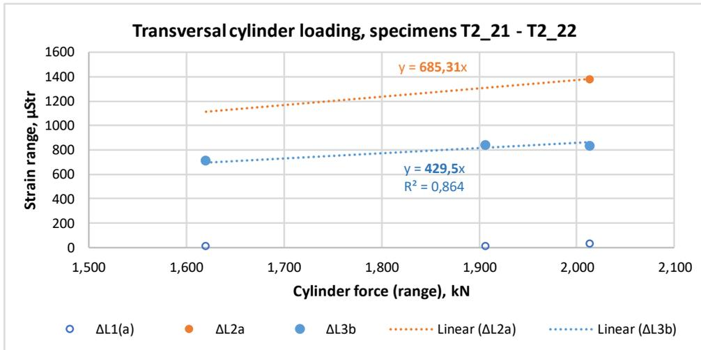
Figure B.5.3: Relation between the strain range and the range of the transversal cylinder loading for specimens T2\_21–T2\_22 (Ø42.4 x 3.3; weld a4.5).
