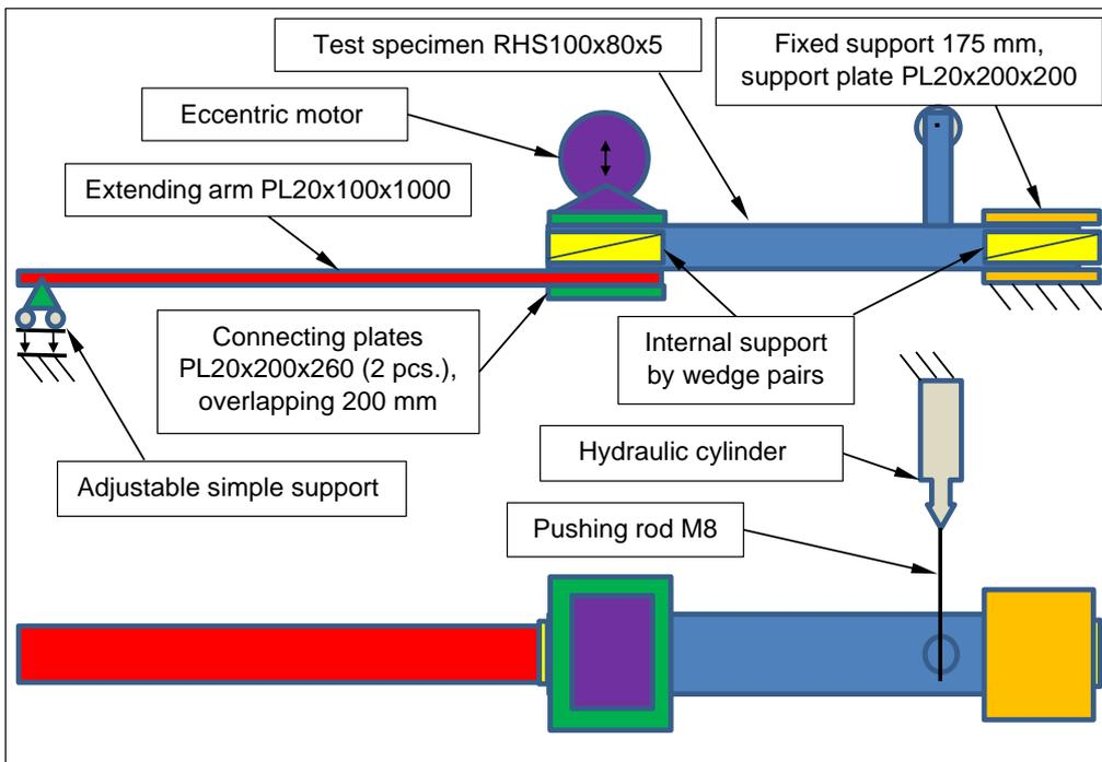
Figure B.1: The principal scheme of the test system.
