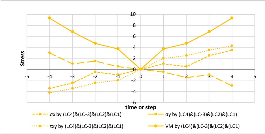
Figure 4.5: The stress history of the anti-symmetric alternating reversal formed by four independent constant amplitude loads. The example is based on the critical combination defined by the yellow curve in Figure 4.4. The continuous curve presents the amplitude-based value of the von Mises equivalent, symmetric for the left and right halves of the stress history.
