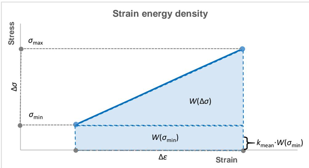
Figure C.1: Strain energy density of uniaxial loading with positive minimum stress
