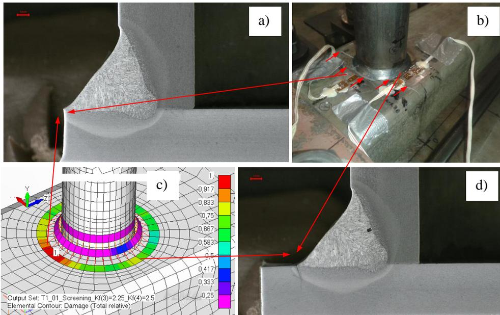
Figure 5.7: Test specimen T1\_01 (b). The weld toe failure at location RHS 0° (a, strain gauge L1), initiated the crack growth at location RHS 90° (d, strain gauge 2a) and estimated the most critical location using the developed screening method (c).
