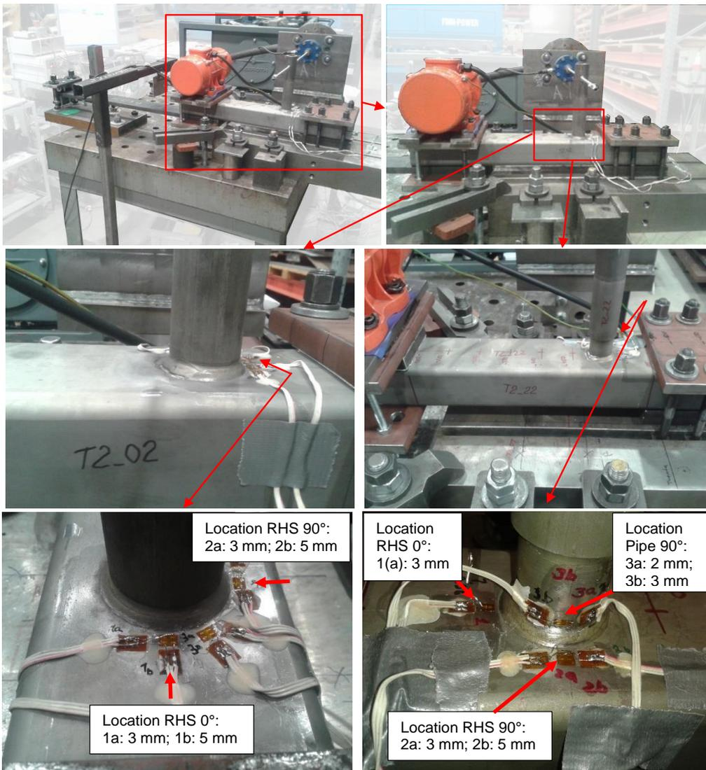
Figure B.3: Locations of the strain gauges on the test specimens T2\_02 and T2\_22.
