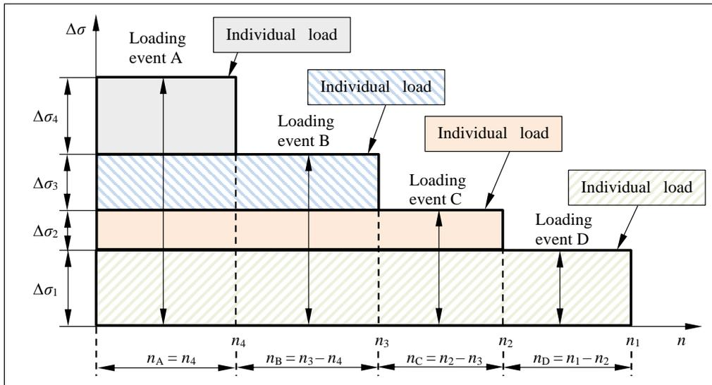
Figure 3.6: Simplified method of determining the stress ranges and number of cycles of the loading events of stress history, consisting of a set of independent individual loadings ( $n_1 > n_2 > n_3 > n_4$ ). Vertical axis  $\Delta\sigma$  is stress range and horizontal axis  $n$  is the number of loading cycles.
