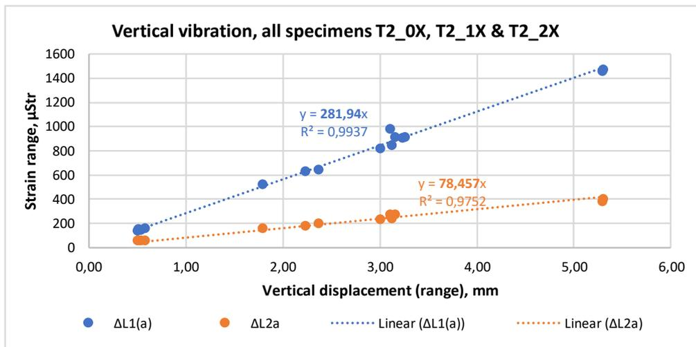
Figure B.4: Relation between the strain range and the range of the vertical displacement under vertical vibration.
