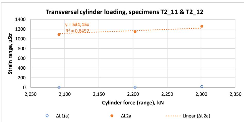
Figure B.5.2: Relation between the strain range and the range of the transversal cylinder loading for specimens T2\_11–T2\_12 (Ø42.4 x 6.3; weld a4).
