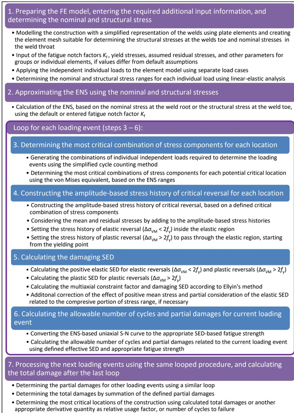
Figure 4.1: Main steps of the developed screening procedure to determine the critical locations of a welded structure, based on the strain energy density method.
