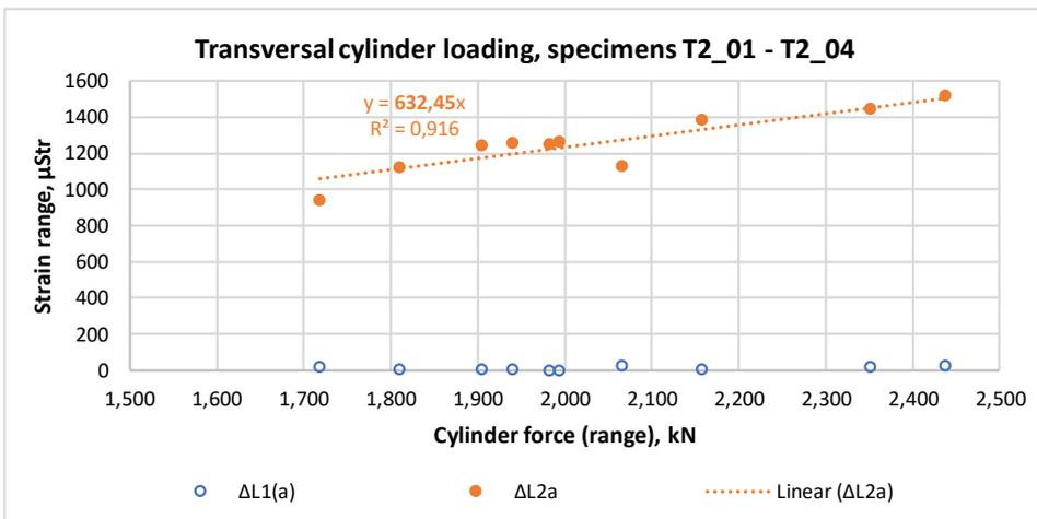
Figure B.5.1: Relation between the strain range and the range of the transversal cylinder loading for specimens T2\_01–T2\_04. Test specimens Ø42.4 x 6.3; weld size 6 mm (semi-V3 and fillet a3).
