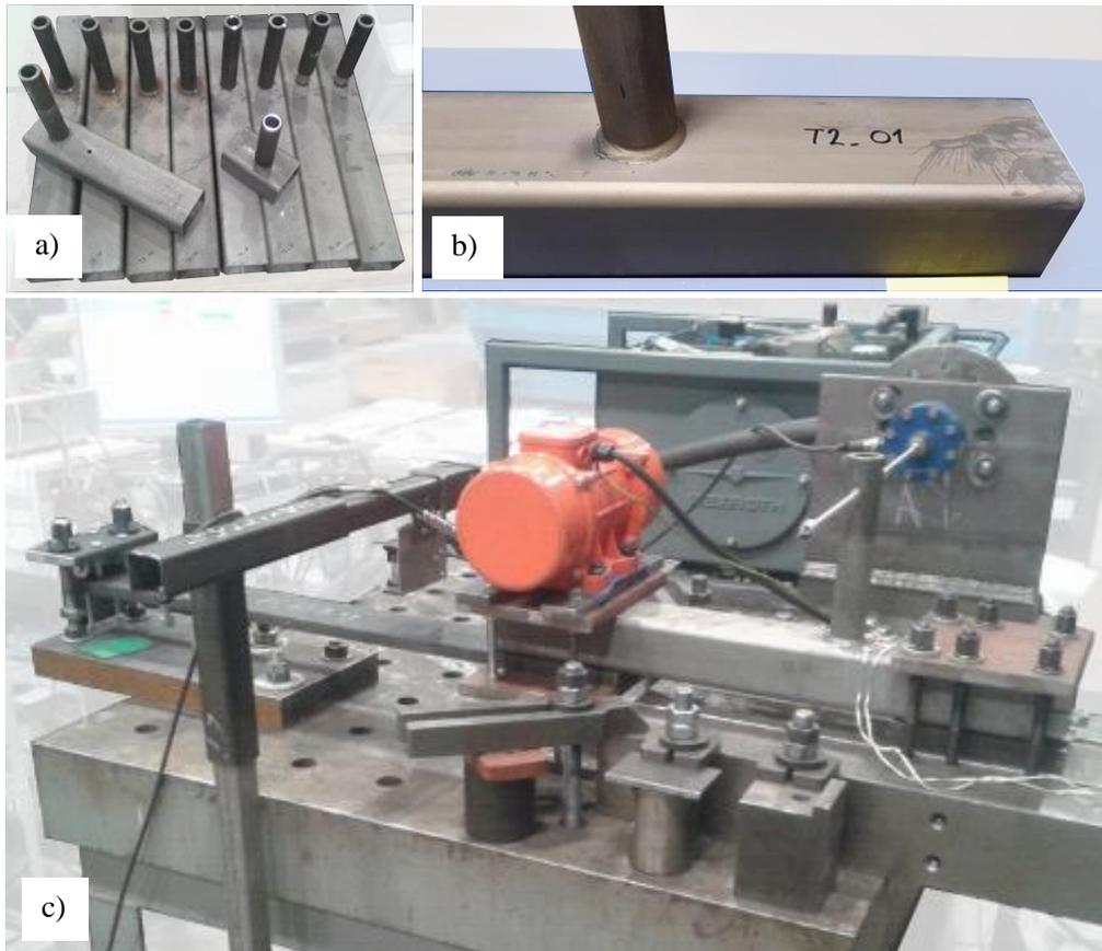
Figure 5.2: Test specimens (a, b) and test system used to verify the screening method (c).
