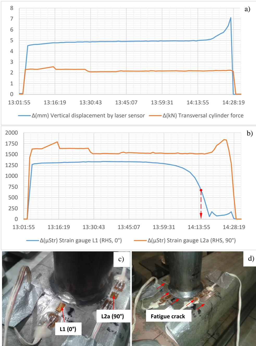
Figure 5.3: The measured loads (a) and strain ranges (b) of Specimen T1\_01 (c,d). The 50% decrease in the range, measured by strain gauge L1, is used as an indicator of failure.
