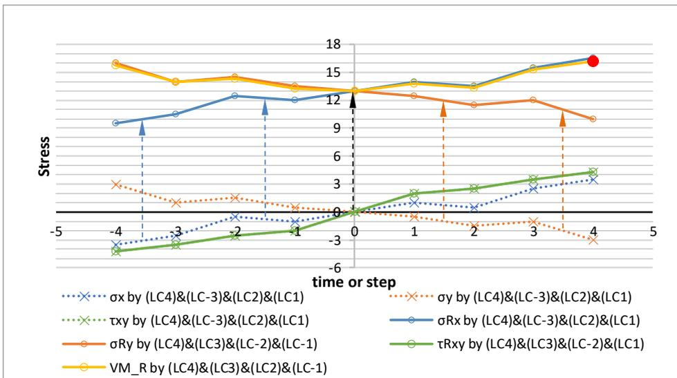
Figure 4.6: Preliminary replacement of the stress history by moving the midpoint from origo to the equi-biaxial yielding point of material. The assumed yield stress of the material and residual stress is 13 units. Index R in the component's names refers to "replaced". The example is based on the critical combination defined by the yellow curve in Figures 4.4 and 4.5.
