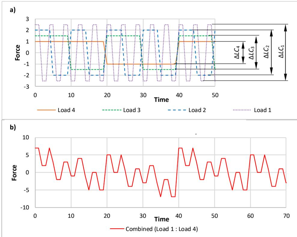
Figure 4.3: Example of the four independent constant amplitude loads (a), corresponding load ranges to generate the separate load cases and combined load history (b).
