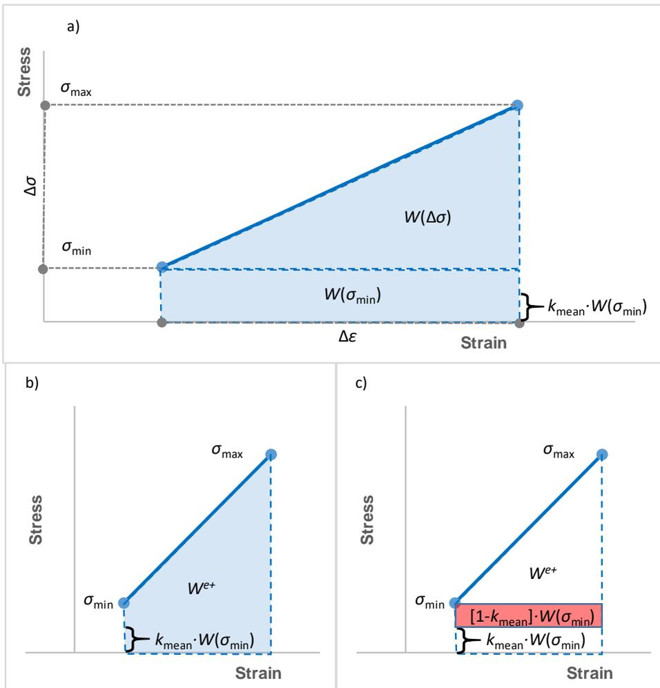
Figure 4.12: a) The strain energy density (SED)  $W^{e+}$  of a cycle with positive minimum stress  $\sigma_{min}$ ; b) correction of the mean stress effect by reduction of the SED below the stress range  $W(\sigma_{min})$  using correction factor  $k_{mean}$ ; c) the corresponding correction by subtracting the overestimated portion  $[1 - k_{mean}] \cdot W(\sigma_{min})$  from the total SED  $W^{e+}$ .
