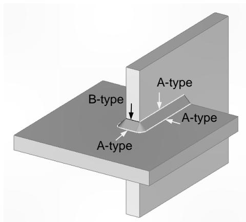
Figure 3.1: Hot spot types A and B. Type A is located on the surface of the plate. Type B is located on the edge of the plate, loaded by in-plane loading.
