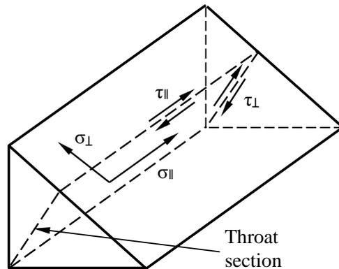
Figure 4.2: Stress components of the fillet weld.
