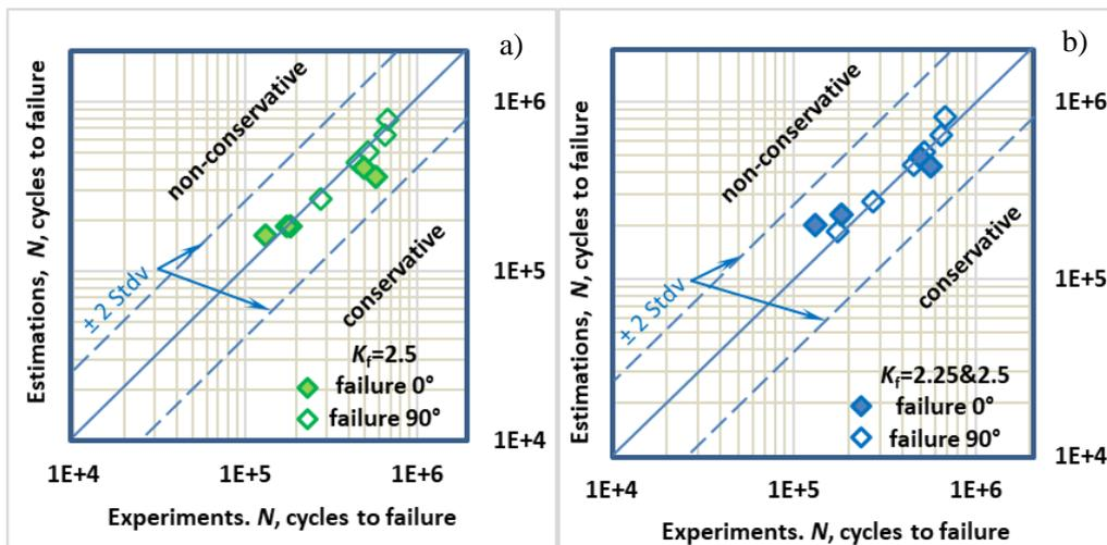
Figure 5.6: The correlation of the experimental results and the estimations defined using the fatigue notch factor  $K_f = 2.5$  (a) and using the fatigue notch factors  $K_f = 2.25$  for vibration and  $K_f = 2.5$  for cylinder loading (b). The estimations are based on  $FAT_{mean} = 308$  MPa with probability of survival  $P_s = 50\%$ .
