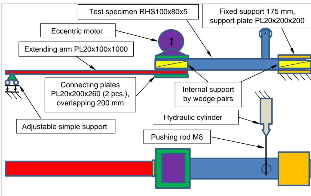
Figure 5.1: The principal scheme of the test system.
