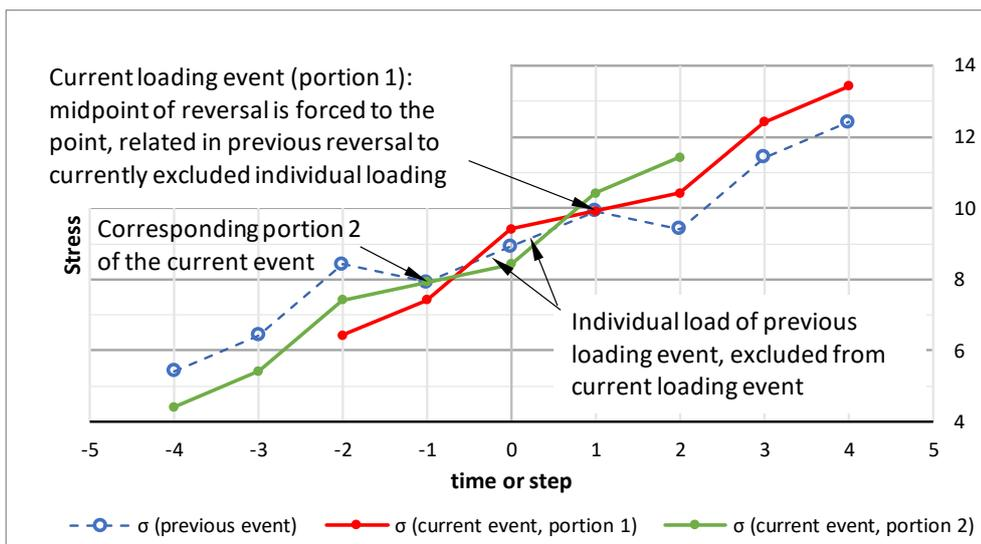
Figure 4.13: Approximation of the mean stress of second and subsequent loading events. The dotted blue line represents the reversal of the previous loading event. The number of current reversals is divided into equivalent portions with similar symmetric reversals, represented in the figure by red and green continuous lines. The midpoints of each portion of these reversals are forced to the points related in the previous reversal to the currently excluded load.
