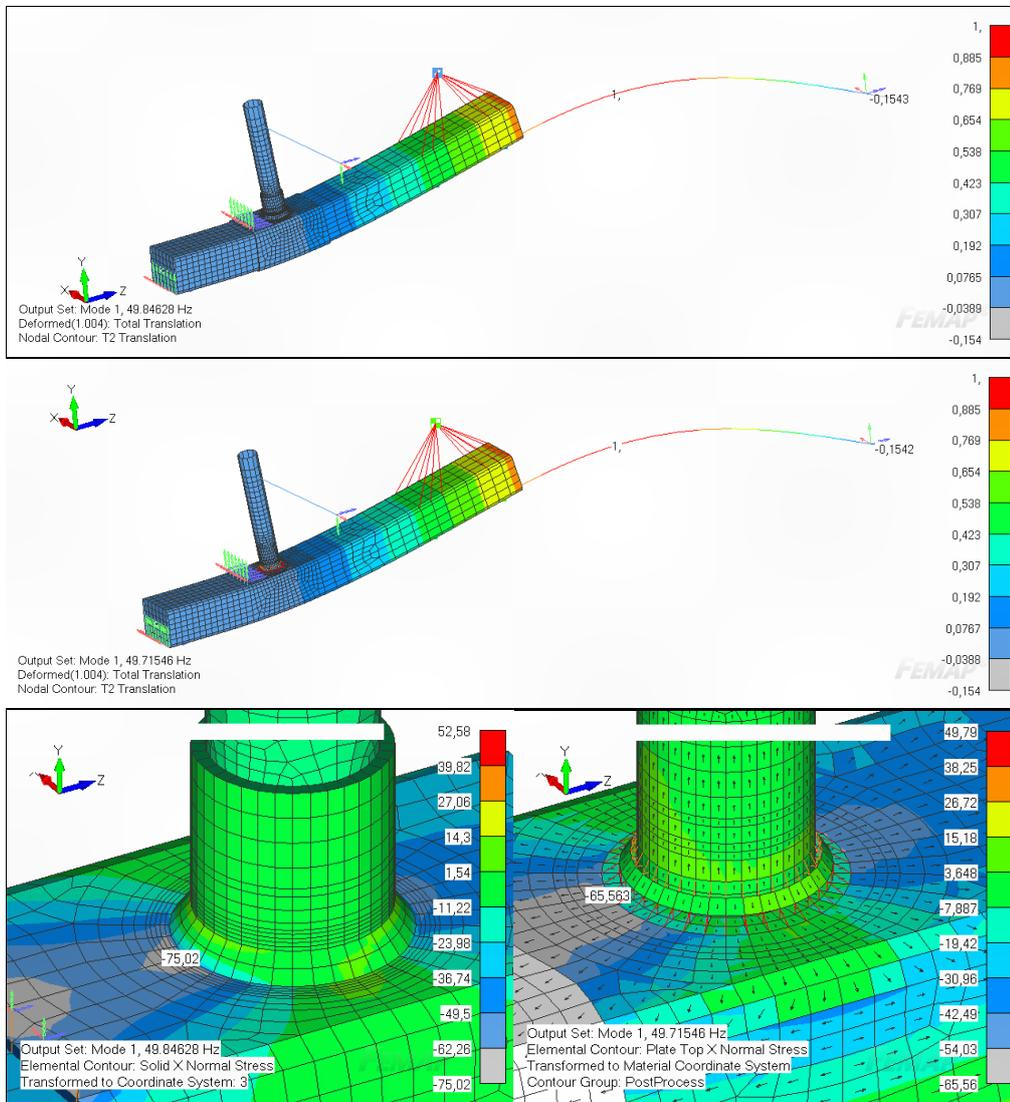
Figure B.6: FE model of test specimen T2\_0X ( $\text{Ø}42.4 \times 6.3$ ; weld size 6 mm). Deformations and normal surface stresses (MPa) perpendicular to the weld toe under vertical vibration loading with unit vertical displacement. The upper and left-hand figures present the results of the FE model with linear solid elements (mesh size 1 mm). The middle and right-hand figures present the results of the FE model with parabolic plate elements (mesh size 5 mm).
