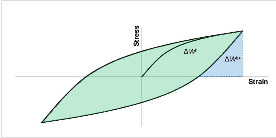
Figure 3.5: Damaging portion of the strain energy density (SED) according to Ellyin's model. The range of plastic SED is inside the hysteresis loop, and the triangle area under the right side of the hysteresis loop is the positive part of the range of elastic SED.
