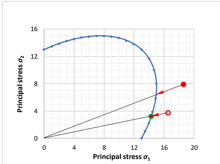
Figure 4.8: Obtaining the scale factor to fit the elastic stress history to the elastic area. The assumed yield stress of the material is  $f_y = 13$  units.
