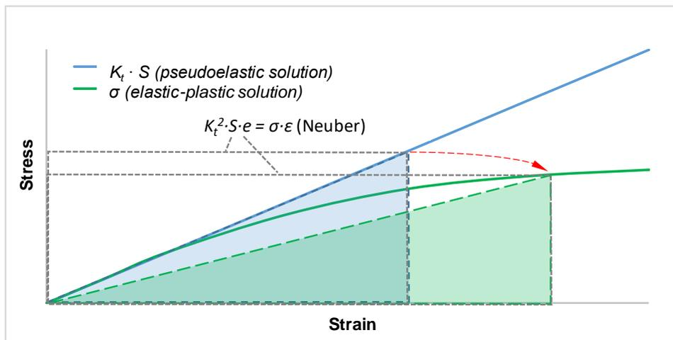
Figure 3.3: Graphical presentation of Neuber's rule. The shaded triangles with equivalent areas present the left- and right-hand sides of Equation 3.15, divided by 2.
