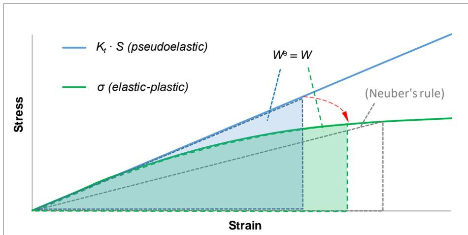
Figure 3.4: Graphical presentation of Glinka's equivalent strain energy density (ESED) method. The shaded equivalent areas represent elastic and elastic-plastic strain energy densities. The unshaded area of the triangle represents Neuber's rule for comparison.
