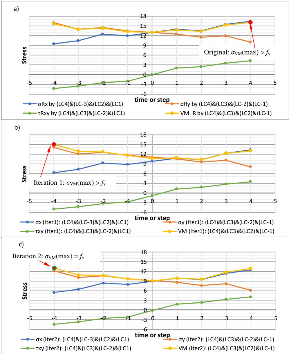
Figure 4.7: Fitting the elastic stress history to the elastic area in two iterations: a) Original history of reversal, replaced from origo to yielding point; b) History of reversal after first fitting iteration; c) History of reversal after second fitting iteration. The assumed yield stress of material is  $f_y = 13$  units.
