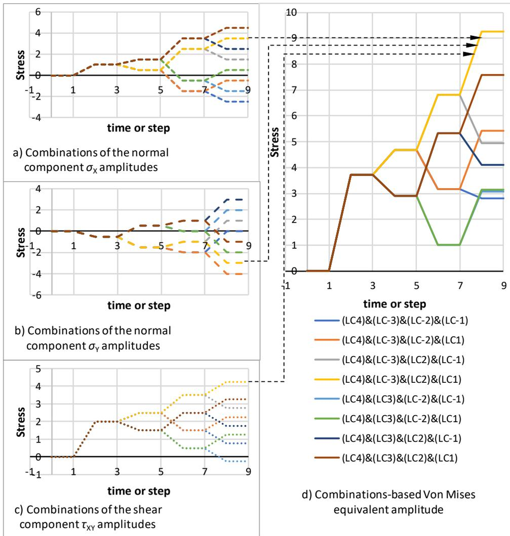
Figure 4.4: Example of the cycle formed by four independent constant amplitude loads. The possible combinations of the stress component are presented on the left-hand side of the figure (a–c). The right-hand side of the figure presents the corresponding von Mises equivalent amplitude (d). The yellow curve represents the determinative combination of the stress amplitudes in this example.
