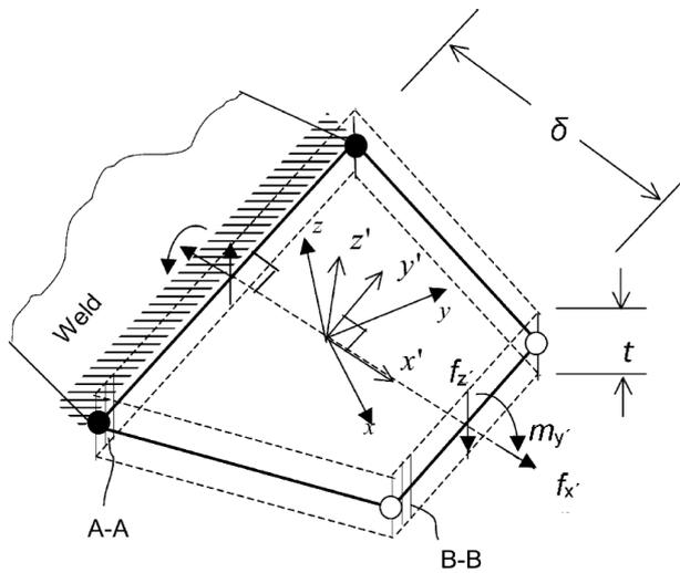
Figure 3.2: Determining structural stress by stress resultants (Dong, 2001, slightly modified).
