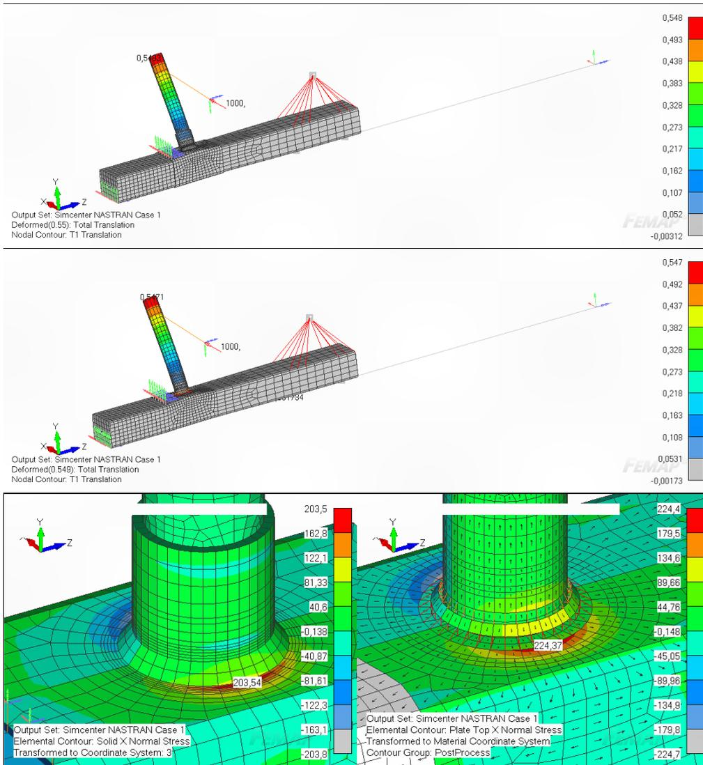
Figure B.7: FE model of test specimen T2\_0X ( $\varnothing 42.4 \times 6.3$ ; weld size 6 mm). Deformations and normal surface stresses (MPa) perpendicular to the weld toe under transversal cylinder loading 1000 N. The upper and left-hand figures present the results of the FE model with linear solid elements (mesh size 1 mm). The middle and right-hand figures present the results of the FE model with parabolic plate elements (mesh size 5 mm).
