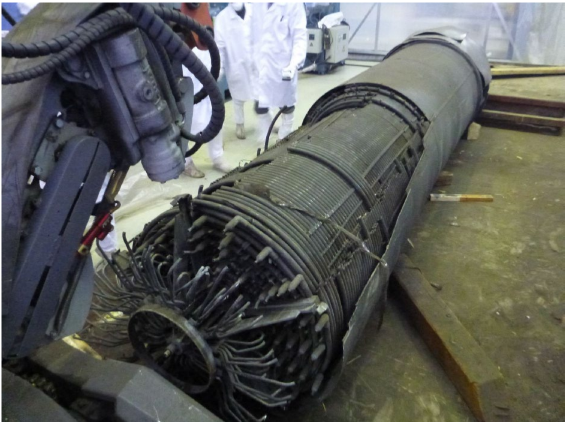
Figure 3.3. PG-28 (after 140,000 hours of operating in 25 years) [14].
