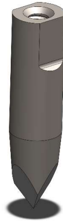
Figure 12. Hole piercing tool head. From top down: mounting thread, wrench faces, hole rounding taper and cutting edges joining in the piercing tip
