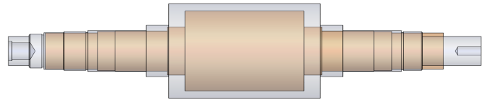
Fig. 5. Cross section of case study rotor (grey) and rotor geometry using baseline dimensions (orange)
