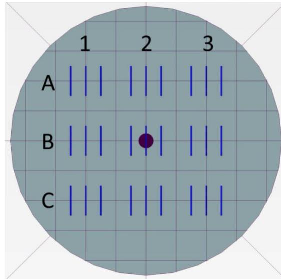
**Figure 25.** A single filament line test matrix including varying printing speeds (1,2,3) versus varying layer heights (A,B,C) (Allevi 2020).
