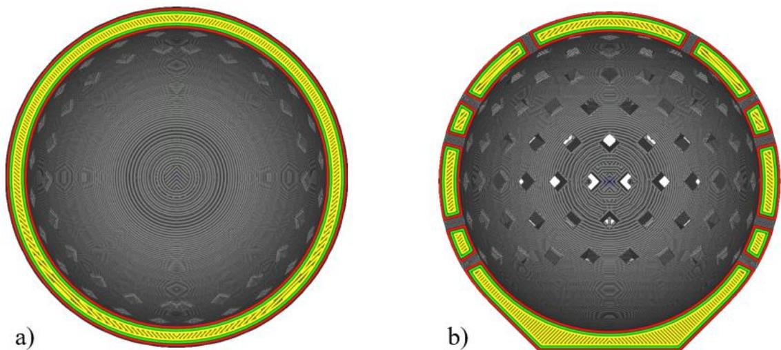
**Figure 30.** The effect of build orientation on filament construction.
