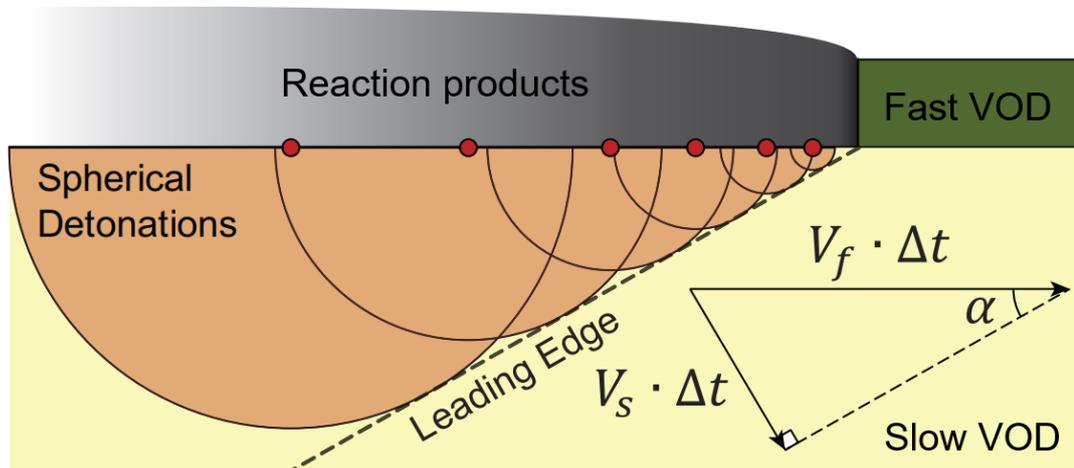
**Figure 18.** Formation of a tilted shock wave (Modified from Loiseau J. et al. 2014 p.2).
