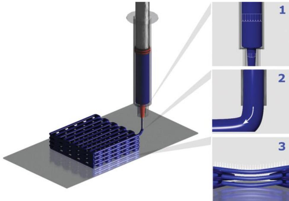
**Figure 20.** DIW deposition process (Modified from Tagliaferri et al. 2021 p.542).
