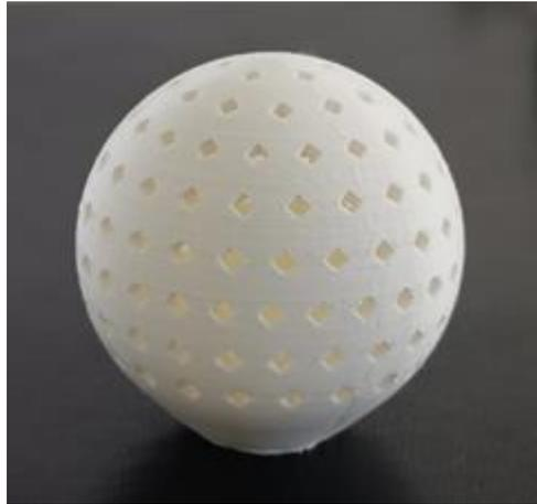
**Figure 31.** Printed prototype part designed according to the best practises of DfAM
