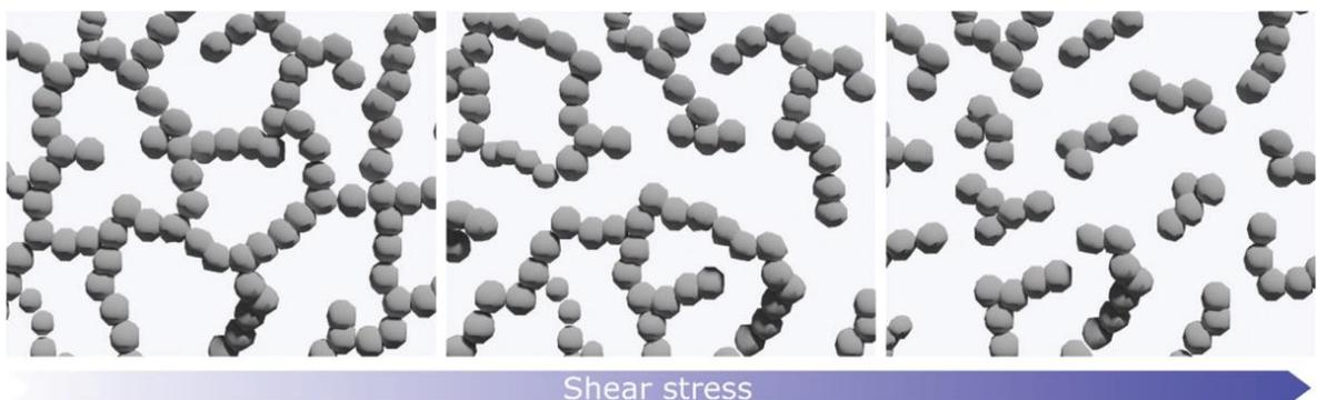
**Figure 22.** Shear thinning behaviour of a material under shear stress (Tagliaferri et al. 2021 p. 544).
