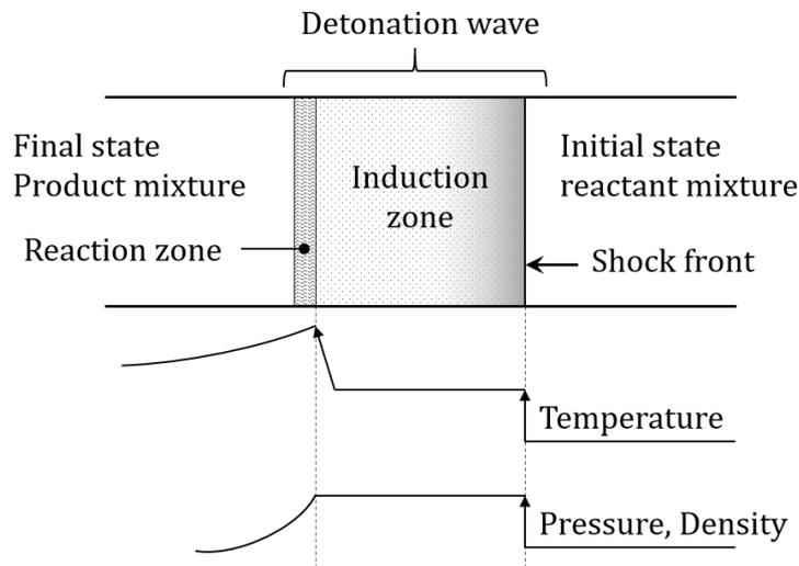
**Figure 14.** A ZND detonation model diagram showing the pressure, temperature and density profiles of the propagating shock wave.
