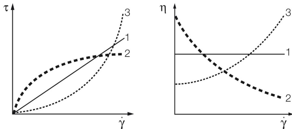
**Figure 21.** Flow curves (left) and viscosity curves (right) for (1) ideally viscous, (2) shear-thinning, and (3) shear-thickening flow behaviour.
