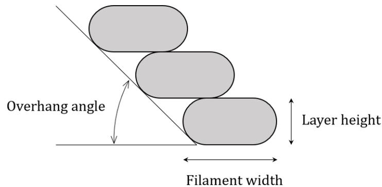
**Figure 28.** Definition of overhang angle
