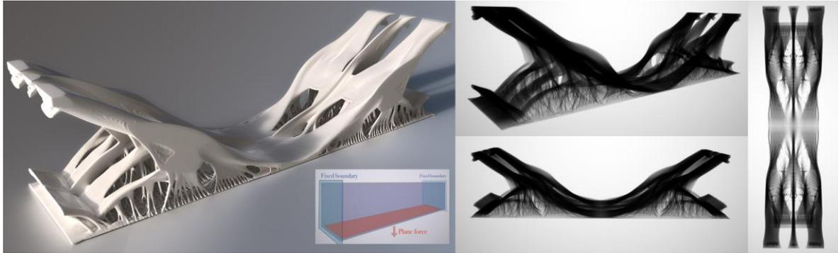
**Figure 6.** High-resolution, Narrow-Band Topology Optimized bridge structure (Liu et al. 2019 p.4).
