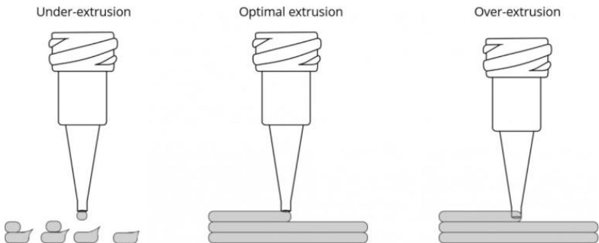
**Figure 24.** The effect of extrusion rate on filament formation (Allevi 2020).
