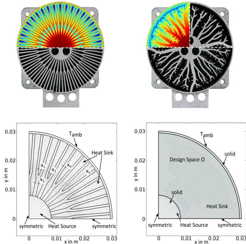
**Figure 8.** Comparison of parametric and topology optimization (Modified from Lange et al. 2018) .
