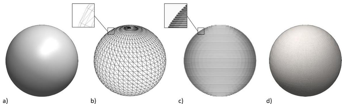
**Figure 26.** Additive manufacturing steps showing a) 3D geometry description, b) STL standard data interface, c) slicing and tool path design, and d) final part.
