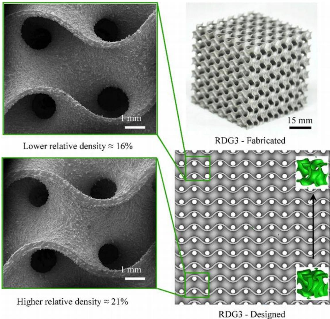
**Figure 11.** AM manufactured lattices with relative density grading TPMS unit cell (Al-Ketan et al. 2019b, p. 7).
