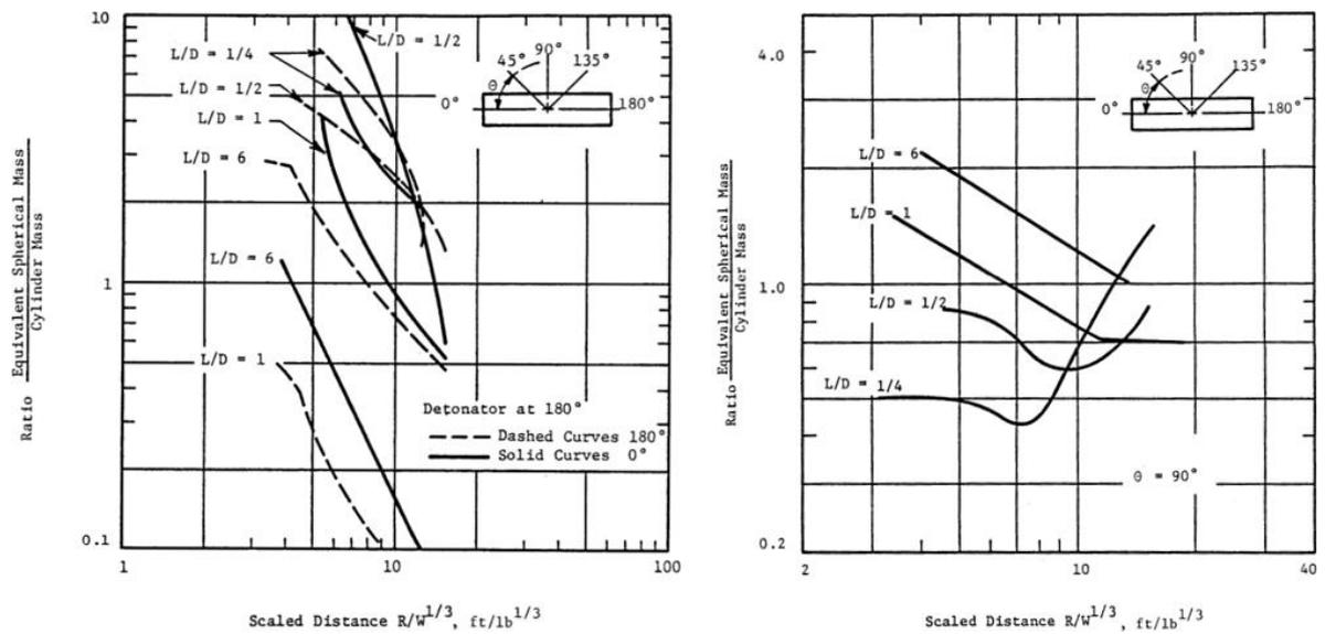
**Figure 17.** Empirical relationships for cylinders with various  $L/D$  ratios at  $\theta = 0^\circ$  and  $90^\circ$  (Modified from United States Department of Energy. 1980, p. 4-62...63).
