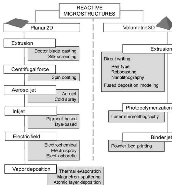
**Figure 19.** Additive manufacturing methods for reactive microstructure fabrication (Muravyev et al. 2019 p.942).
