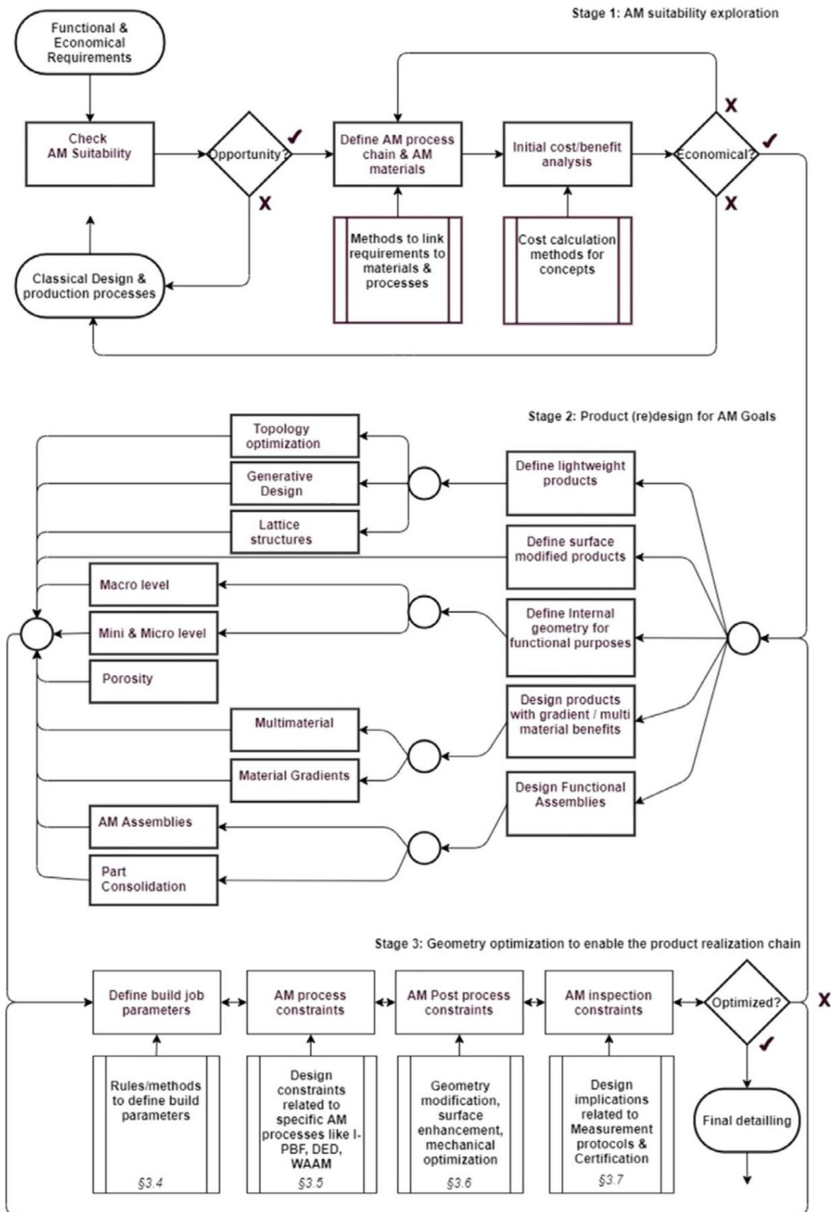
**Figure 4.** Design framework linking DfAM stages, actions and goals (Vaneker et al. 2020, p. 581).
