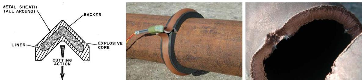
**Figure 16.** Munroe cutting effect (Modified from Scopex 2021 and Smith J. 1984).
