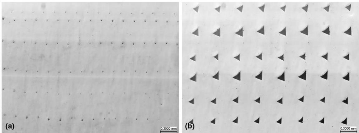
Figure 32. Mesostructure voids with (a) 0.2 mm and (b) 0.4 mm layer thickness. (Rankouhi B. et al. 2016 p.477)
