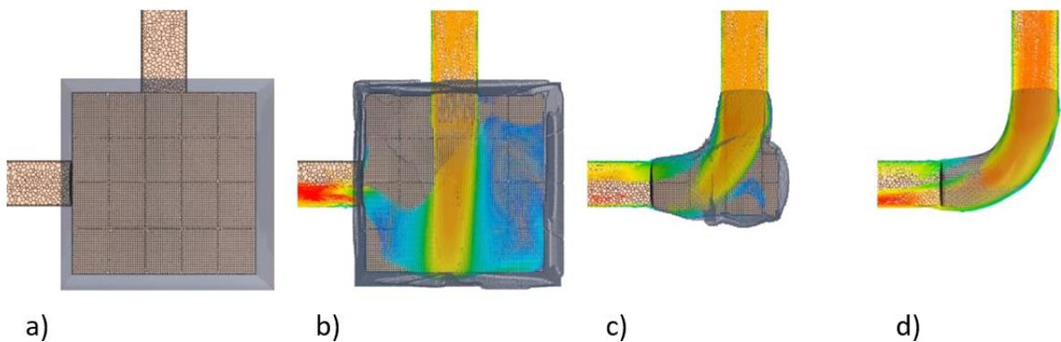
**Figure 7.** CFD driven topology optimization process (Modified from Siemens 2021).
