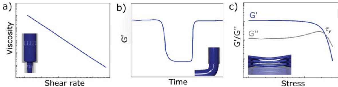
**Figure 23.** The rheological response of a printable material (Modified from Tagliaferri et al. 2021 p.545).
