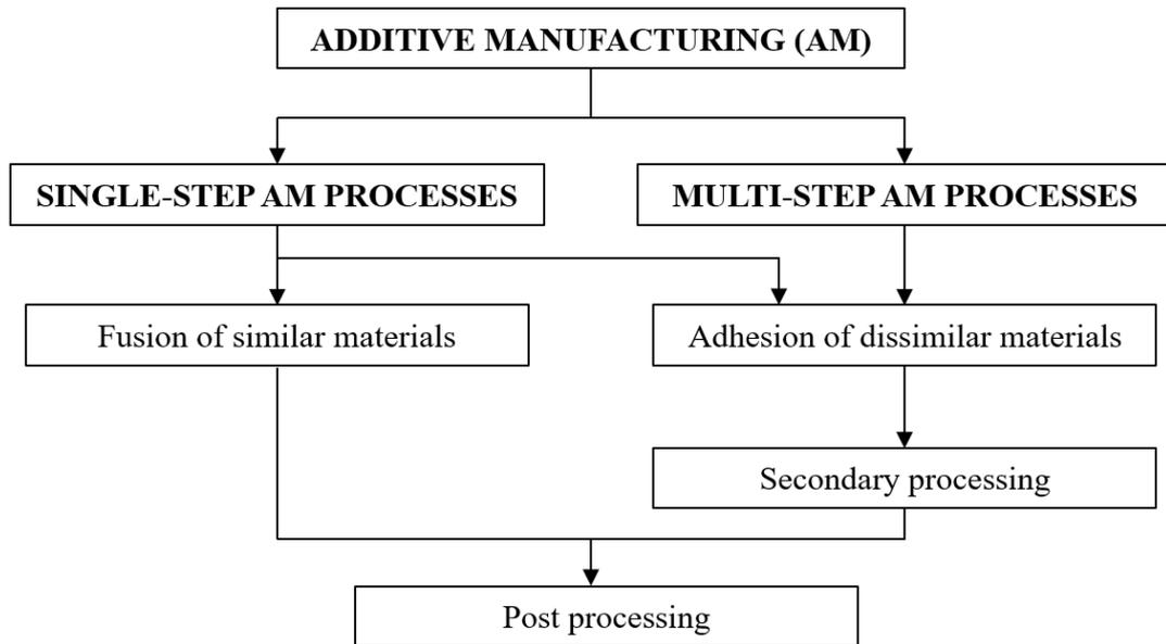
**Figure 1.** Single-step and multi-step AM processes.
