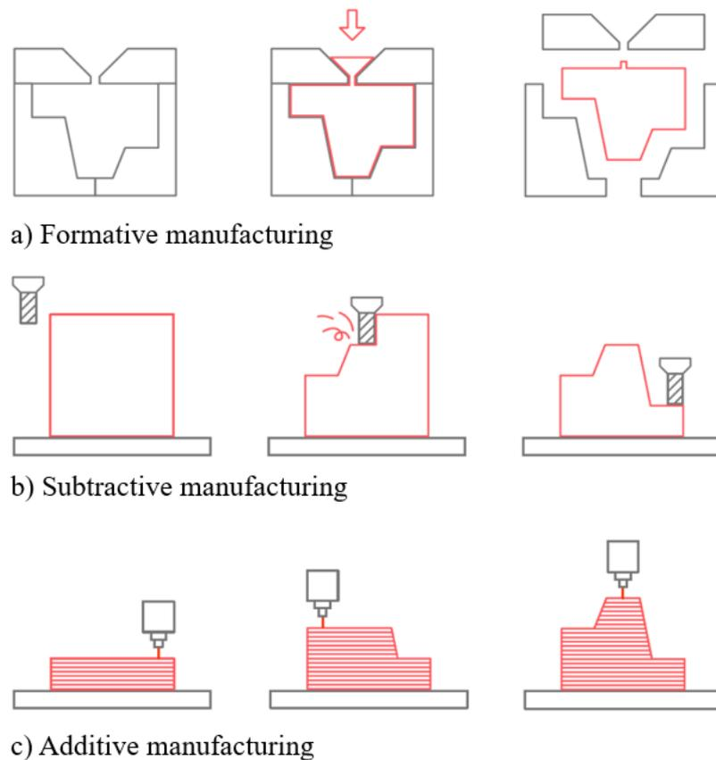
**Figure 2.** Subtractive manufacturing method (Modified from 3D HUBS. 2021a).
