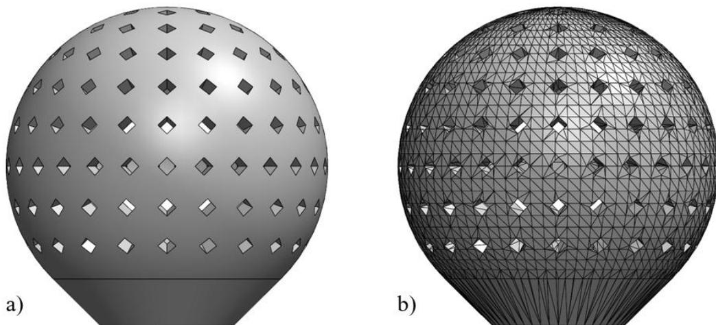
Figure 29. The effect of STL geometry approximation on 3D geometry.
