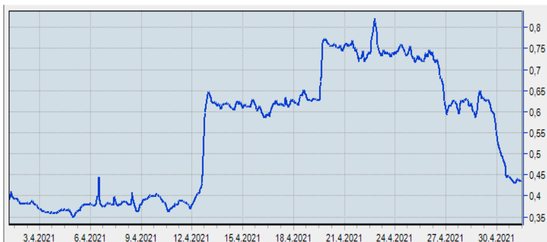
Figure 19. Specific conductivity, mS/m, of boiler water during the sodium tracer trial period in Metsä Fibre Äänekoski, measured with mill online analyzer
