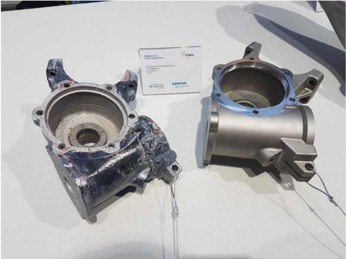
Figure 8. A reproduction of an original Roston Hornsby A1 model 1920 car gear box by Siemens. In comparison the original worn out part shown on the left had been machined from a solid metal block.
