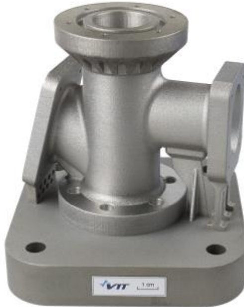
Figure 3. L-PBF print with integrated support structure and platform (Kokkonen et al. 2016).
