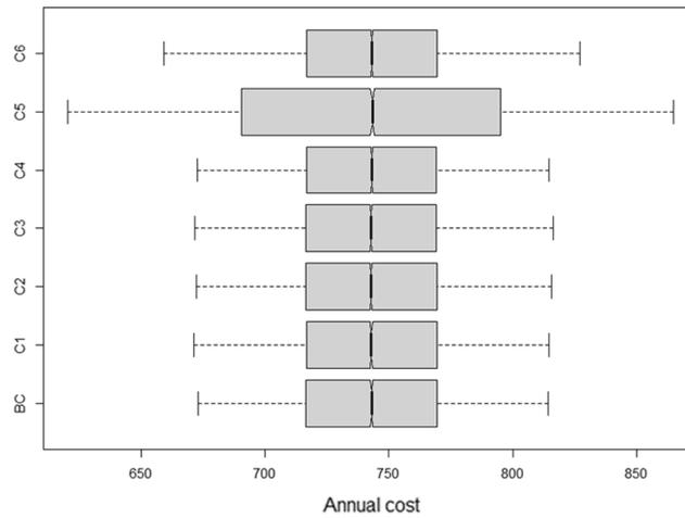
**Fig. B3.** Boxplot of the annual costs of implementing thickened tailings technology and water supply of 50% of water quality 1 and 50% of water quality 2. BC represents the base case, C1 CAPEX<sub>d</sub> ± 20%, C2 OPEX<sub>d</sub> ± 20%, C3 CAPEX<sub>w</sub> filtered seawater ± 20%, C4 OPEX<sub>w</sub> filtered seawater ± 20%, C5 COST<sub>T</sub> ± 20%, and C6 COST<sub>RO</sub> ± 20%.
