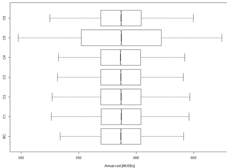
**Fig. 2.** Boxplot of the annual costs of implementing filtered tailings technology and water supply of 50% of higher quality water and 50% of lower quality water. BC represents the base case, C1 CAPEX<sub>d</sub> ± 20%, C2 OPEX<sub>d</sub> ± 20%, C3 CAPEX<sub>w</sub> filtered seawater ± 20%, C4 OPEX<sub>w</sub> filtered seawater ± 20%, C5 COST<sub>T</sub> ± 20%, and C6 COST<sub>RO</sub> ± 20%.
