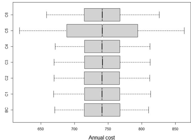
**Fig. B1.** Boxplot of the annual costs of implementing conventional tailing disposal technology and water supply of 50% of water quality 1 and 50% of water quality 2. BC represents the base case, C1 CAPEX<sub>d</sub> ± 20%, C2 OPEX<sub>d</sub> ± 20%, C3 CAPEX<sub>w</sub> filtered seawater ± 20%, C4 OPEX<sub>w</sub> filtered seawater ± 20%, C5 COST<sub>T</sub> ± 20%, and C6 COST<sub>RO</sub> ± 20%.
