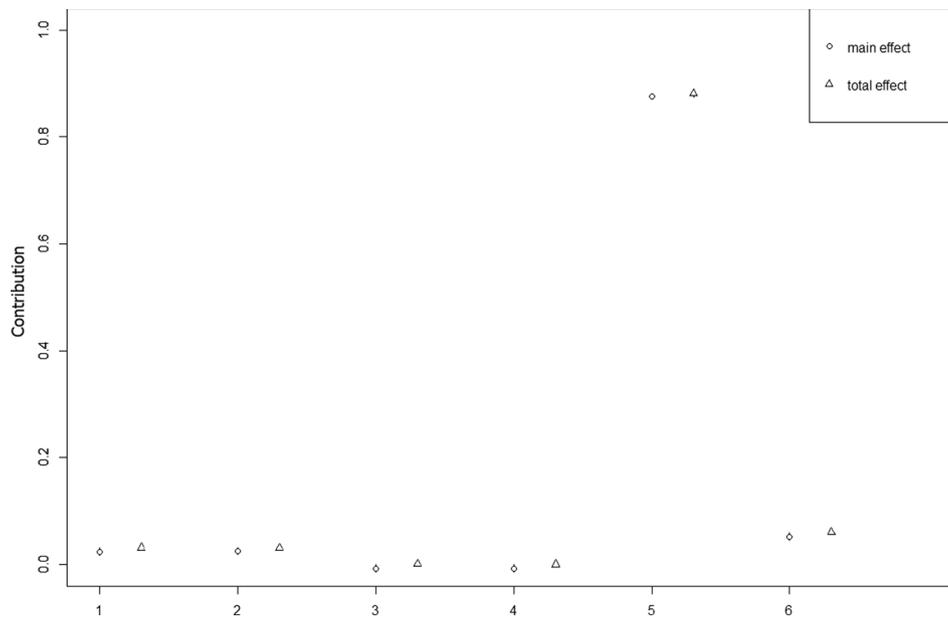
**Fig. 3.** Sobol' indices of the annual costs of implementing filtered tailings and water supply of 50% of higher quality water and 50% of lower quality water. Where 1 CAPEX<sub>d</sub>, 2 OPEX<sub>d</sub>, 3 CAPEX<sub>w</sub> filtered seawater, 4 OPEX<sub>w</sub> filtered seawater, 5 COST<sub>T</sub>, and 6 COST<sub>RO</sub>.
