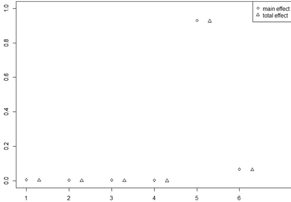
**Fig. B2.** Sobol' indices of the annual costs of implementing conventional tailing disposal and water supply of 50% of water quality 1 and 50% of water quality 2. Where 1 CAPEX<sub>d</sub>, 2 OPEX<sub>d</sub>, 3 CAPEX<sub>w</sub> filtered seawater, 4 OPEX<sub>w</sub> filtered seawater, 5 COST<sub>T</sub>, and 6 COST<sub>RO</sub>.
