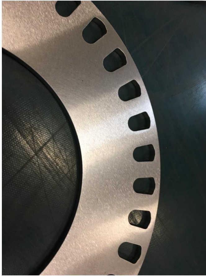
Figure 14. Deburred and ground lamination disk.
