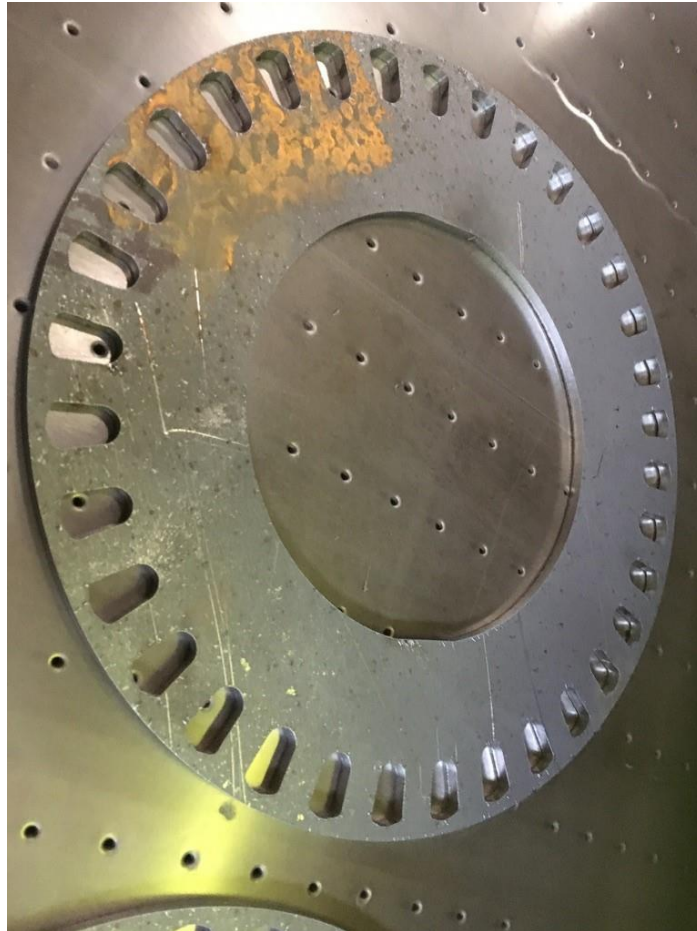
Figure 13. Hardox 400 disk after first round of grinding.
