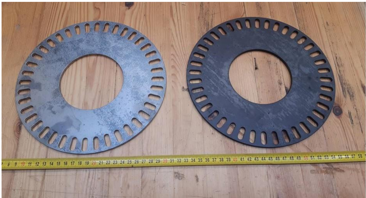
Figure 16. Lamination disks with and without black oxide coating.
