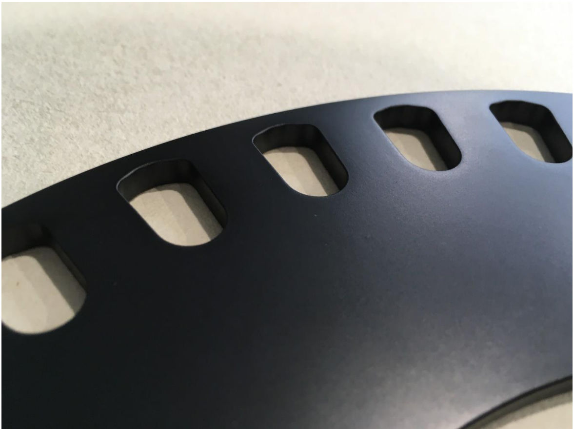
Figure 17. PTFE coated lamination disk.
