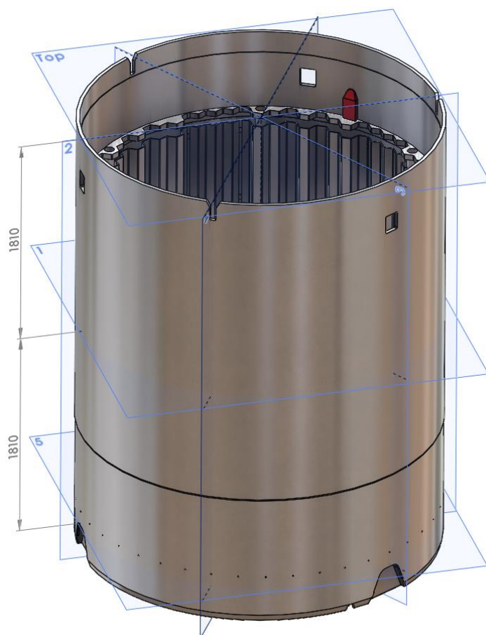
Figure 8. Segmentation scheme of core basket, where three vertical and two horizontal cuts are made.
