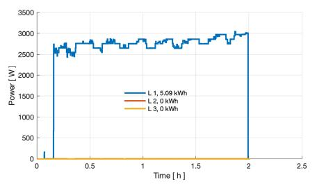
Figure 19: Power curve of three phases at -20  $^{\circ}$ C ambient temperature in the Nissan preheating test.
