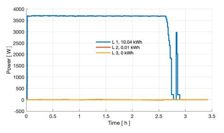
Figure 42: Power curve of three phases at -10 °C ambient temperature in the Volvo charging test.
