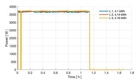
Figure 24: Power curve of three phases at 0 °C ambient temperature in the Volkswagen charging test.
