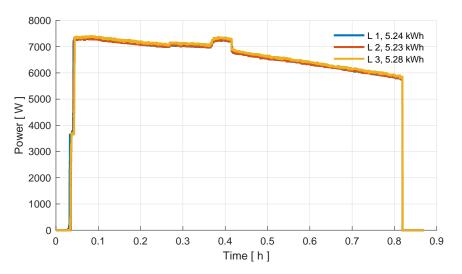
Figure 6: Power curve of three phases at 20 °C ambient temperature in the Tesla charging test.
