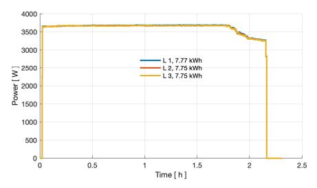
Figure 37: Power curve of three phases at -20 °C ambient temperature after overnight parking at the 70% SoC in the Kia charging test.
