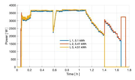
Figure 29: Power curve of three phases at -20 °C ambient temperature after overnight parking at the 60% SoC in the Volkswagen charging test.
