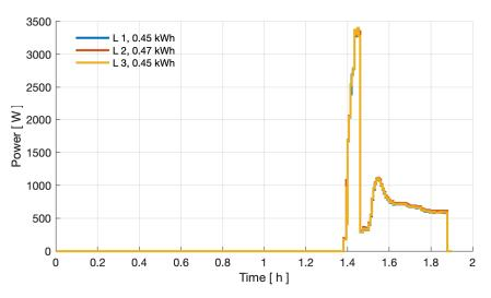
Figure 31: Power curve of three phases at 0 °C ambient temperature in the Kia preheating test.
