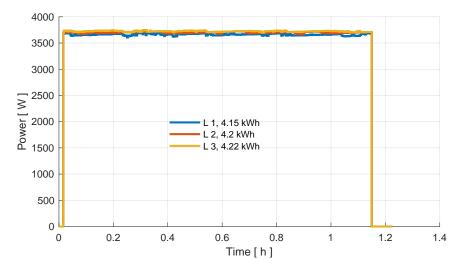
Figure 28: Power curve of three phases at -20 °C ambient temperature in the Volkswagen charging test.
