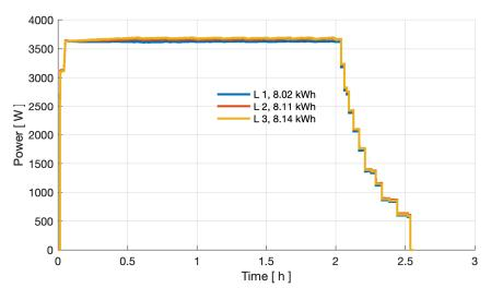
Figure 36: Power curve of three phases at -20 °C ambient temperature in the Kia charging test.
