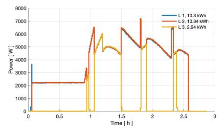
Figure 13: Power curve of three phases at -20  $^{\circ}$ C ambient temperature after overnight parking at the 70% SoC in the Tesla charging test.
