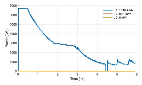
Figure 21: Power curve of three phases at -20 °C ambient temperature after overnight parking at the 70% SoC in the Nissan charging test.
