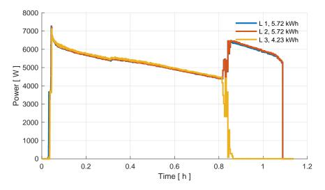
Figure 10: Power curve of three phases at -10 °C ambient temperature in the Tesla charging test.
