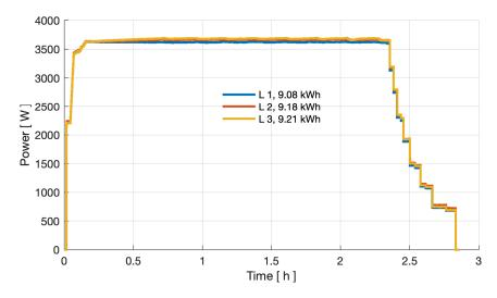
Figure 32: Power curve of three phases at 0 °C ambient temperature in the Kia charging test.
