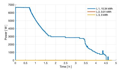
Figure 20: Power curve of three phases at -20 °C ambient temperature in the Nissan charging test.
