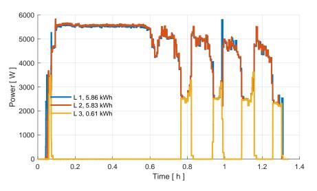
Figure 11: Power curve of three phases at -20  $^{\circ}$ C ambient temperature in the Tesla preheating test.
