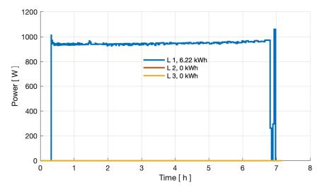
Figure 45: Power curve of three phases at -20 °C ambient temperature after overnight parking at the 0% SoC in the Volvo charging test.
