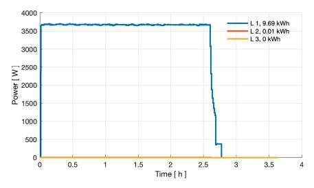
Figure 44: Power curve of three phases at -20 °C ambient temperature in the Volvo charging test.
