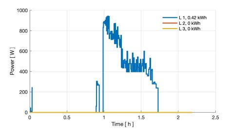
Figure 43: Power curve of three phases at -20 °C ambient temperature in the Volvo preheating test.
