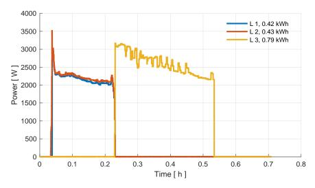
Figure 23: Power curve of three phases at 0  $^{\circ}$ C ambient temperature in the Volkswagen preheating test.
