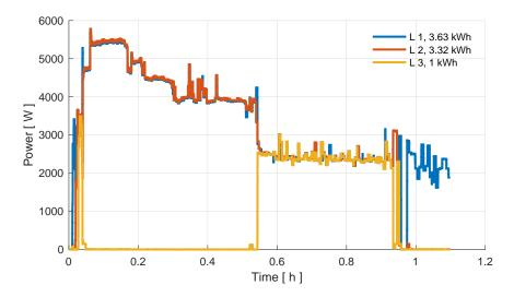
Figure 9: Power curve of three phases at -10 °C ambient temperature in the Tesla preheating test.
