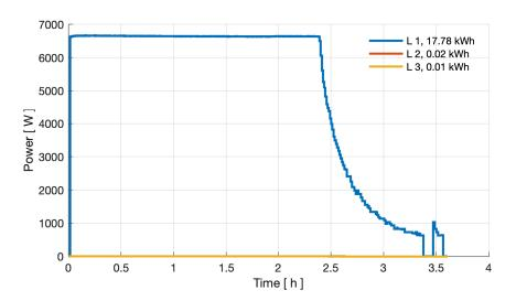
Figure 16: Power curve of three phases at 0 °C ambient temperature in the Nissan charging test.
