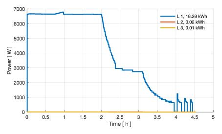
Figure 18: Power curve of three phases at -10 °C ambient temperature in the Nissan charging test.
