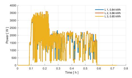
Figure 35: Power curve of three phases at -20 °C ambient temperature in the Kia preheating test.
