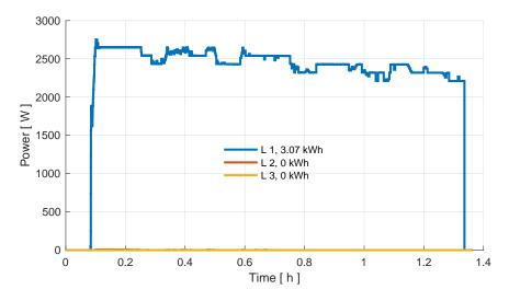
Figure 17: Power curve of three phases at -10  $^{\circ}$ C ambient temperature in the Nissan preheating test.
