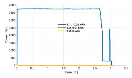
Figure 38: Power curve of three phases at 20 °C ambient temperature in the Volvo charging test.
