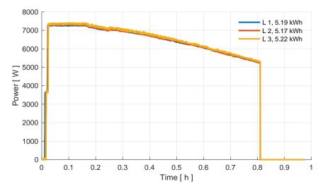
Figure 8: Power curve of three phases in 0 °C ambient temperature in the Tesla charging test.
