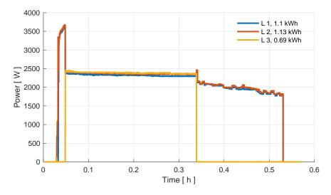
Figure 25: Power curve of three phases at -10 °C ambient temperature in the Volkswagen preheating test.
