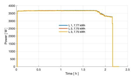
Figure 30: Power curve of three phases at 20 °C ambient temperature in the Kia charging test.
