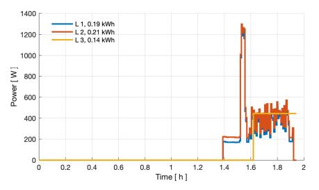
Figure 33: Power curve of three phases at -10 °C ambient temperature in the Kia preheating test.
