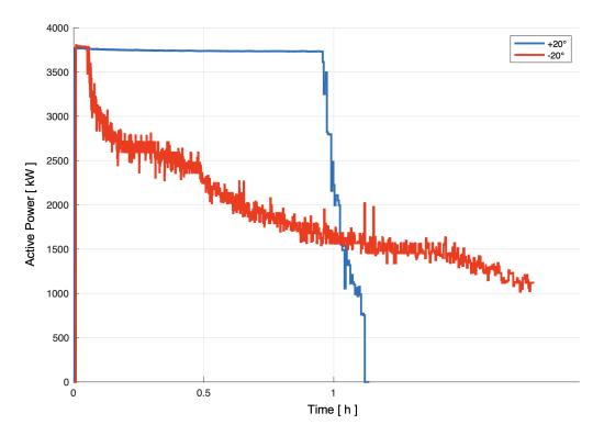
Figure 2: Example of the EV charging curve in the ambient temperature of 20  $^{\circ}$ C and -20  $^{\circ}$ C. Both example curves show the shape of the power curve when the battery SoC is approaching 100%.
