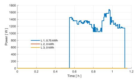
Figure 15: Power curve of three phases at 0  $^{\circ}$ C ambient temperature in the Nissan preheating test.
