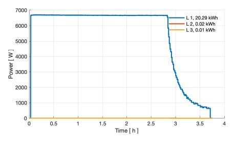
Figure 14: Power curve of three phases at 20 °C ambient temperature in the Nissan charging test.
