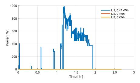
Figure 41: Power curve of three phases in -10  $^{\circ}$ C ambient temperature in the Volvo preheating test.
