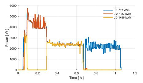
Figure 7: Power curve of three phases at 0 °C ambient temperature in the Tesla preheating test.
