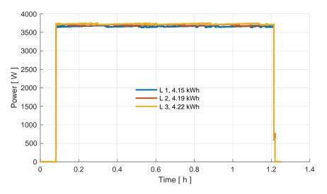
Figure 26: Power curve of three phases at -10  $^{\circ}$ C ambient temperature in the Volkswagen charging test.
