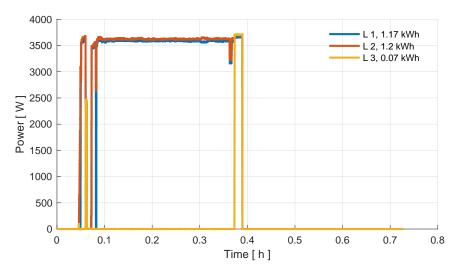
Figure 27: Power curve of three phases at -20 °C ambient temperature in the Volkswagen preheating test.
