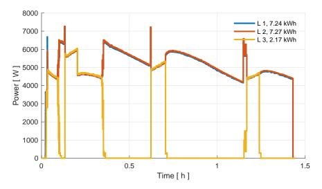
Figure 12: Power curve of three phases at -20 °C ambient temperature in the Tesla charging test.
