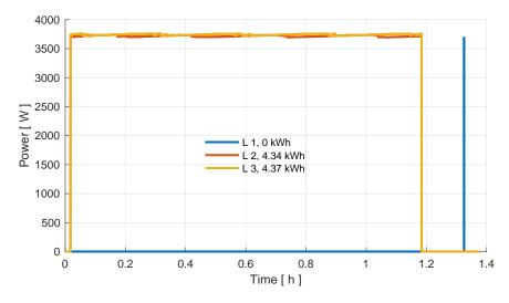
Figure 22: Power curve of three phases at 20 °C ambient temperature in the Volkswagen charging test.
