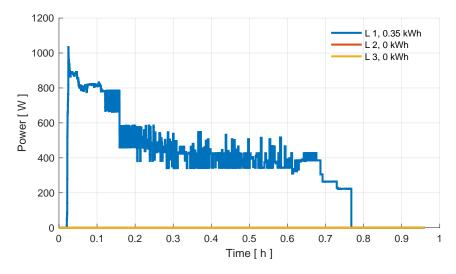
Figure 39: Power curve of three phases at -0 °C ambient temperature in the Volvo preheating test.
