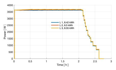
Figure 34: Power curve of three phases at -10 °C ambient temperature in the Kia charging test.
