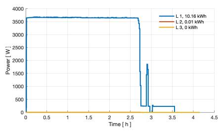
Figure 40: Power curve of three phases at -0 °C ambient temperature in the Volvo charging test.
