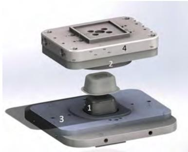
**Fig. 2** Press-forming tool set: (1) the male mould, (2) the female mould, (3) the rim tool and (4) the heating unit
