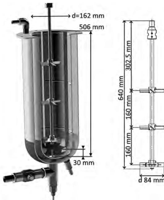
Figure 4.2: Reactor III. The reactor was equipped with a cooling or heating jacket. The stirring element was attached to a motor (Elma Troyan 1.5 kW, 2.0 hp) for powerful stirring. The reactor was designed for 10 L batches but a slightly smaller batch size was used as stirring and the presence of the gaseous phase required additional space.
