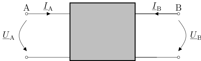
Figure 2.1 Exemplary schematics depiction of a quadropol
