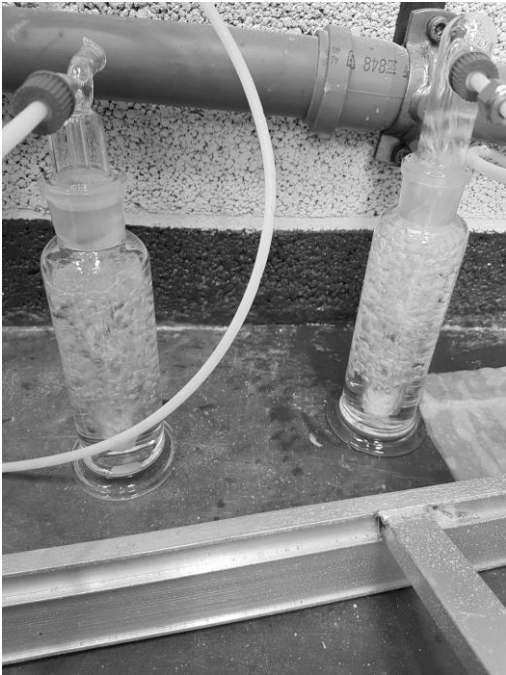
Figure 13 Gas impingers used in time lag measurements for DO
