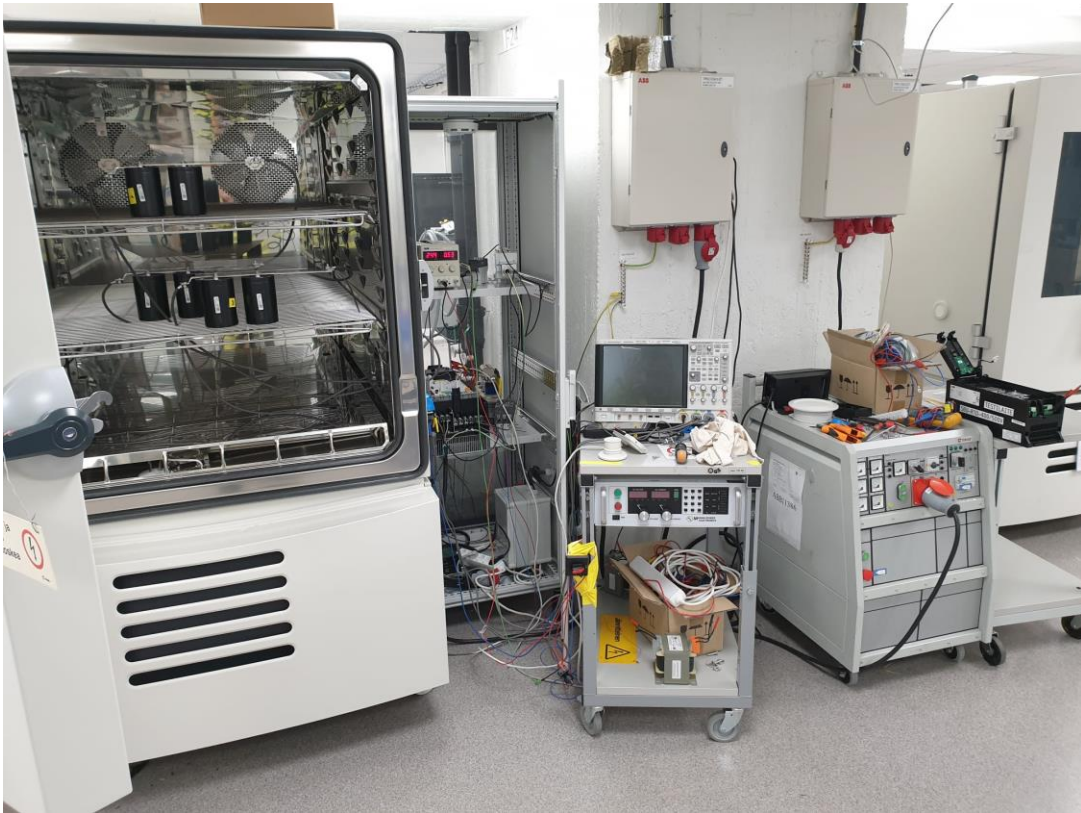
Figure 7. Picture of the whole test setup. Environmental chamber with the capacitors. Cabinet with the VSD, power resistor and contactors. On the table DC-power supply and an oscilloscope and on the far right a variable AC power source.
