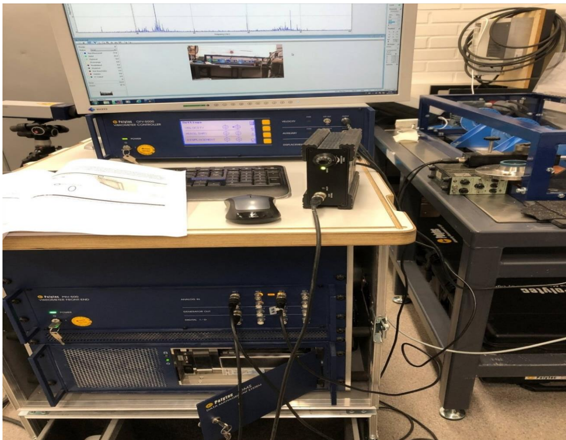
Figure 9. The measurement set-up showing the scanning laser Doppler vibrometer.
