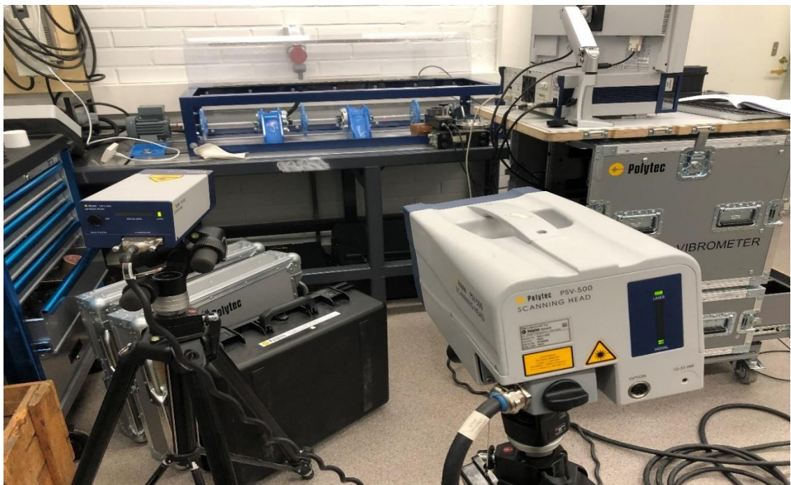
Figure 15. The scanning head of SLDV taking the measurements.
