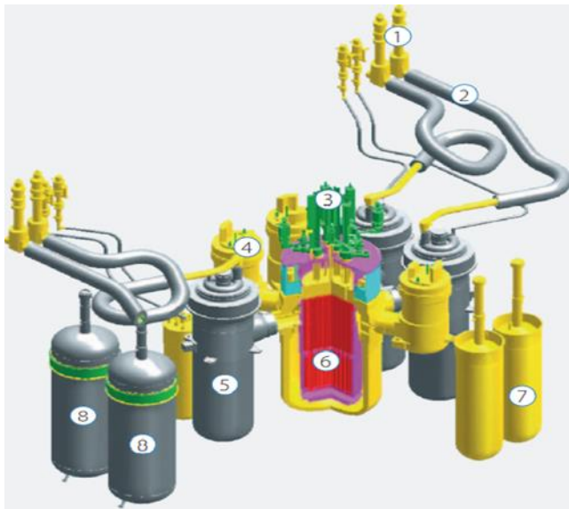
Figure 38. KLT-40S: 1) isolation valves, 2) steam lines, 3) CRDS, 4) primary coolant pump, 5) steam generator (SG), 6) reactor, 7) pressurizer, 8) hydro accumulator (JSC OKBM 2021, 15).
