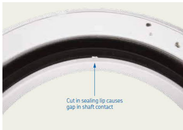
Figure 46. Cut seal surface (SKF 2019, p. 50).
